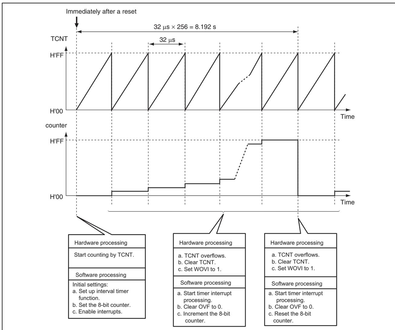
Figure 2 Operation of 8-Bit Counter Incrementation Using Interval Timer Function
