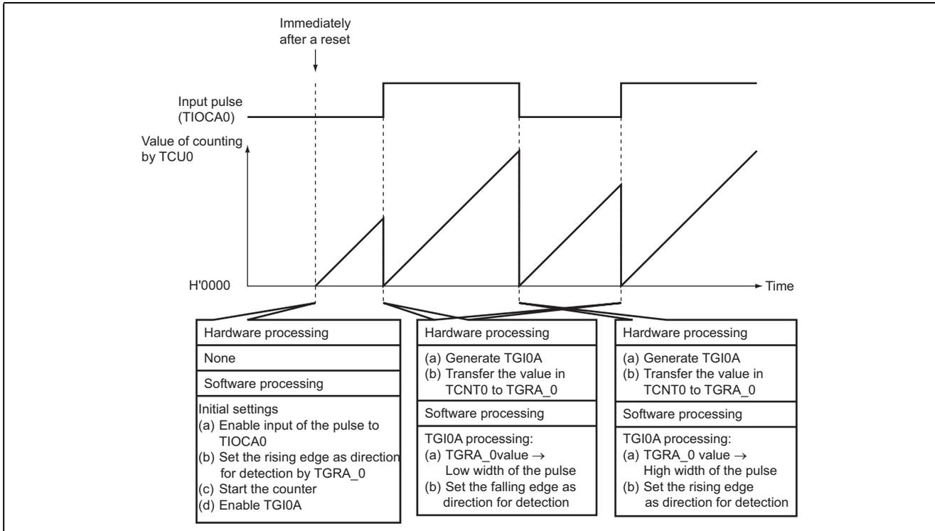
Figure 3 Measuring the Pulse Width
