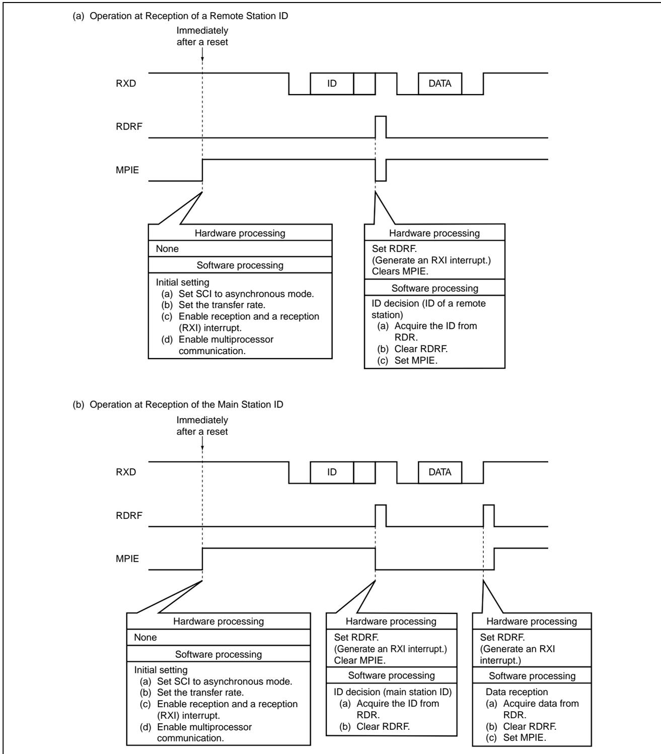
**Figure 5 Principles of Operations Used of Multiprocessor Communication (Receiving Station)**
