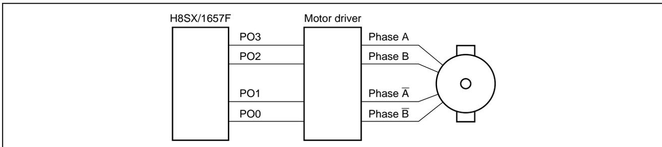
**Figure 1 Connections for Two-Phase Stepping Motor Control**
