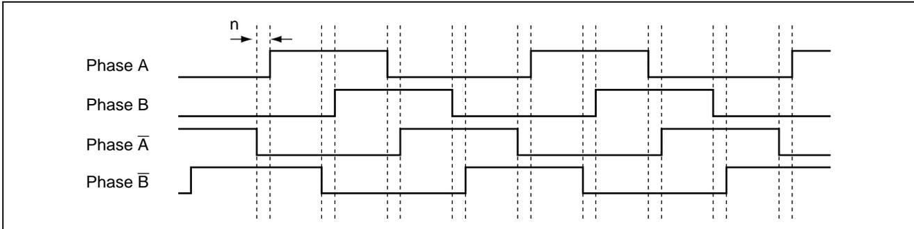
Figure 5 Example of Output with Non-Overlap Time
