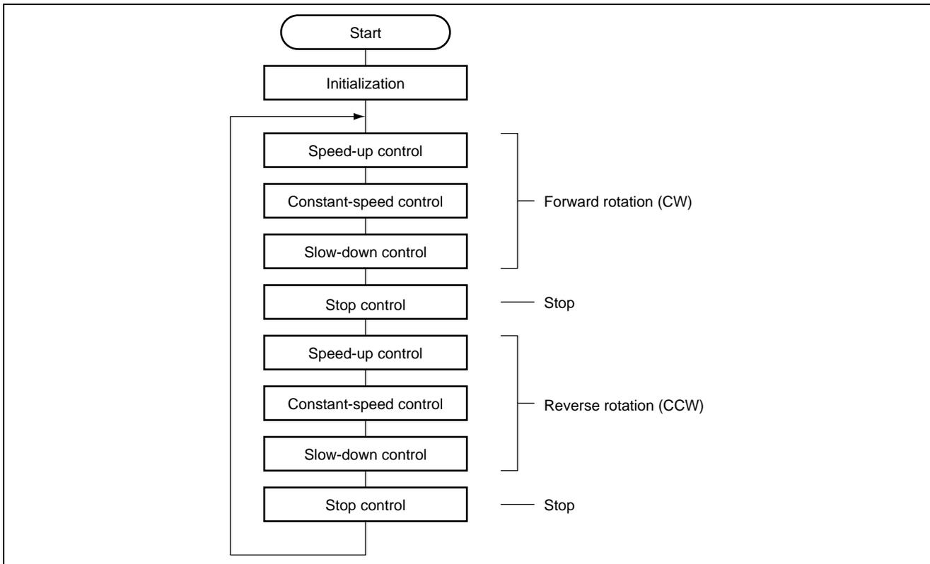
Figure 7 Flowchart of Stepping Motor Control
