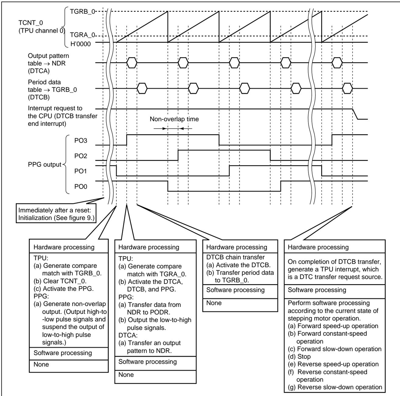
Figure 8 Timing of Stepping Motor Operation
