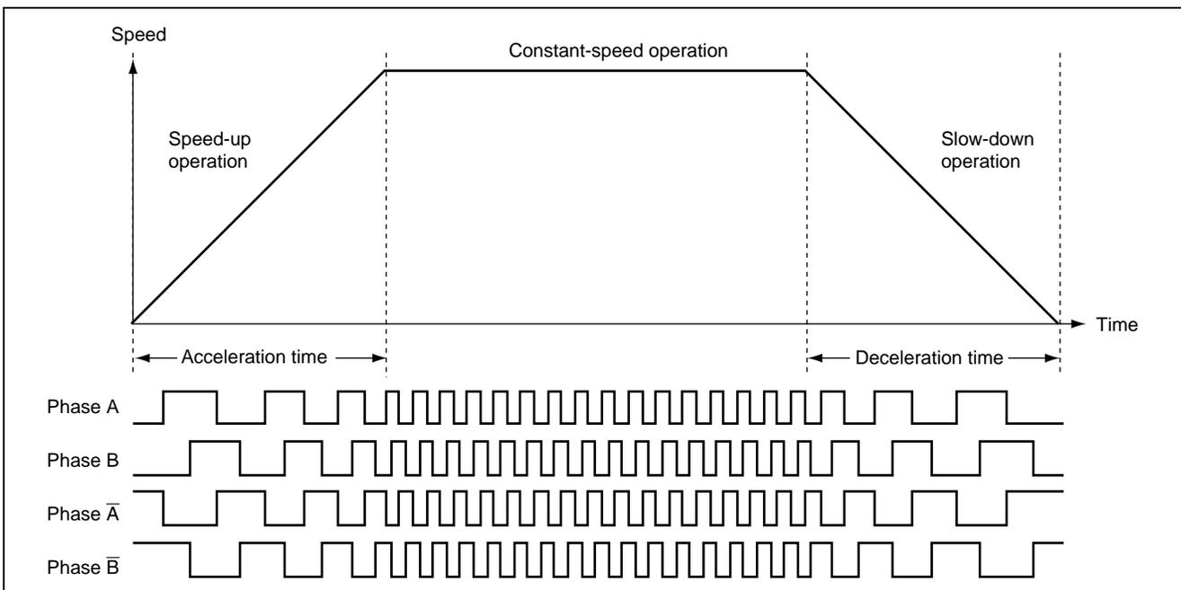
Figure 6 Speed-Up and Slow-Down Operation
