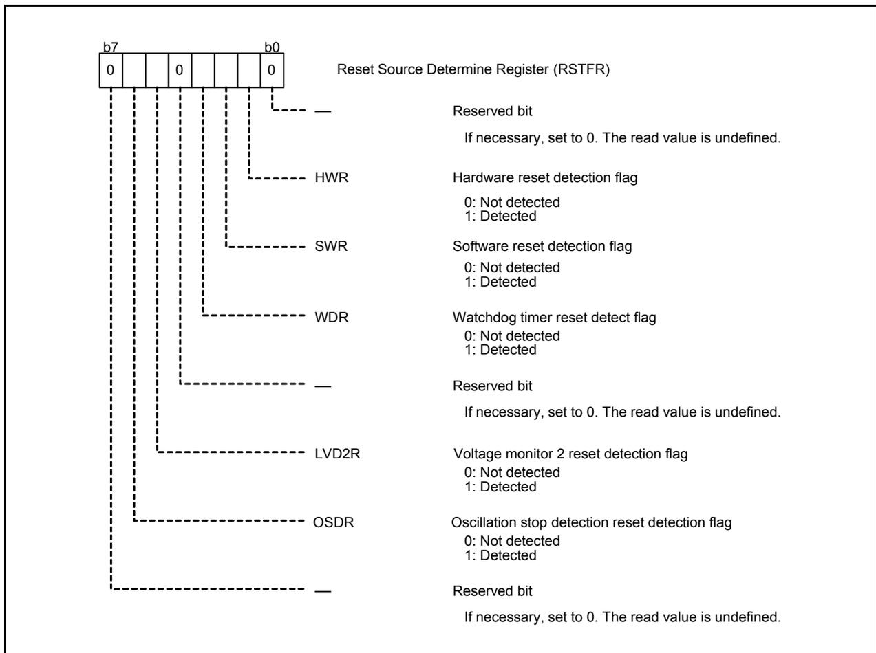
**Figure 3.1 Reset Source Determine Register**
