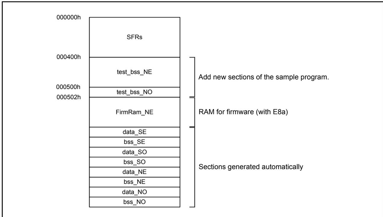
Figure 4.1 Application Example of Section Assignment
