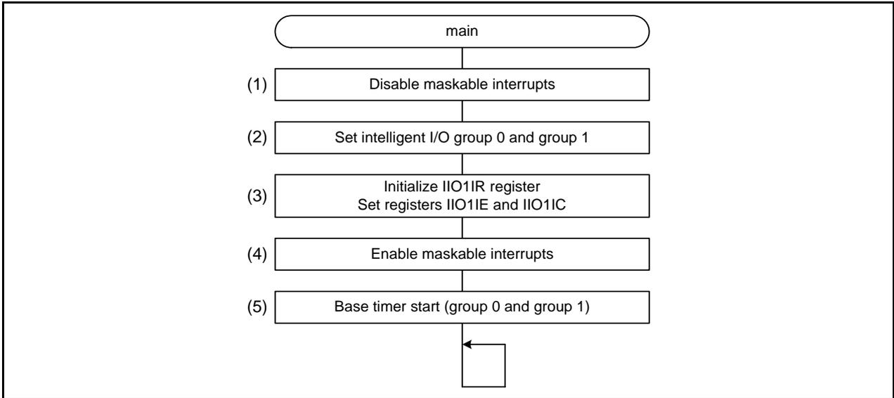
Figure 4.3 main Function Flowchart
