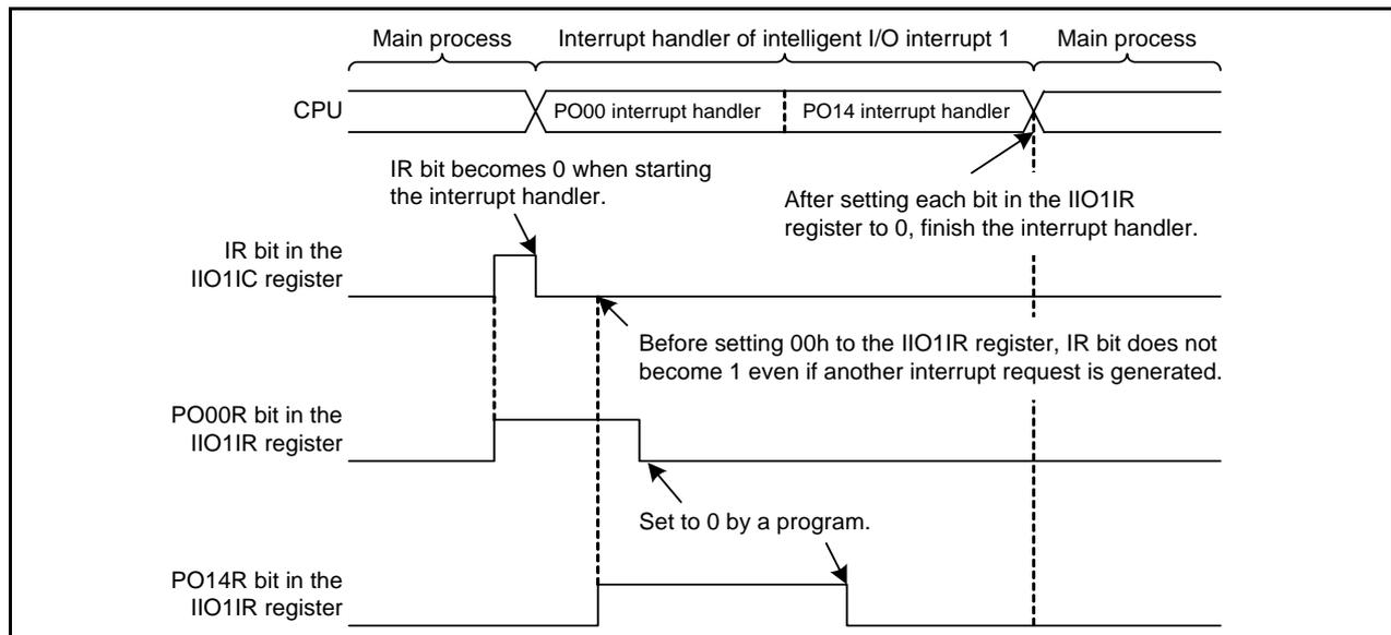
**Figure 4.1 Operation Example of Intelligent I/O Interrupt 1**
