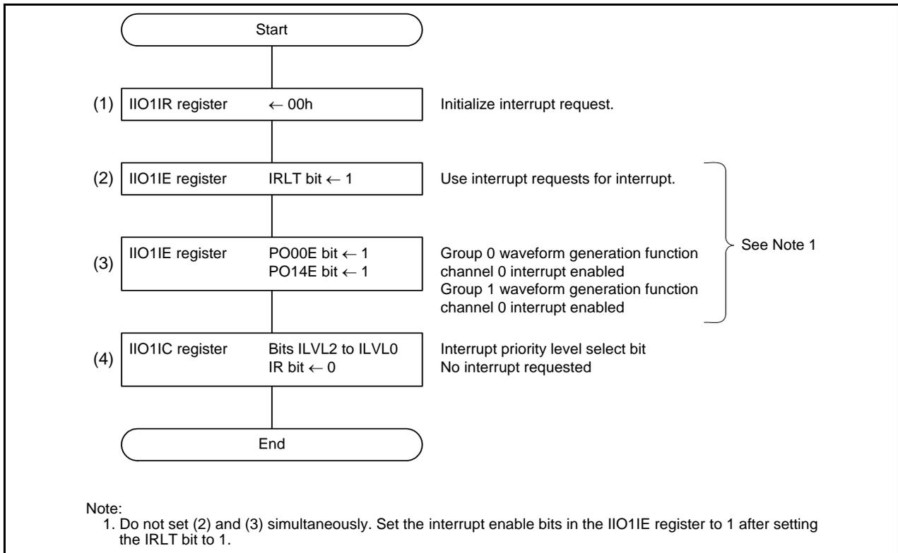
**Figure 4.2 Register Setting Procedure of Intelligent I/O Interrupt 1**
