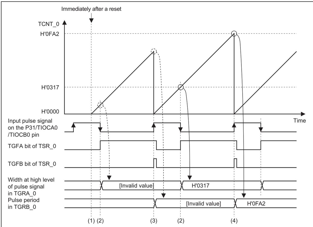
**Figure 4 Example of Operation to Measure the Width at High Level and Period of a Pulse Signal by Using the Input-Output Multiplexing Function of a TPU Pin**
