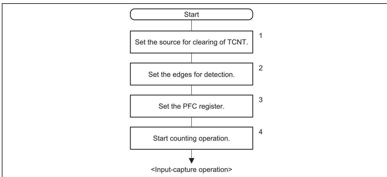
**Figure 3 Example of Settings to Apply the Input–Output Multiplexing Function of a TPU Pin for Measuring the Width at High Level and Period of a Pulse Signal**
