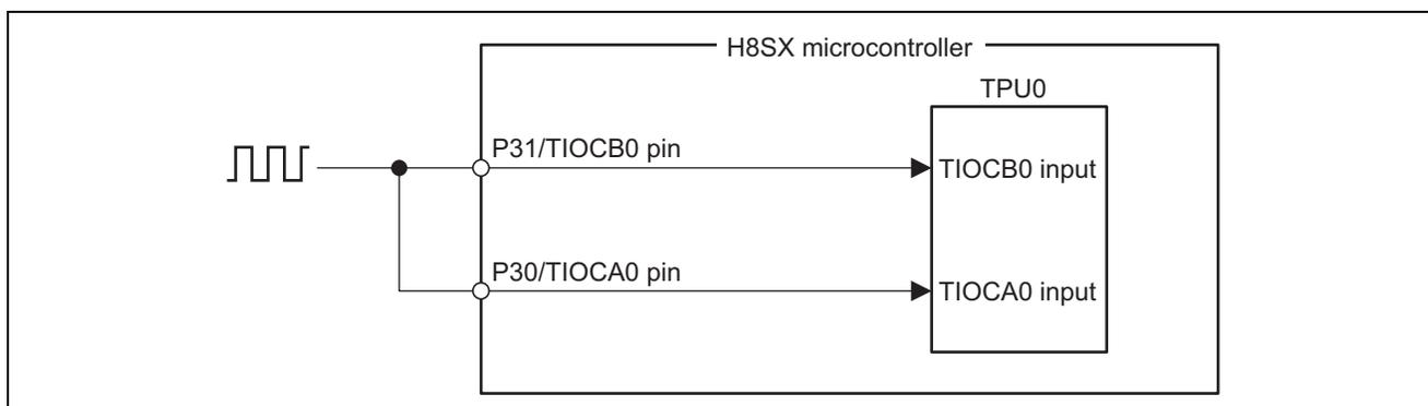
Figure 1 Example of the Usual form of Connection for Pulse Measurement
