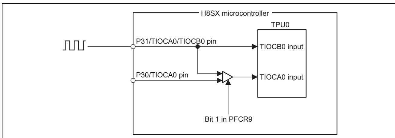
Figure 2 Example of the Connection for Pulse Measurement when the Multiplexing Function for TPU Input-Output Pins is Applied
