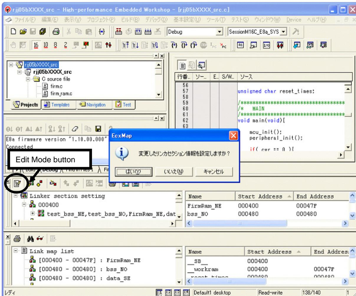
(7) test\_bss\_NE and test\_bss\_NO sections are assigned.
