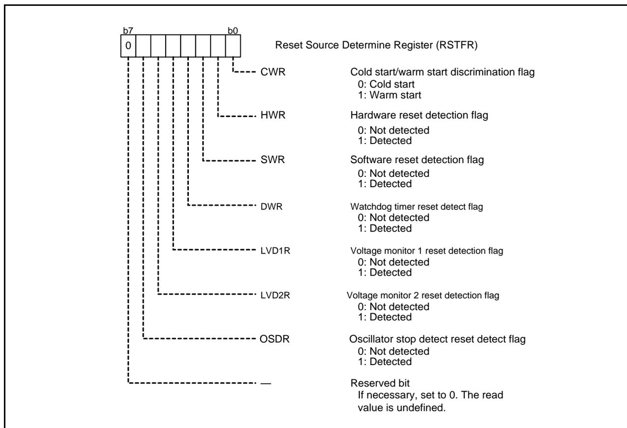
**Figure 3.1 Reset Source Determine Register**
