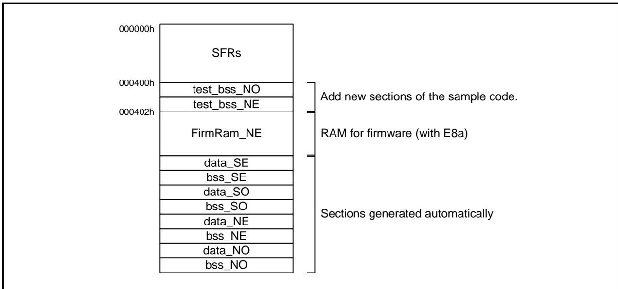
Figure 4.1 Application Example of Section Assignment
