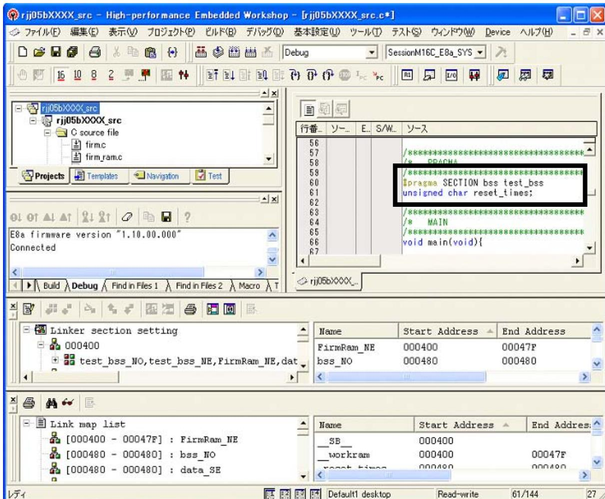
(9) When executing the build, the variable reset\_times is assigned to the test\_bss\_NO section.
