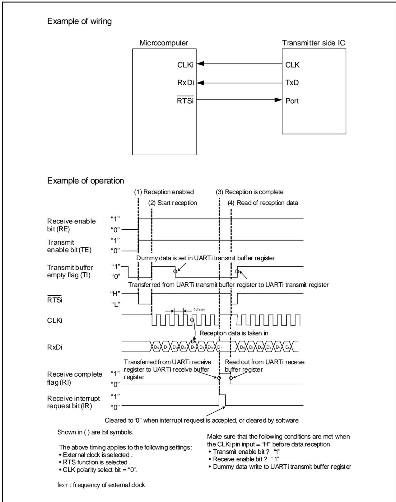
**Figure 4.1 Operation Timing of Reception in Clock-Synchronous Serial I/O Mode**
