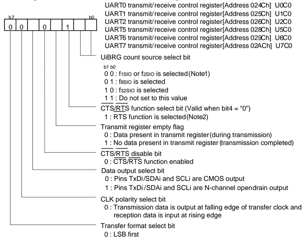
Note 1: When the PCLK1 bit in the PCLKR register is "1", the selected clock source is f1sio. When the PCLK1 bit is "0", the selected clock source is f2sio.
