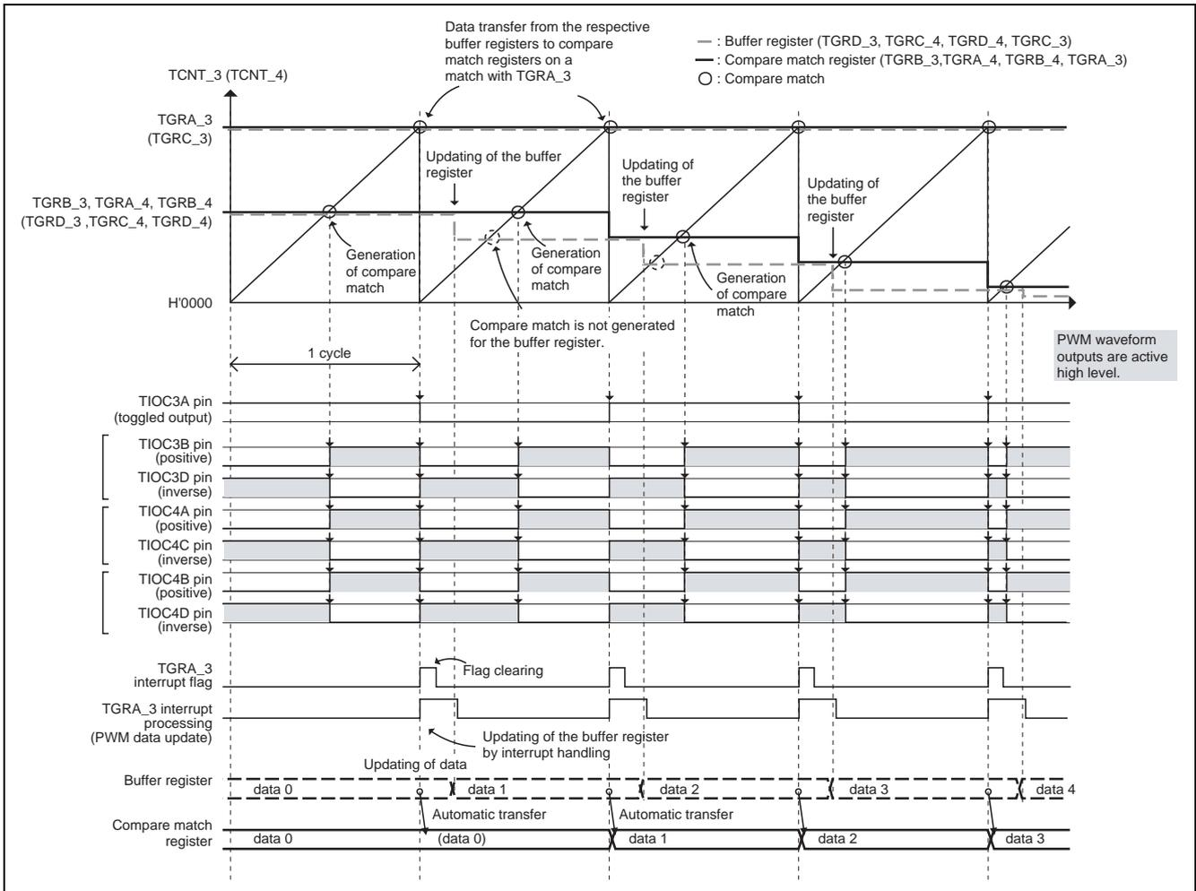
Figure 4 Operation (Buffered Operation) in Reset-Synchronized PWM Mode
