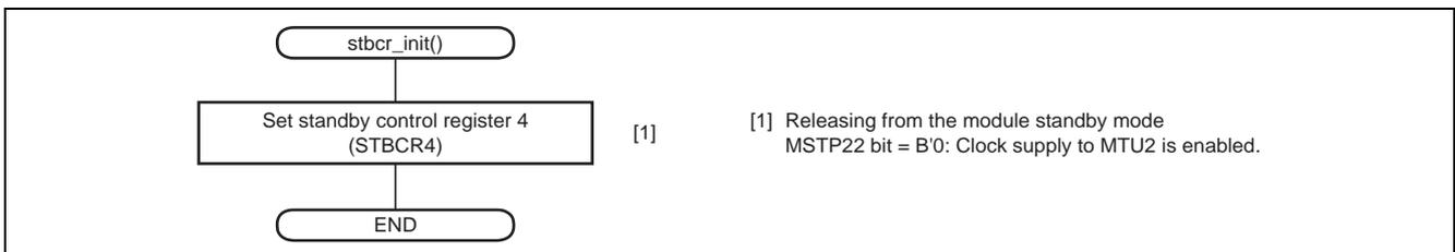
Figure 7 Setting for Release of the Module from Standby
