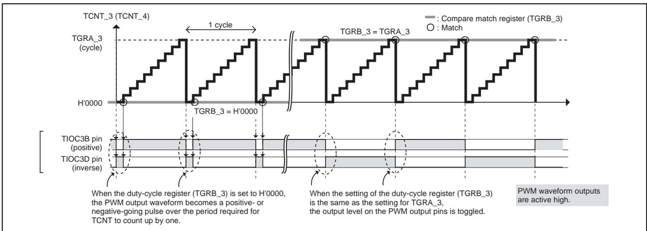
Figure 5 Settings of the Duty-Cycle Register and Corresponding PWM Output Waveforms
