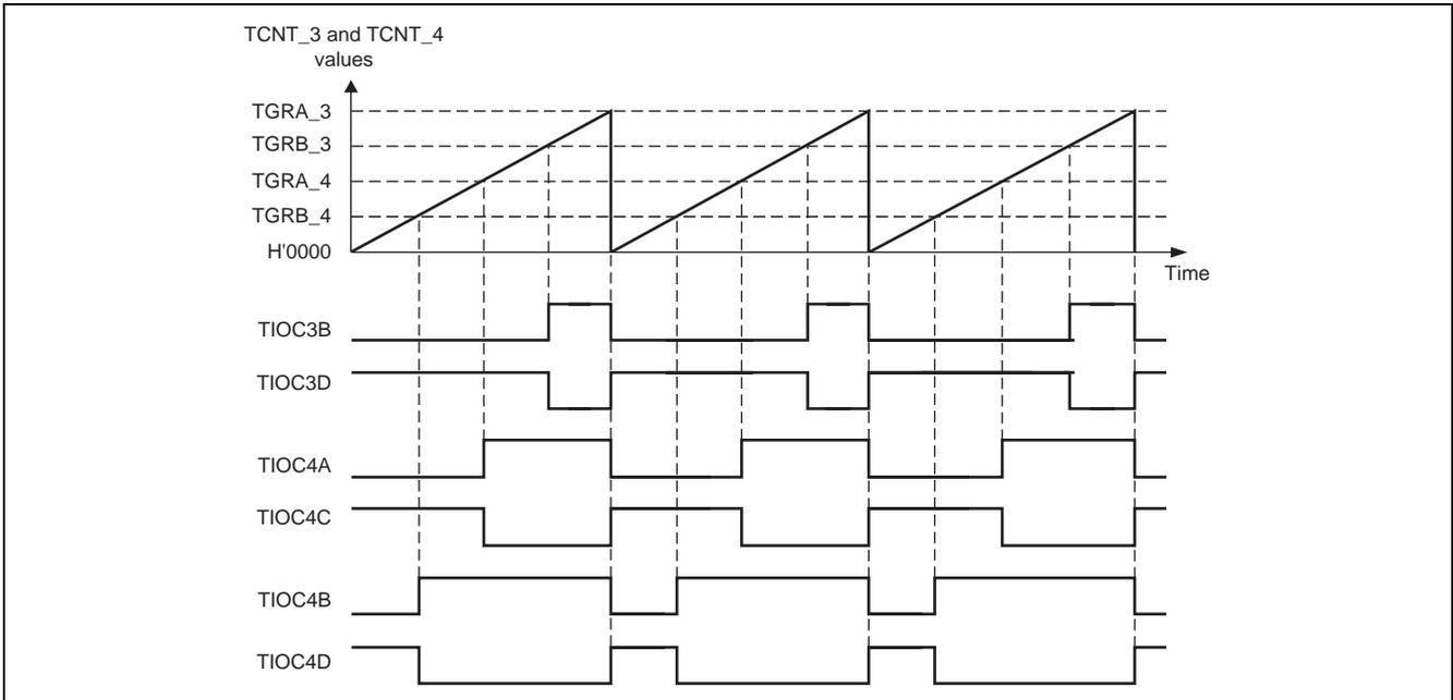
**Figure 3 Sample Timing of Operation in Reset-Synchronized PWM Mode
