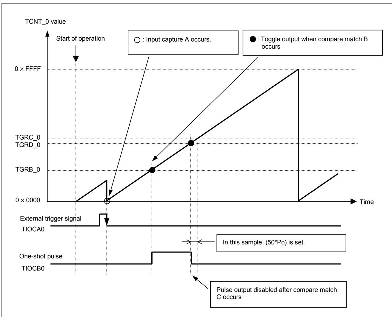
**Figure 3 Example of One-Shot Pulse Output Operation**
