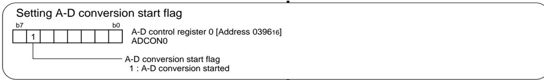
Repeatedly carries out A-D conversion on pins selected through the A-D sweep pin select bit. **Start A-D conversion**
