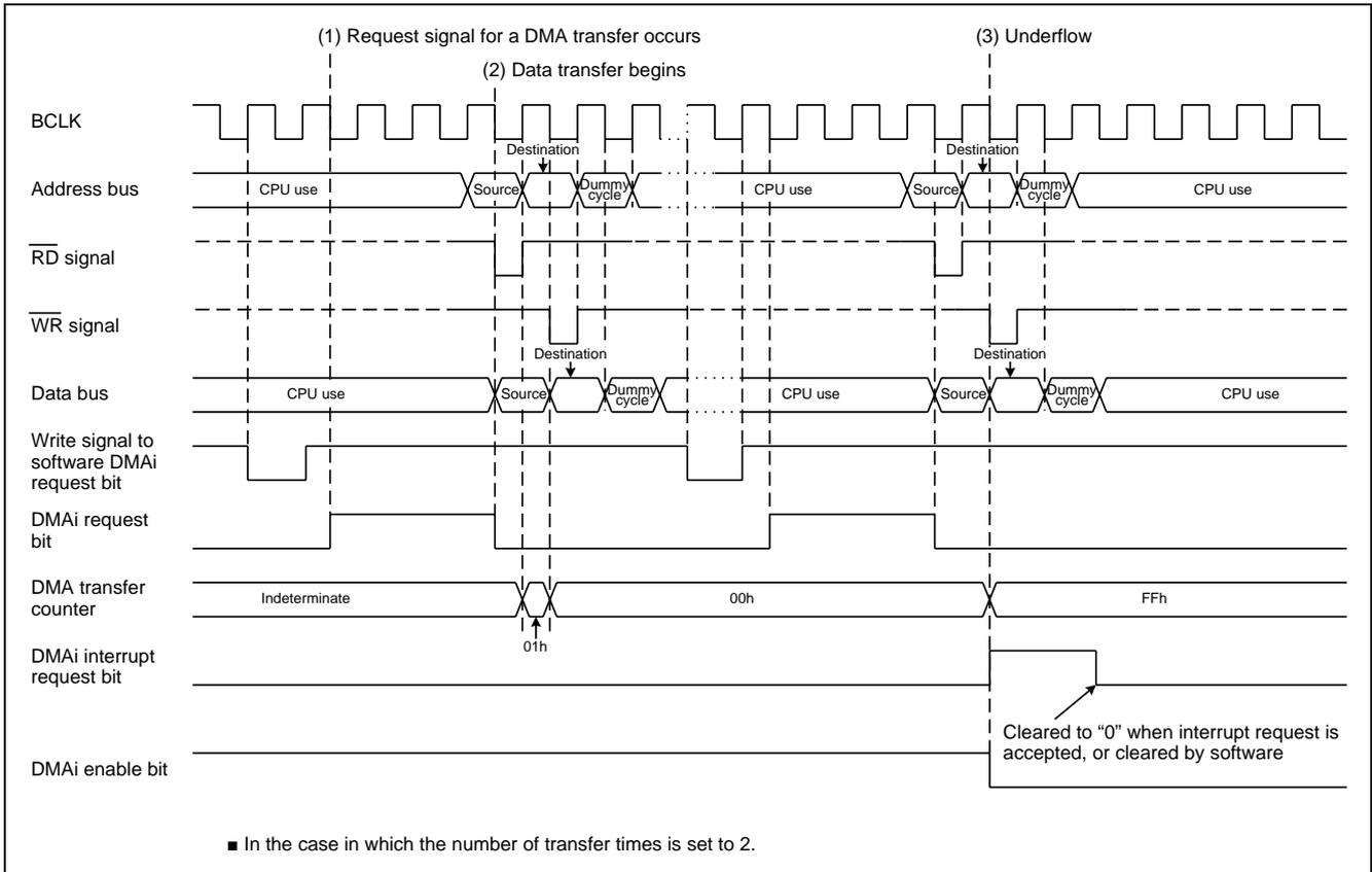
Figure 1. Example of operation of one-shot transfer mode
