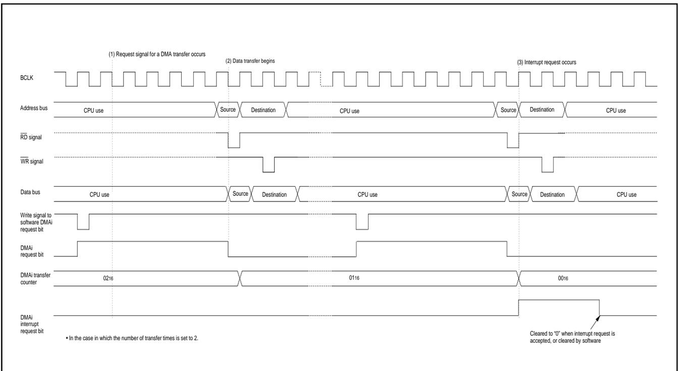
**Figure 1. Example of operation of one-shot transfer mode**
