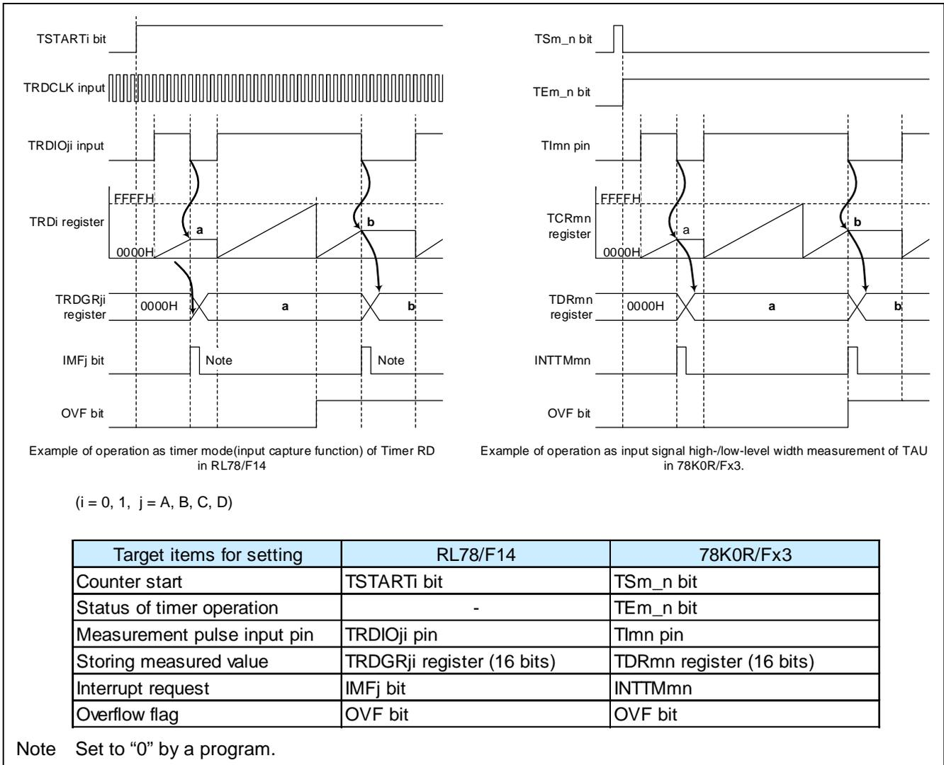
**Figure 15-19 Comparison of operation between timer mode in RL78/F14 and input signal high-/low-level width measurement in 78K0R/Fx3**
