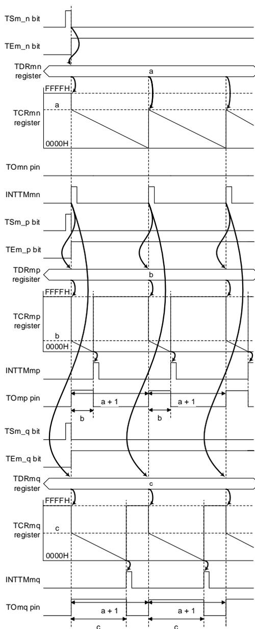
Example of operation as multiple PWM output of TAU in 78K0R/Fx3
