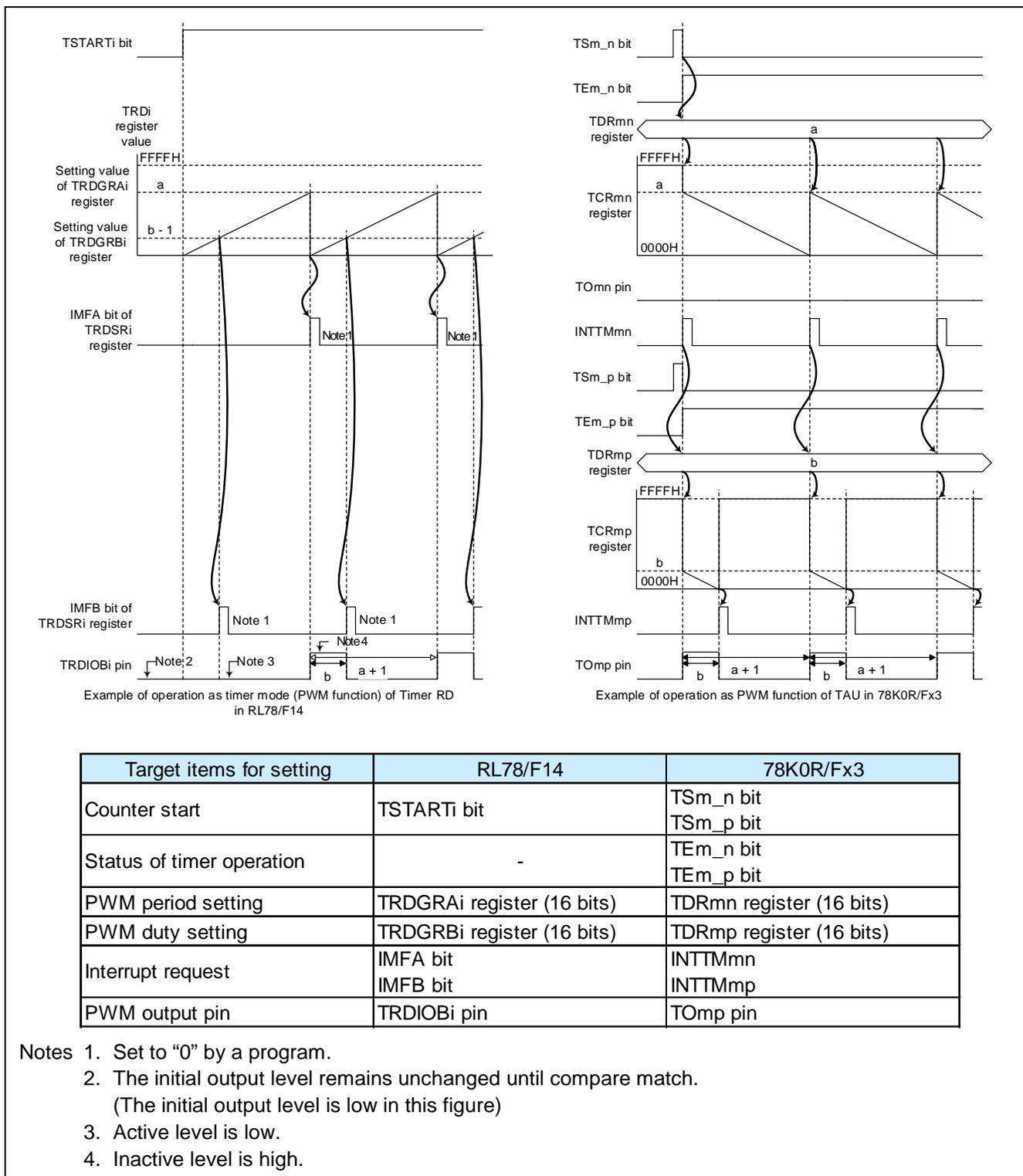
**Figure 15-20 Comparison of operation between timer mode (PWM function) in RL78/F14 and PWM function in 78K0R/Fx3**
