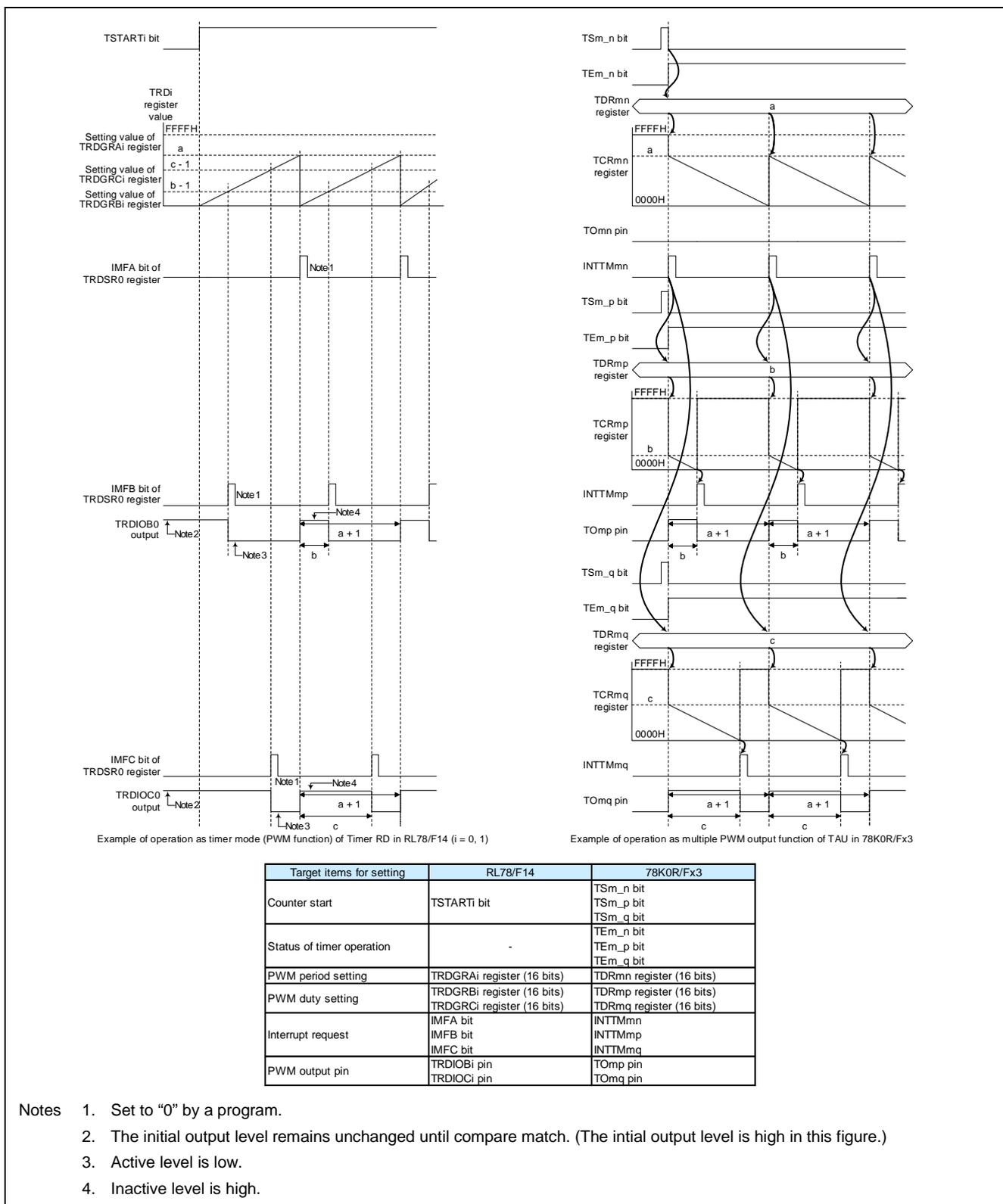
Figure 15-21 Comparison of operation between timer mode (PWM function) in RL78/F14 and multiple PWM output function in 78K0R/Fx3
