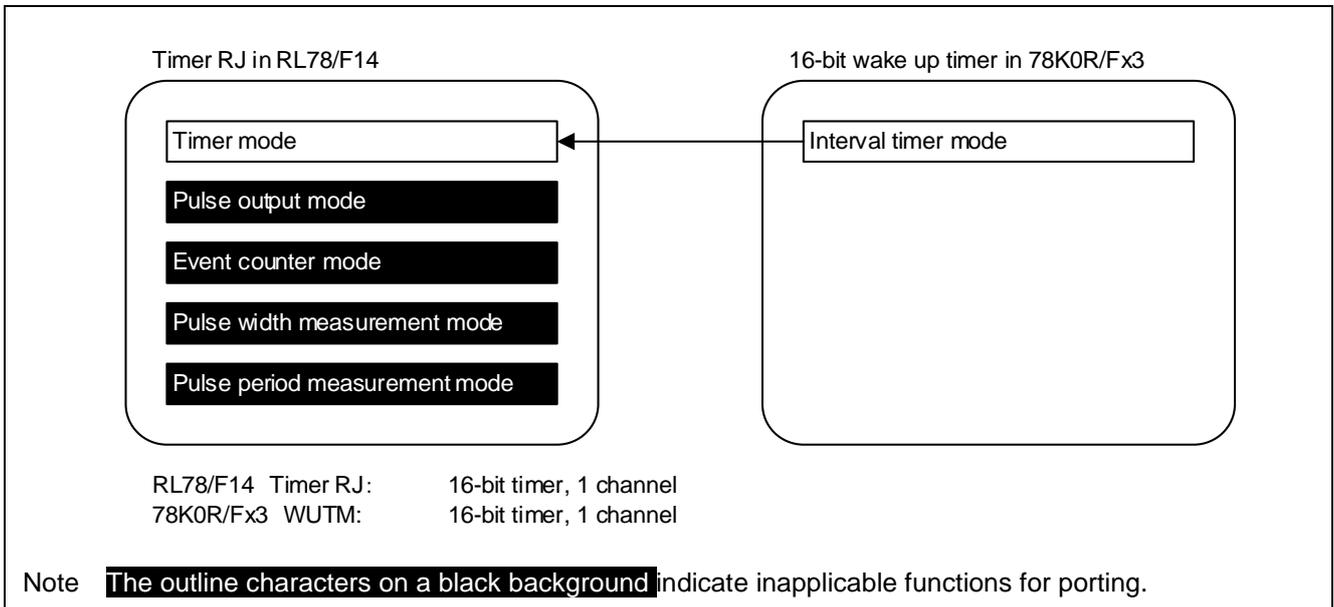
Figure 15-11 Relationship between each mode of Timer RJ in RL78/F14 and that of 16-bit WUTM in 78K0R/Fx3
