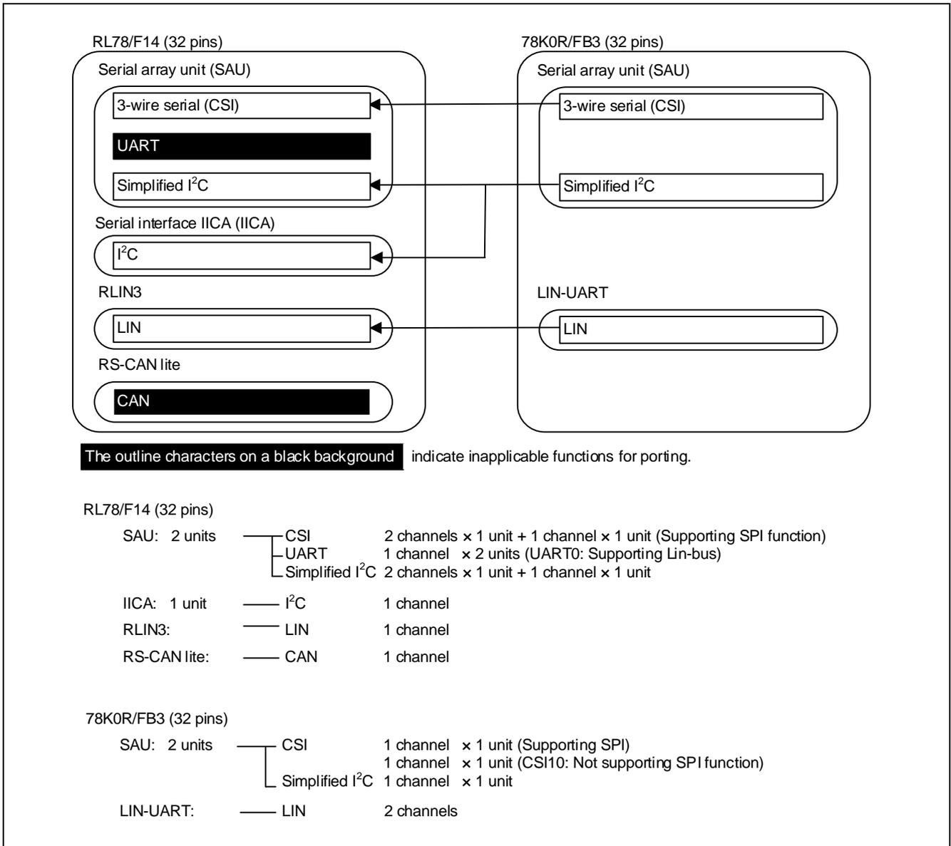
Figure 16-6 Relationship between each communication mode of serial interface in RL78/F14 (32 pins) and that in 78K0R/FB3 (32 pins)
