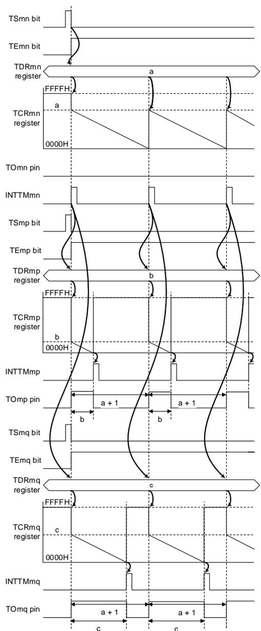
Example of operation as multiple PWM output of TAU in RL78/F14
