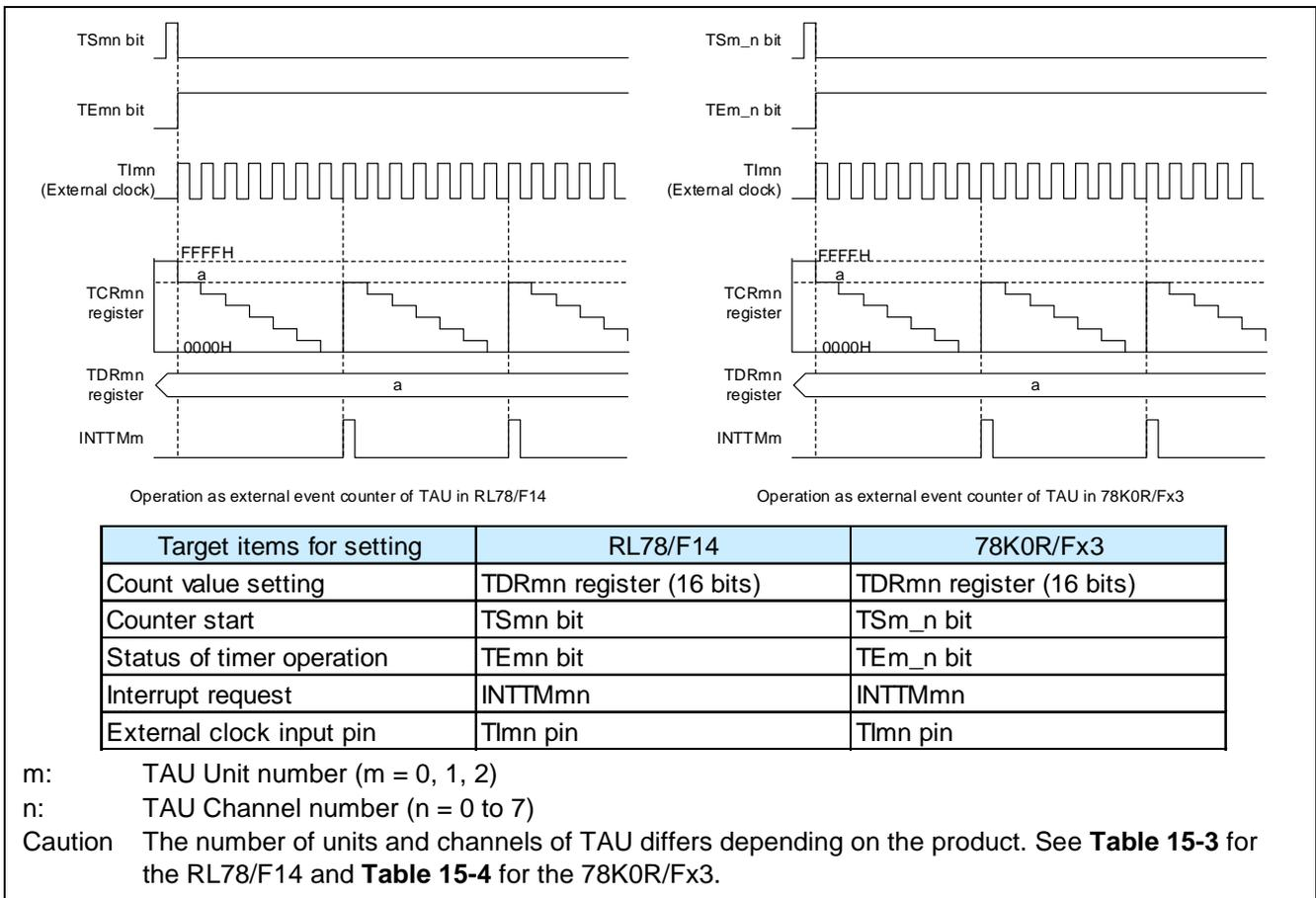
**Figure 15-4 Comparison of operation as external event counter of TAU between RL78/F14 and 78K0R/Fx3**
