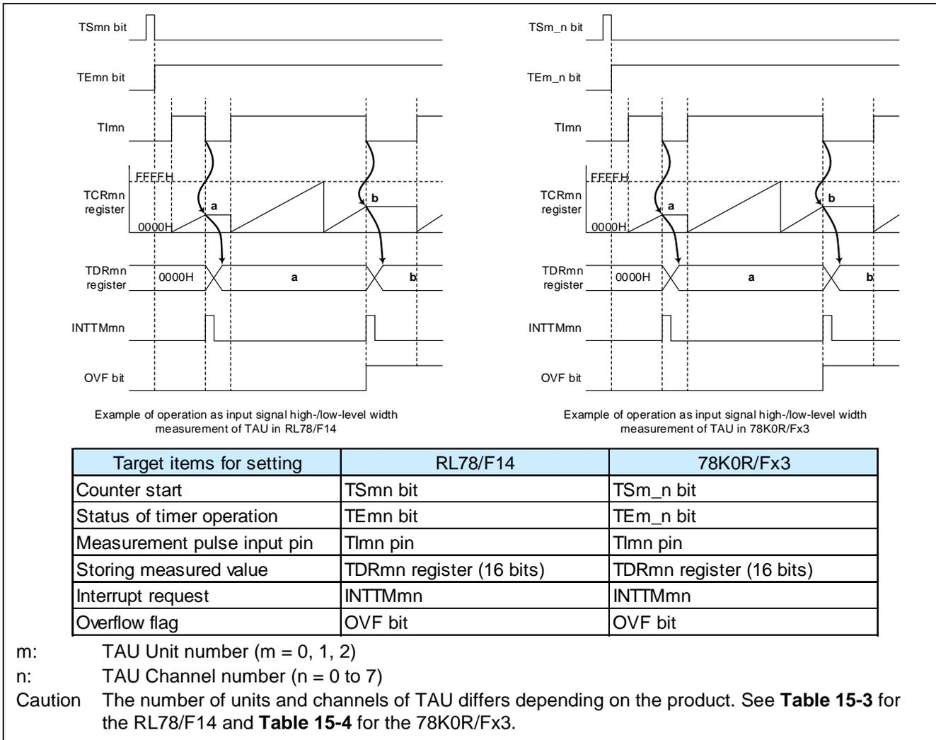
**Figure 15-7 Comparison of operation as input signal high-/low-level width measurement of TAU between RL78/F14 and 78K0R/Fx3**
