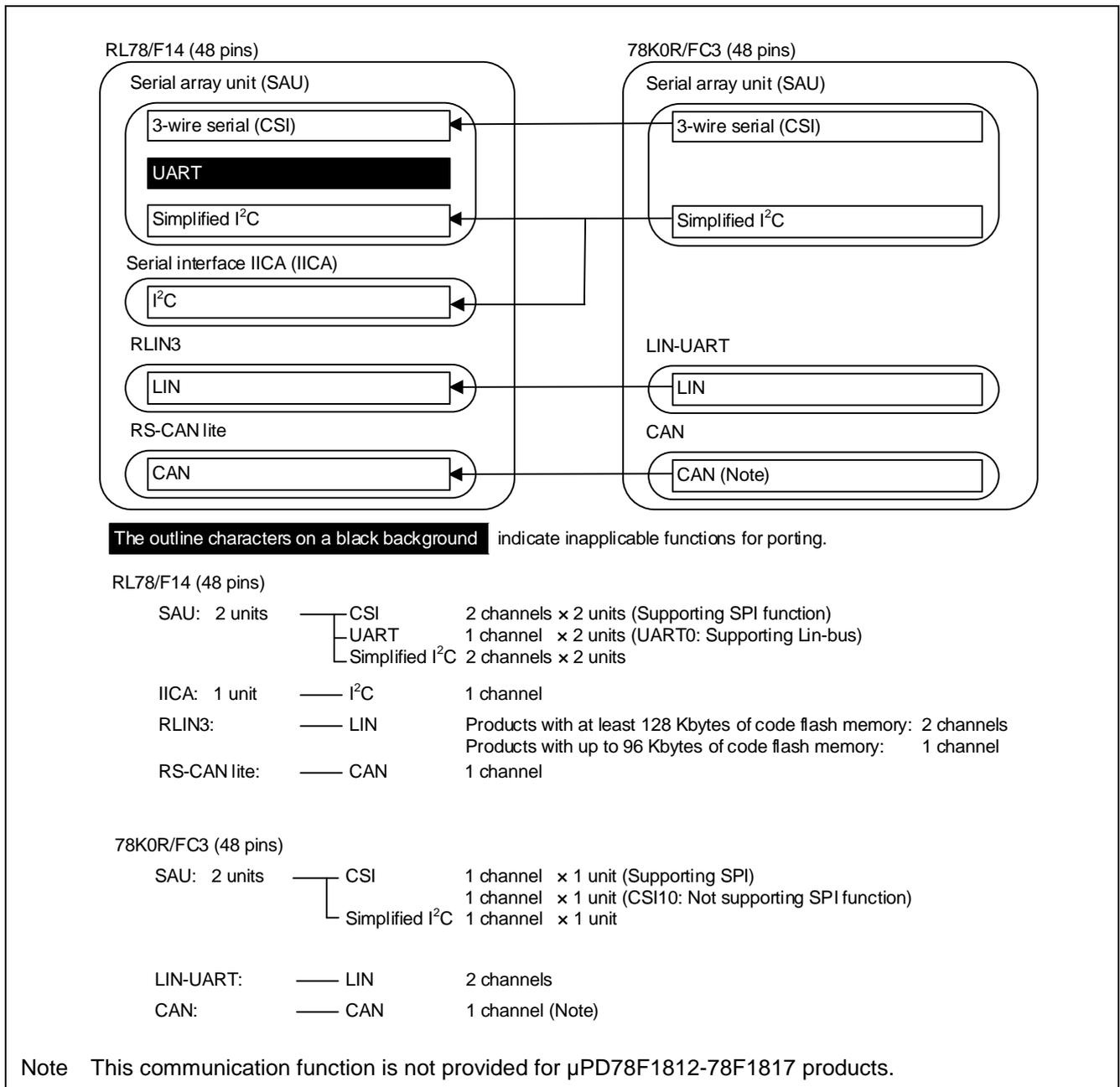
**Figure 16-4 Relationship between each communication mode of serial interface in RL78/F14 (48 pins) and that in 78K0R/FC3 (48 pins)**
