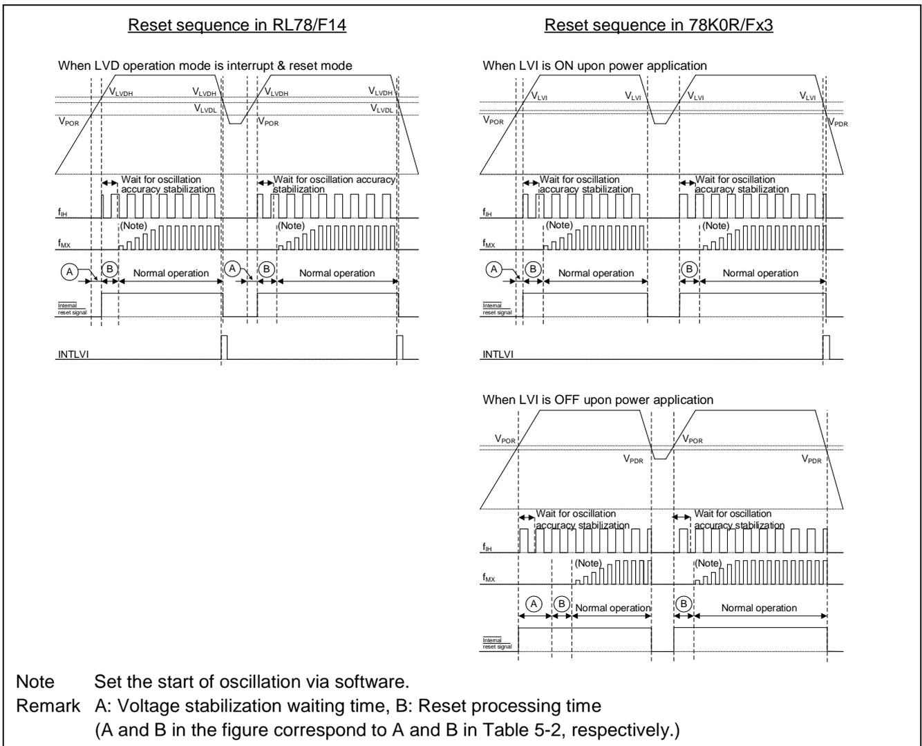
Figure 5-2 Comparison of reset sequences between RL78/F14 and 78K0R/Fx3
