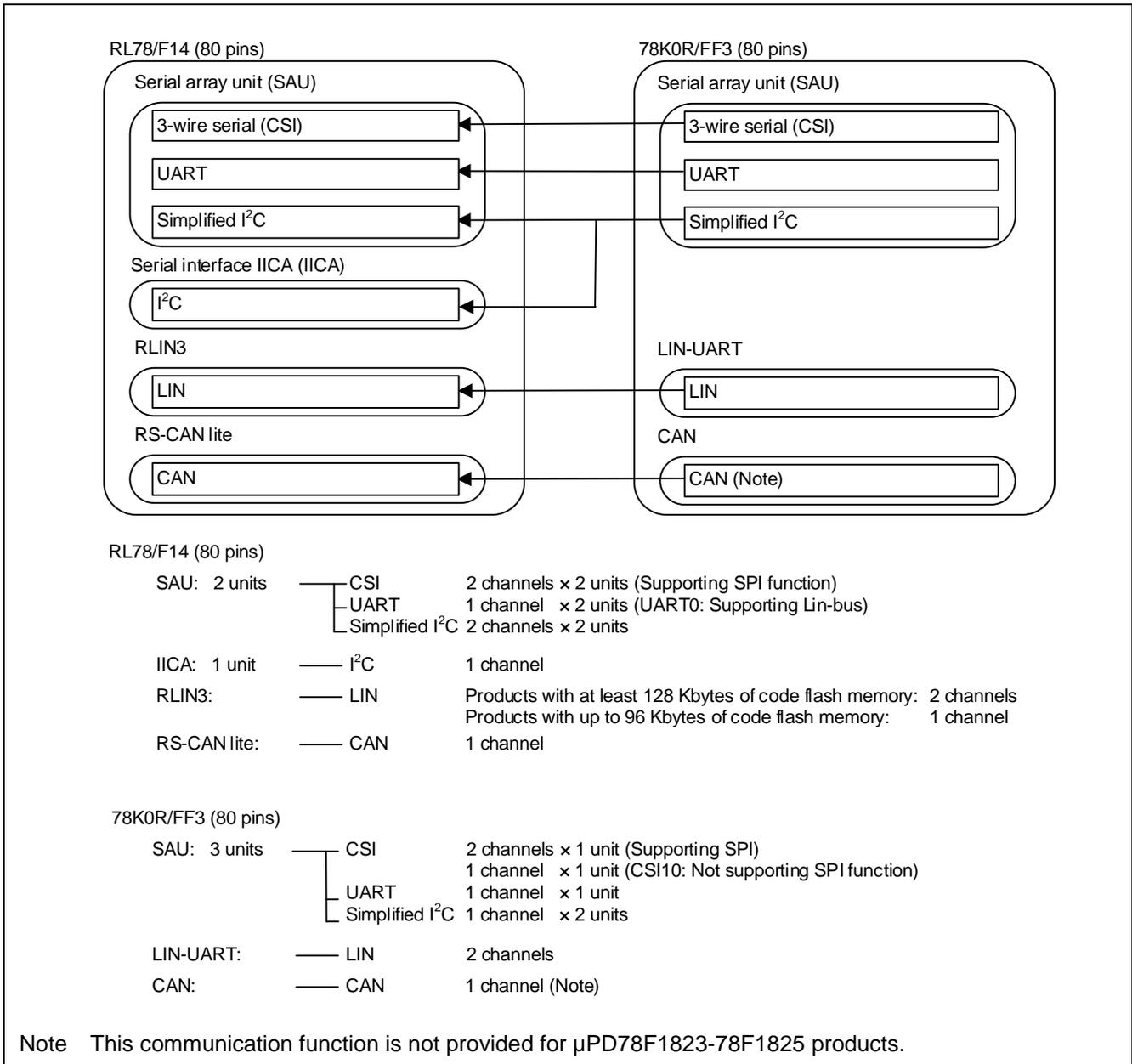
Figure 16-2 Relationship between each communication mode of serial interface in RL78/F14 (80 pins) and that in 78K0R/FF3
