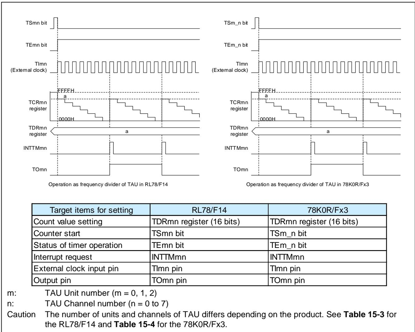
**Figure 15-5 Comparison of operation as frequency divider of TAU between RL78/F14 and 78K0R/Fx3**
