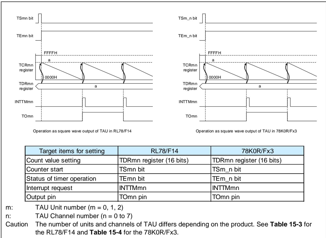
**Figure 15-3 Comparison of operation as square wave output of TAU between RL78/F14 and 78K0R/Fx3**
