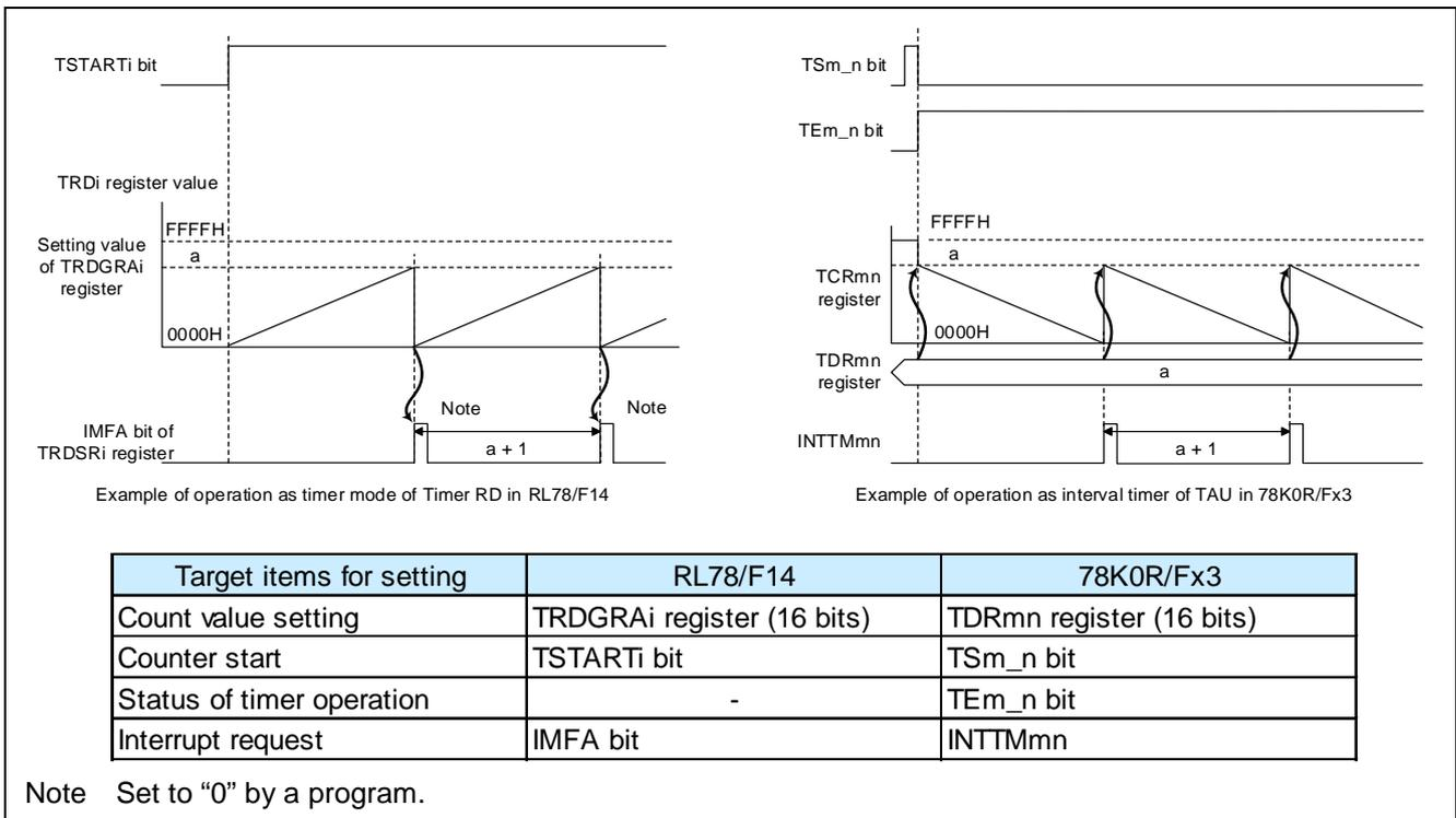
**Figure 15-14 Comparison of operation between timer mode in RL78/F14 and interval timer in 78K0R/Fx3**
