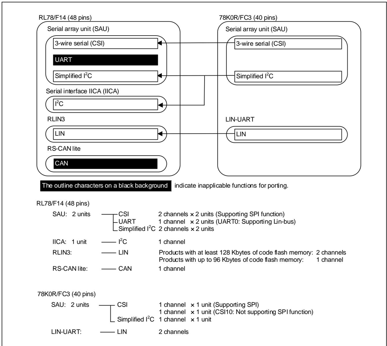
Figure 16-5 Relationship between each communication mode of serial interface in RL78/F14 (48 pins) and that in 78K0R/FC3 (40 pins)
