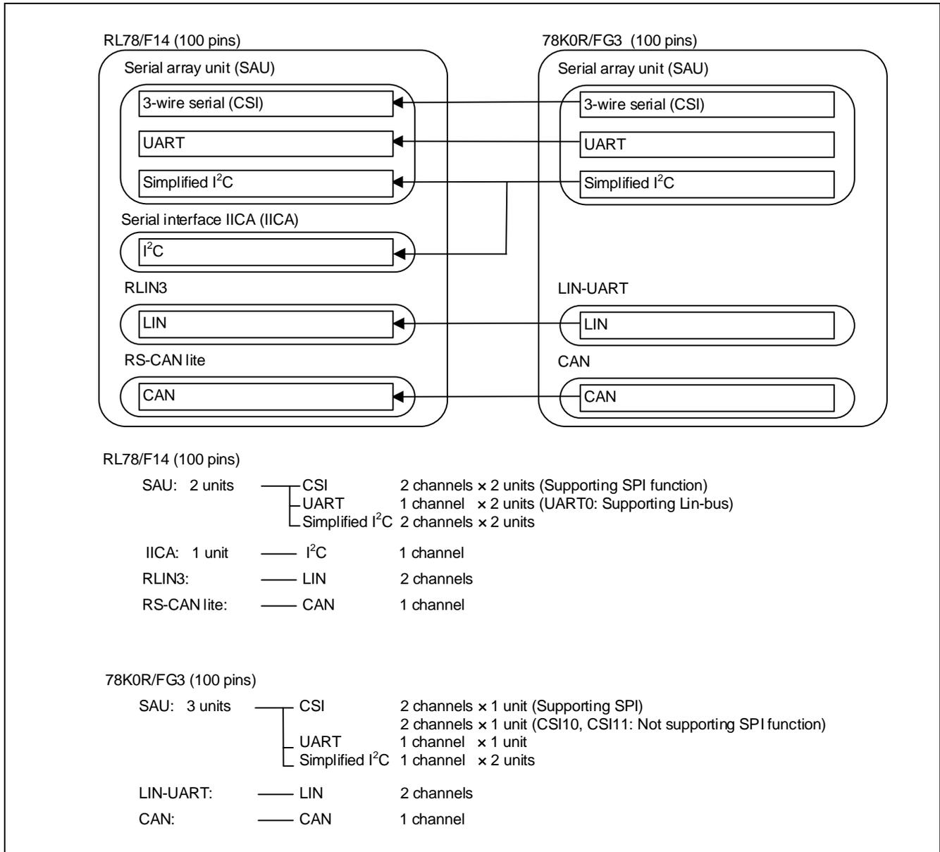
**Figure 16-1 Relationship between each communication mode of serial interface in RL78/F14 (100 pins) and that in 78K0R/FG3**
