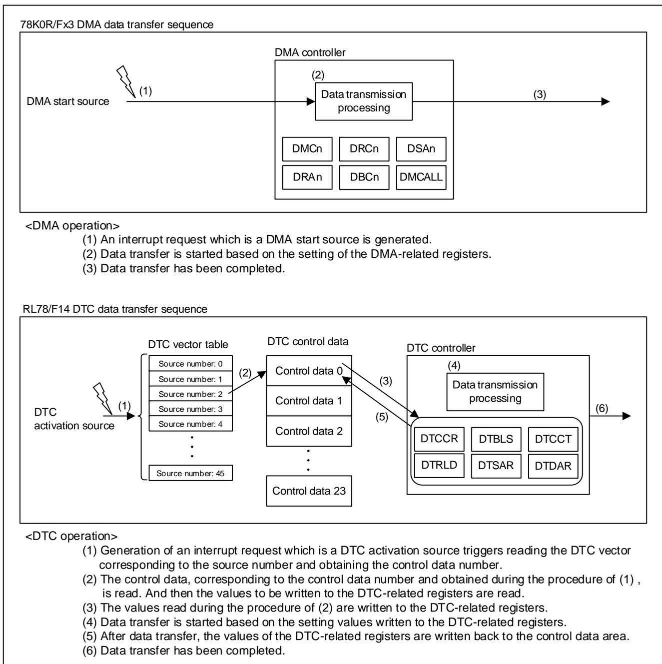
**Figure 14-1 Comparison between DTC data transfer sequence in RL78/F14 and DMA data transfer sequence in 78K0R/Fx3**
