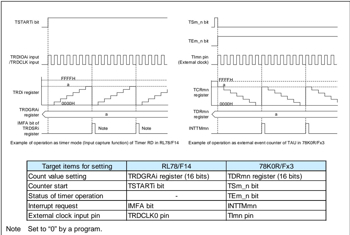
**Figure 15-16 Comparison of operation between timer mode in RL78/F14 and external event counter in 78K0R/Fx3**
