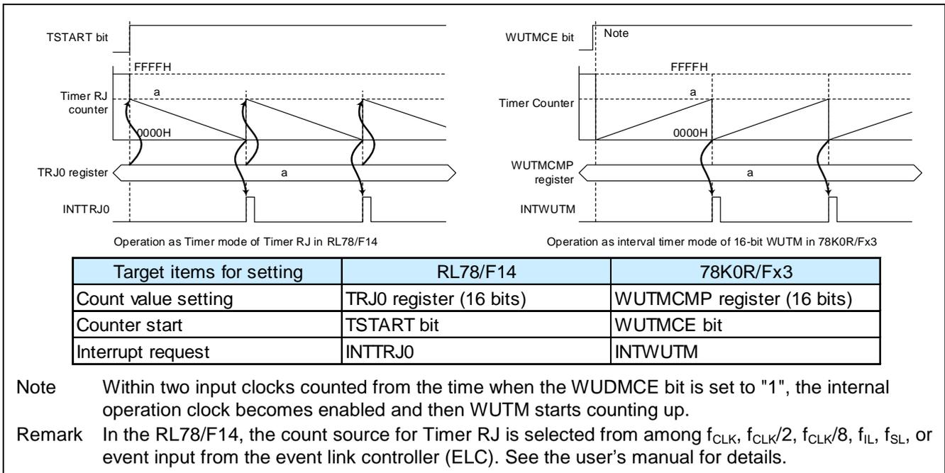
Figure 15-12 Comparison of 16-bit WUTM operation and Timer RJ operation
