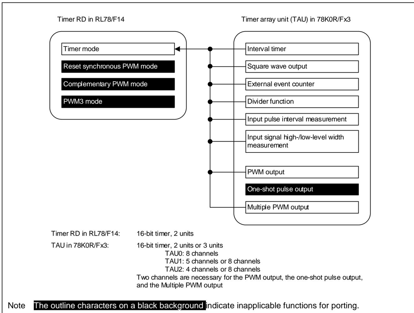
**Figure 15-13 Relationship between each mode of Timer RD in RL78/F14 and that of TAU in 78K0R/Fx3**
