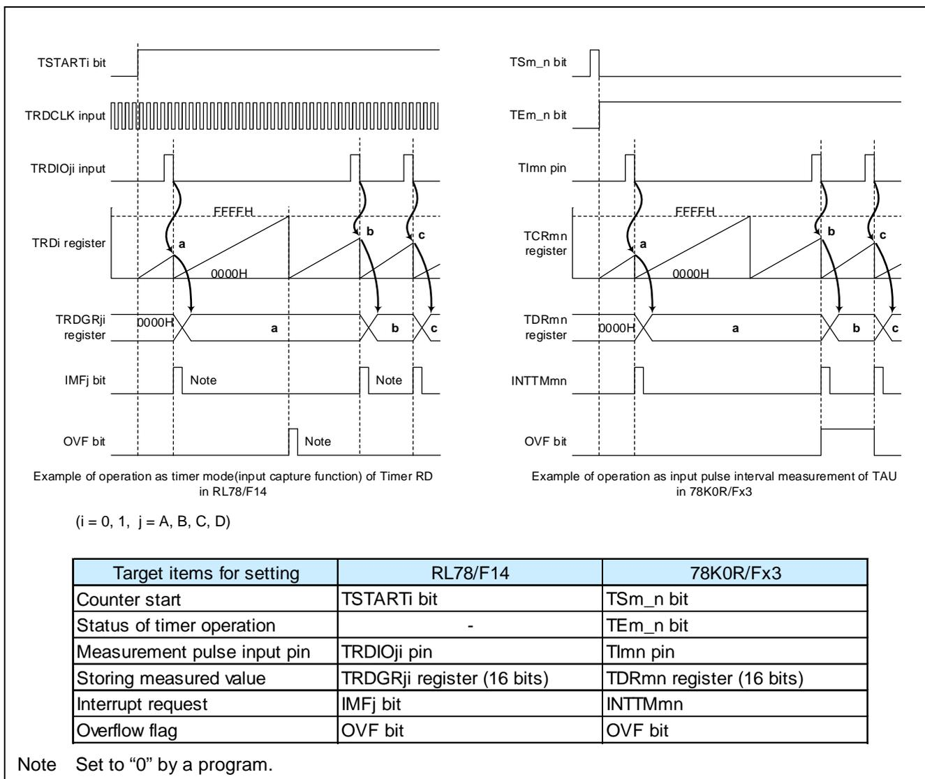
**Figure 15-18 Comparison of operation between timer mode in RL78/F14 and input pulse interval measurement in 78K0R/Fx3**
