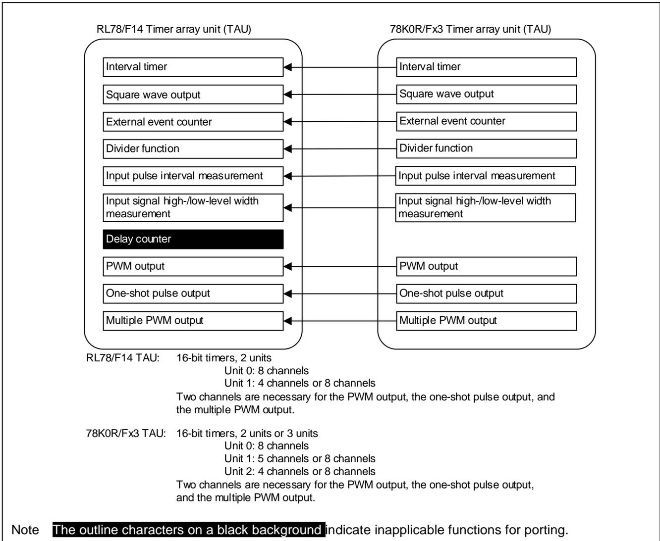
**Figure 15-1 Relationship between each mode of TAU in RL78/F14 and that in 78K0R/Fx3**
