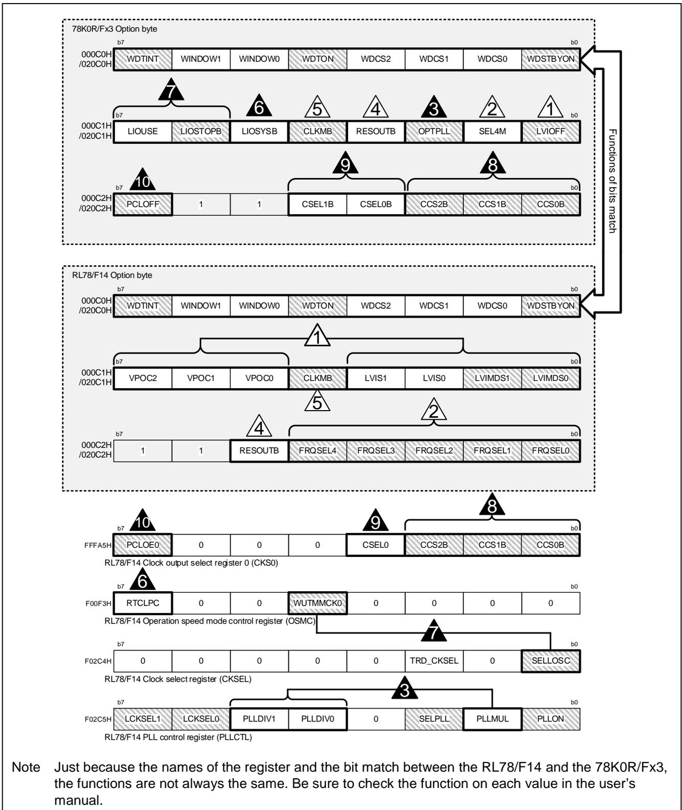
**Figure 9-1 Comparison of register configuration of option byte between RL78/F14 and 78K0R/Fx3**
