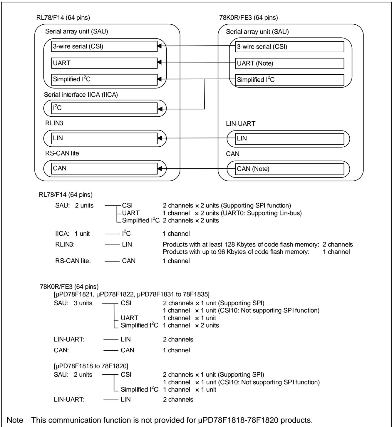
Figure 16-3 Relationship between each communication mode of serial interface in RL78/F14 (64 pins) and that in 78K0R/FE3
