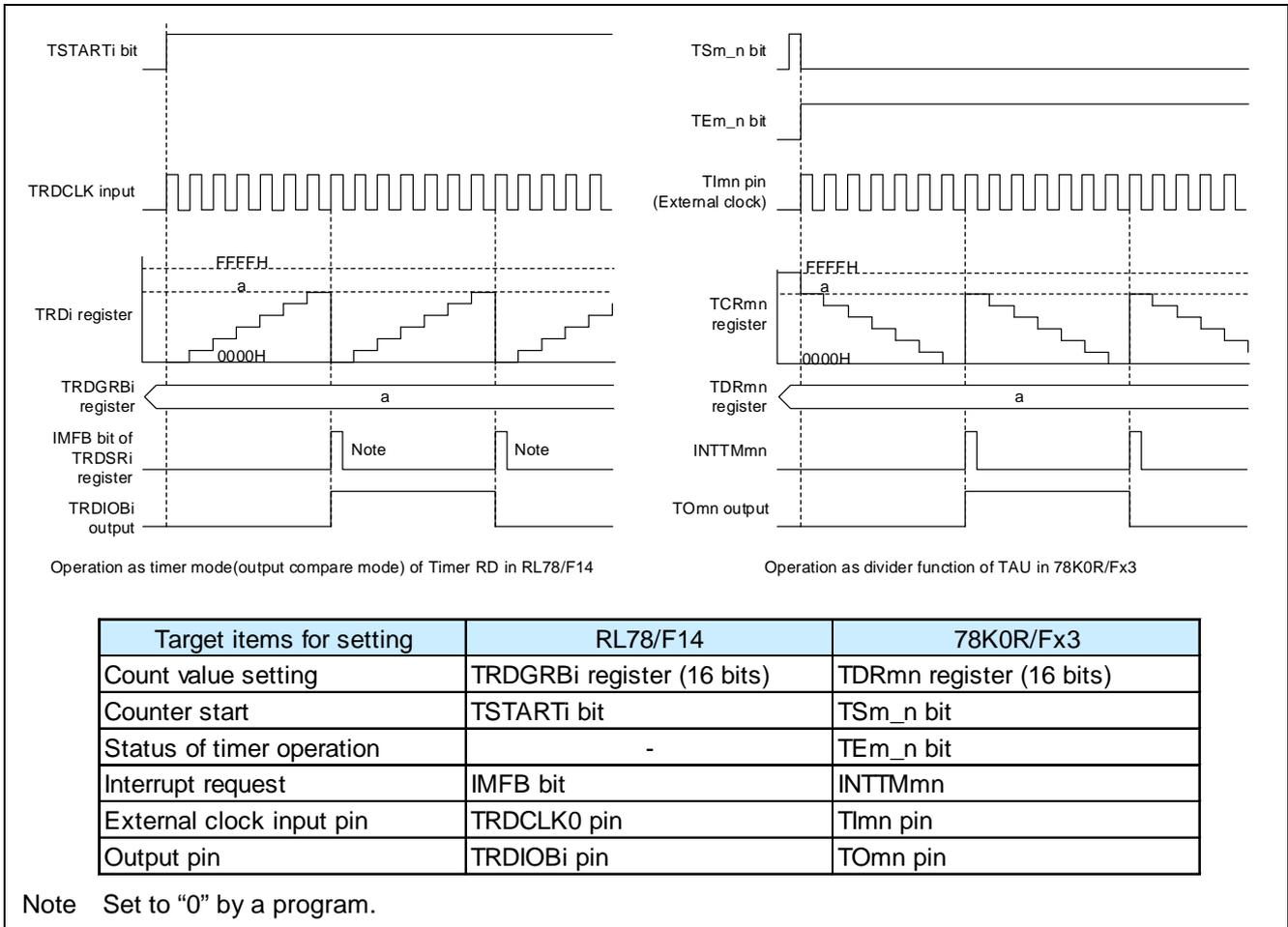
**Figure 15-17 Comparison of operation between timer mode in RL78/F14 and divider function in 78K0R/Fx3**
