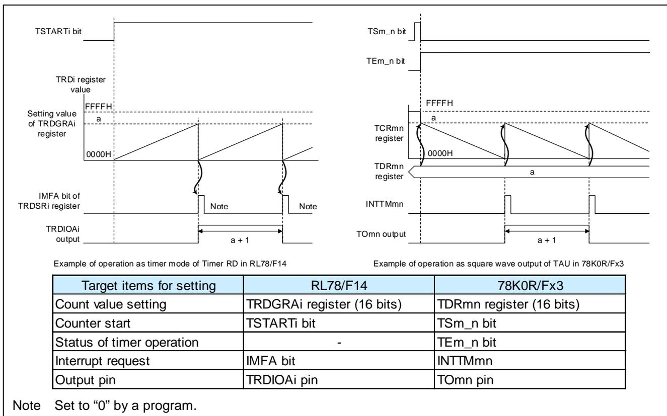
**Figure 15-15 Comparison of operation between timer mode in RL78/F14 and square wave output in 78K0R/Fx3**
