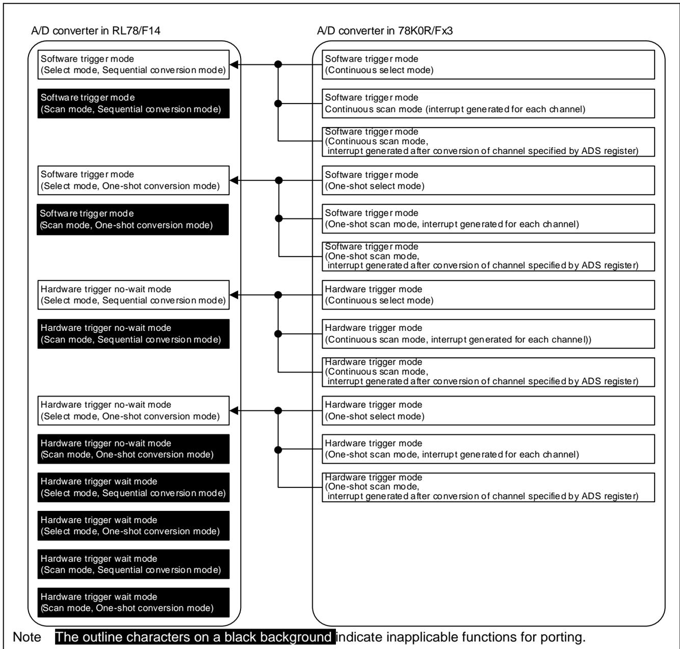
**Figure 17-1 Relationship between each mode of A/D converter in RL78/F14 and that in 78K0R/Fx3**
