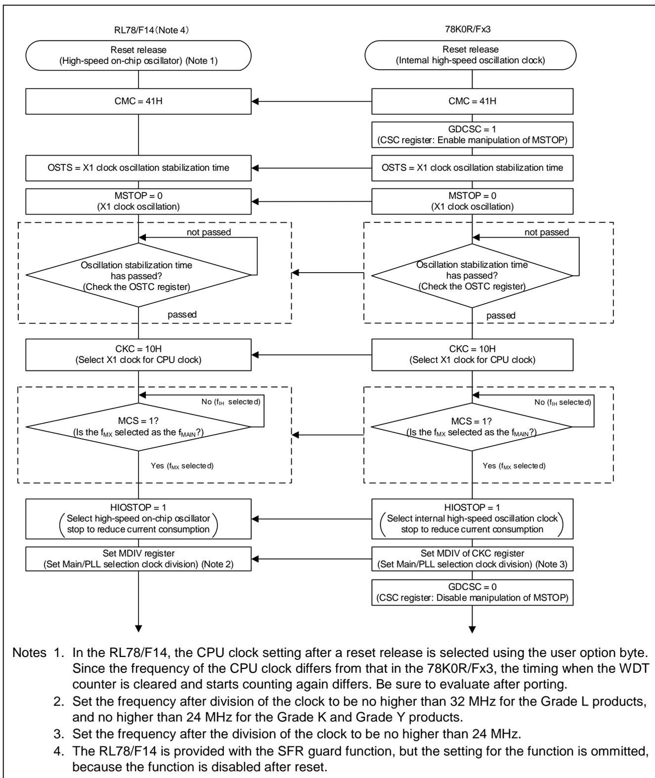
Figure 7-1 Procedure for setting X1 Clock after reset in RL78/F14 and 78K0R/Fx3
