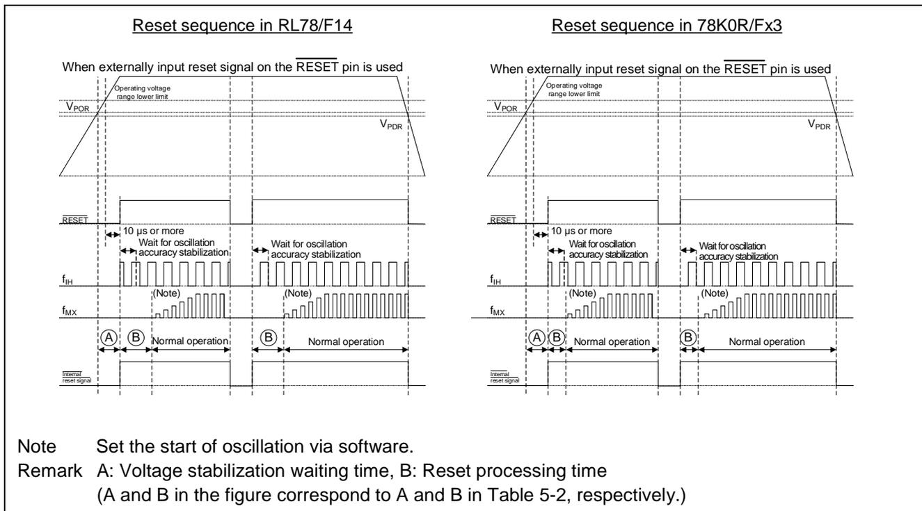
**Figure 5-1 Comparison of reset sequences by  $\overline{RESET}$  pins between RL78/F14 and 78K0R/Fx3**
