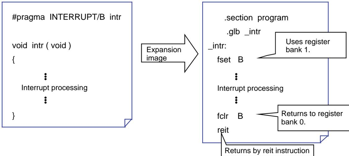
**Figure 2.5.2 Image Depicting Expansion of Fast Interrupt Processing Function**
