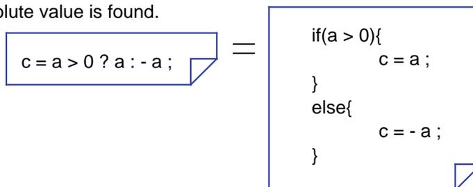
**Figure 1.3.3 Example for Using Conditional Operator**
