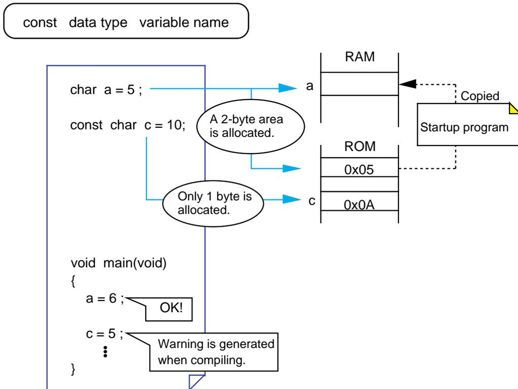
**Figure 2.1.6 const Modifier and Memory Mapping**
