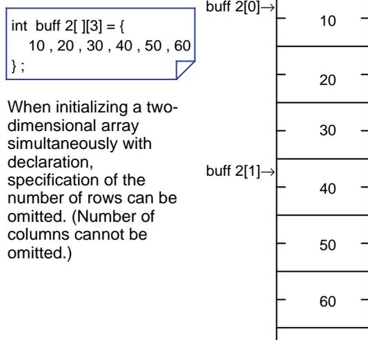
**Figure 1.7.3 Declaration of Two-dimensional Array and Memory Mapping**
