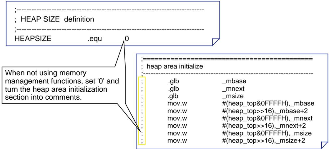
Figure 2.2.6 Setting the Heap Area
