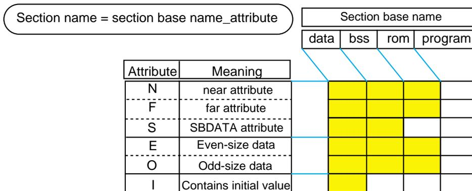
**Figure 2.1.4 Rule for Assigning Section Names**
