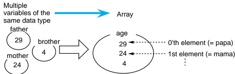
Figure 1.7.1 Concept of an Array
