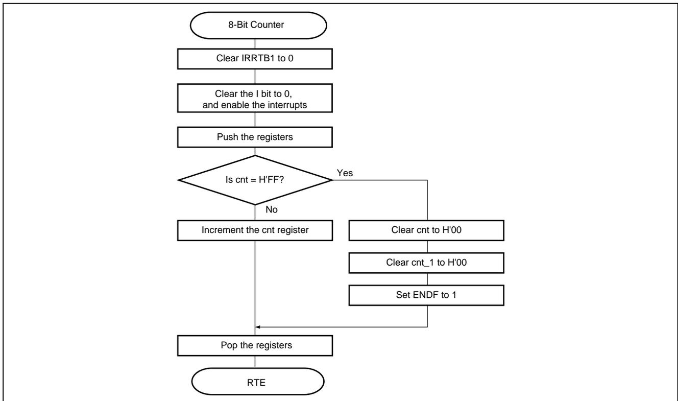
**Figure 5.2 Timer B1 Interrupt Service Routine**
