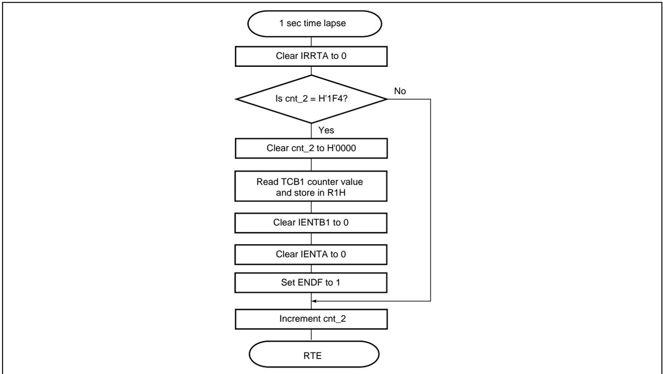
Figure 5.3 Timer V Interrupt Service Routine
