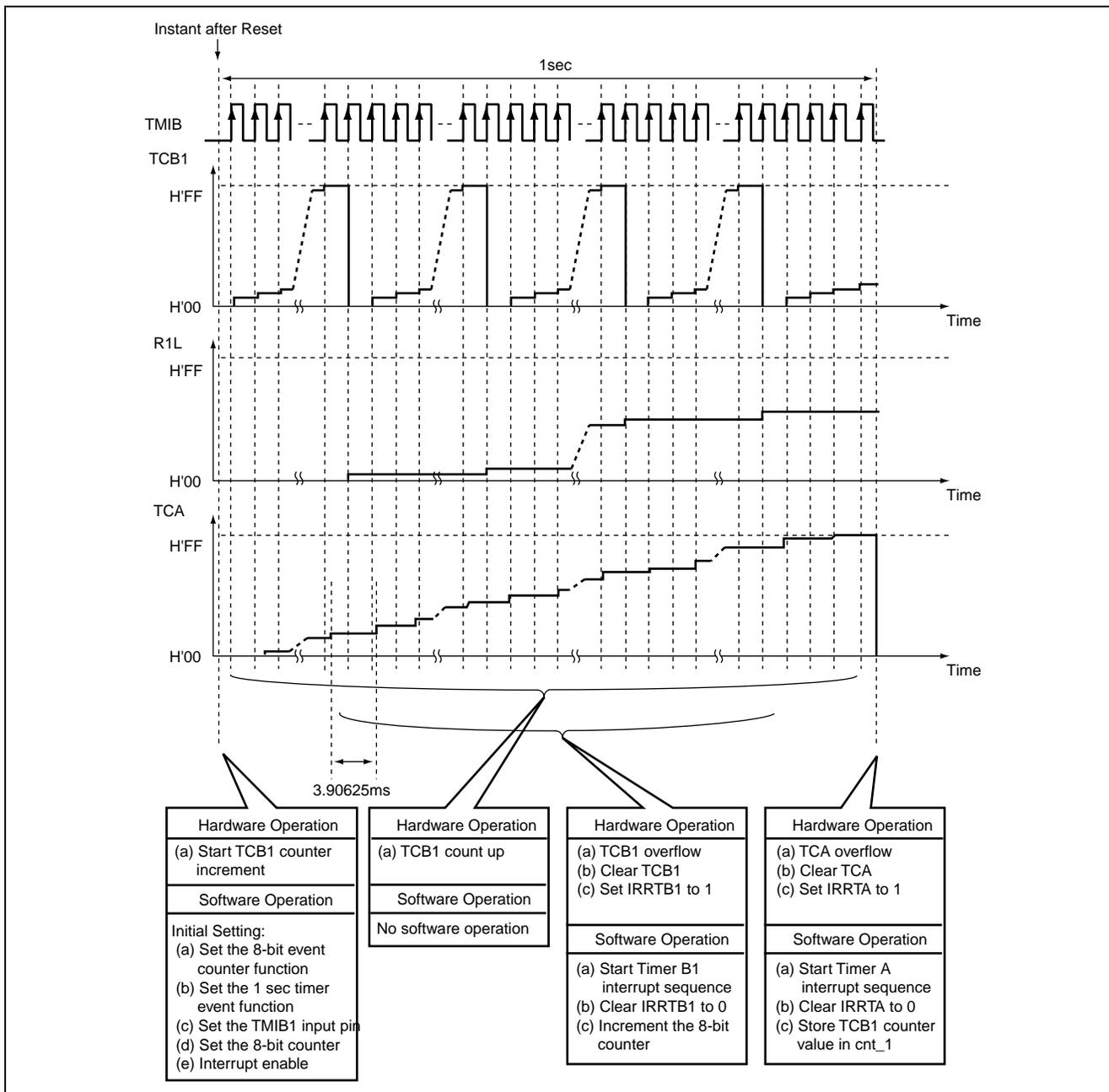
**Figure 3.1 Operating Principle of Frequency Measurement by Timer B1 Event Counter Function**
