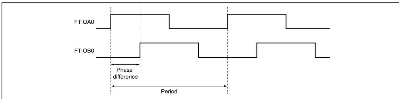
Figure 1.1 Outputting Pulses with a Desired Phase Difference
