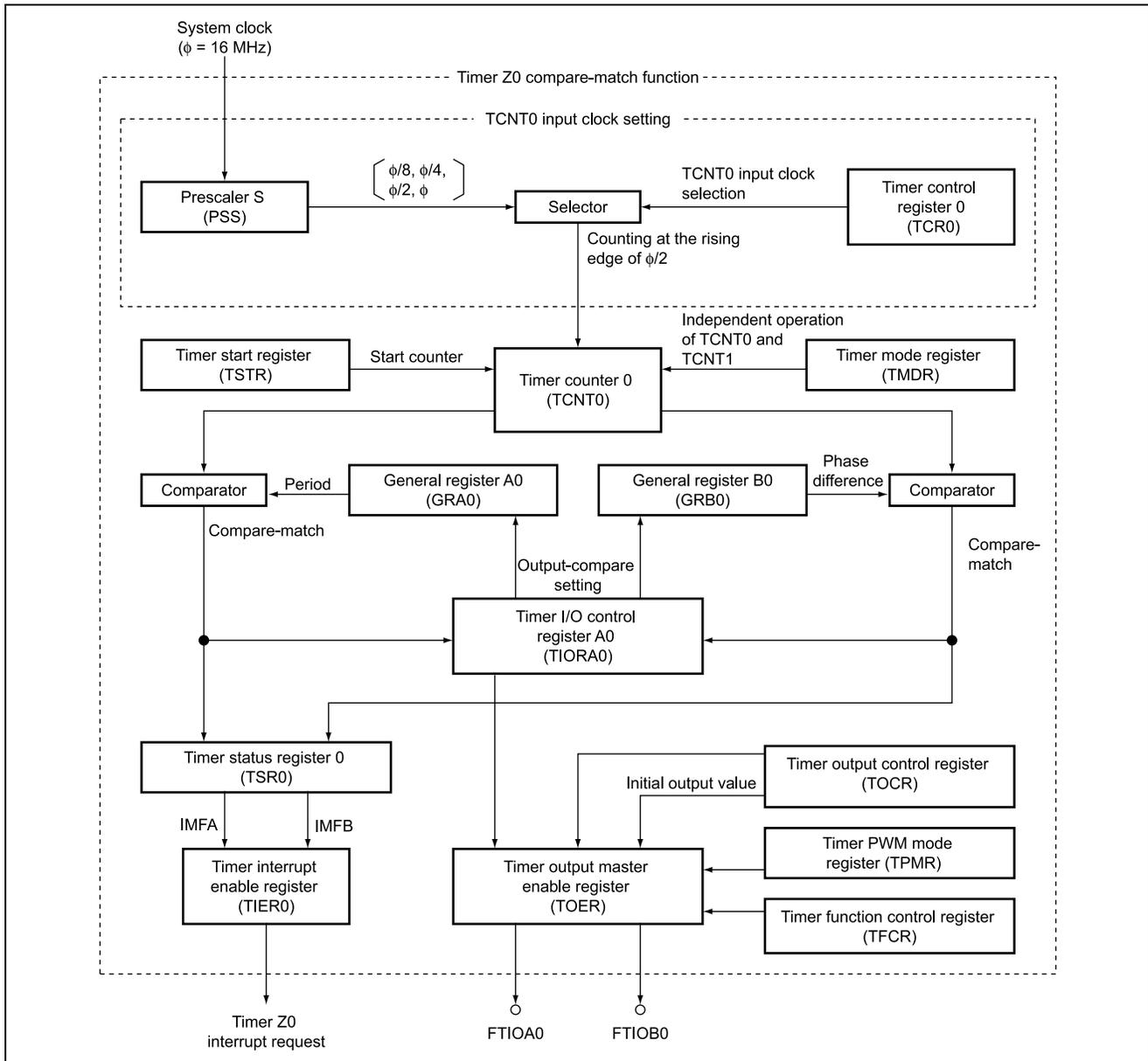
**Figure 2.1 Block Diagram of Timer Z0**
