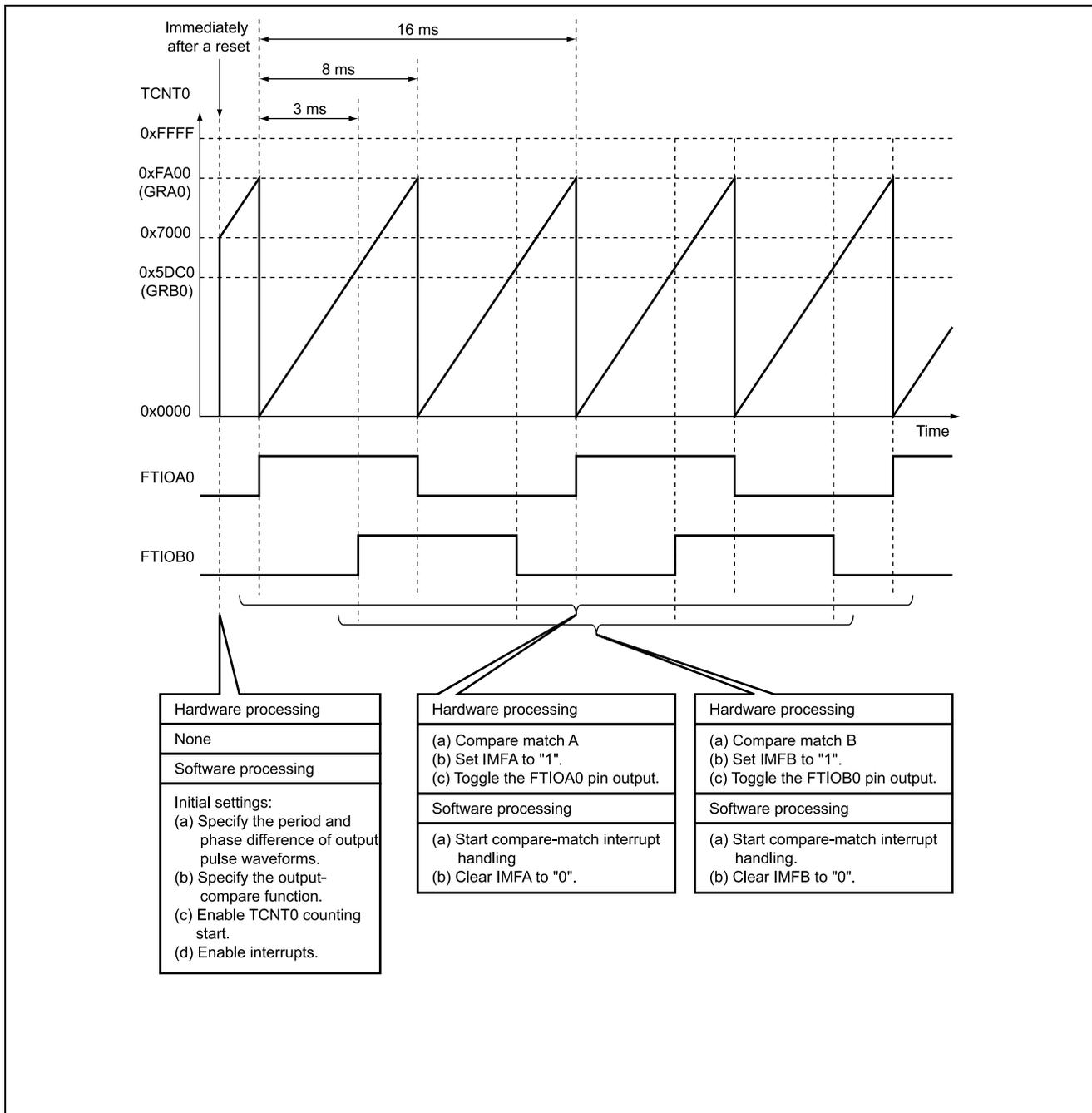
Figure 3.1 Principle of Operation
