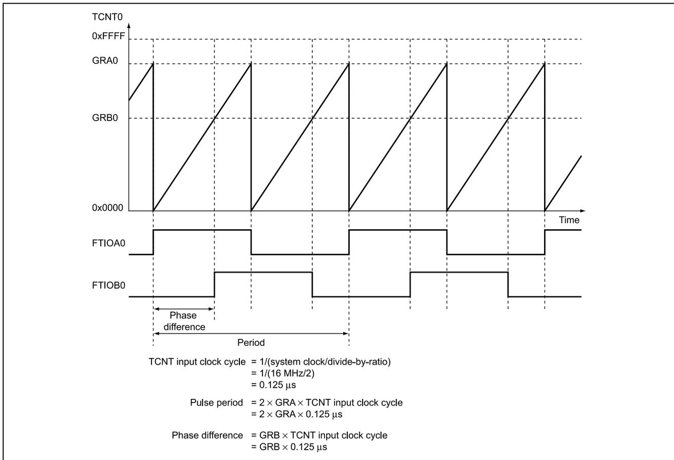
**Figure 2.2 How the Period and Phase Difference of the Output Pulses are Set**
