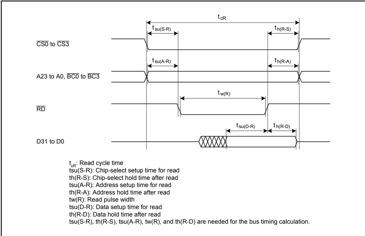
Figure 4.1 Read Cycle of the R32C/100 Series
