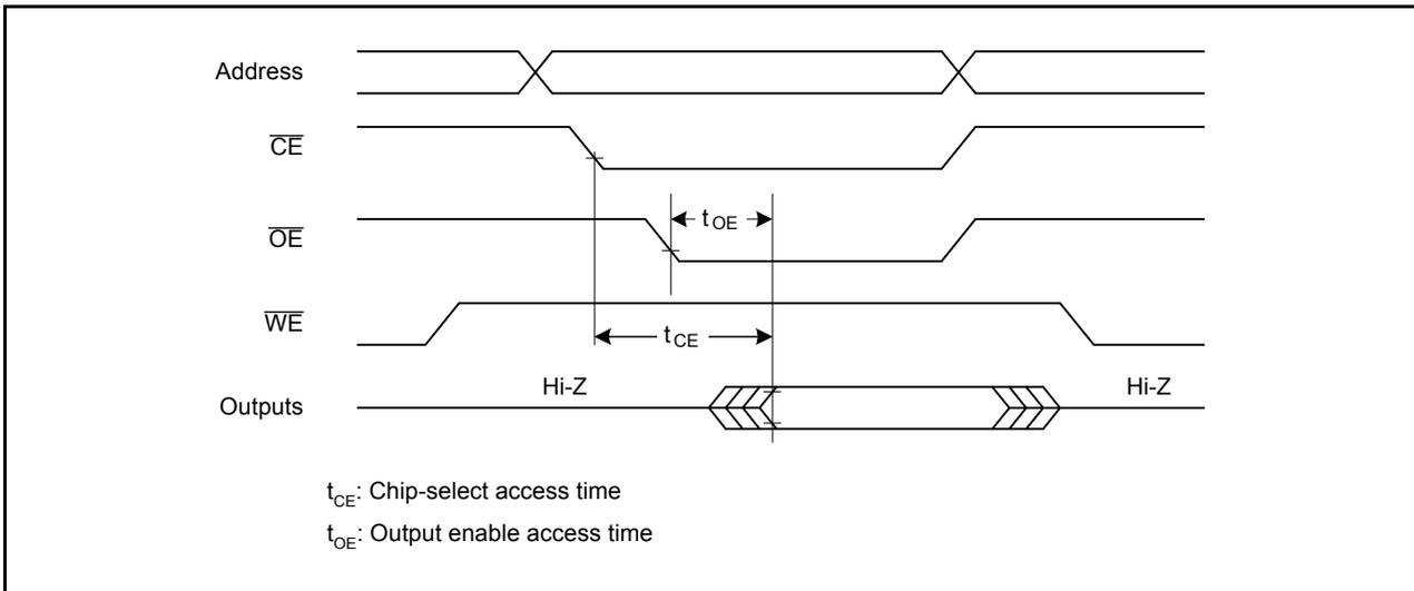
Figure 4.2 Example of External Device Bus Timing When Reading
