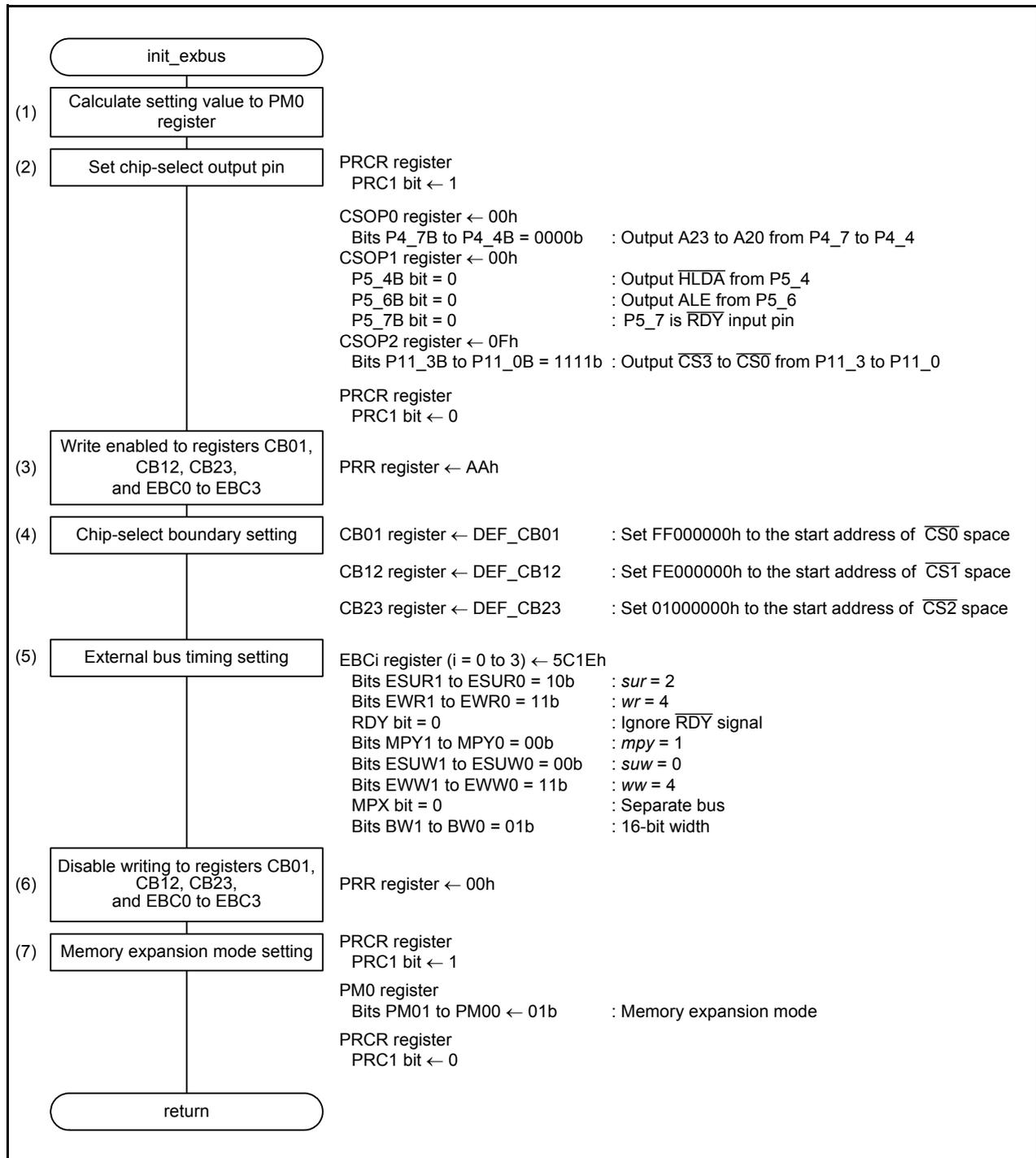
Figure 6.3 External Bus Initial Setting
