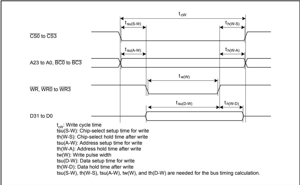
Figure 4.4 R32C/100 Series Write Cycle
