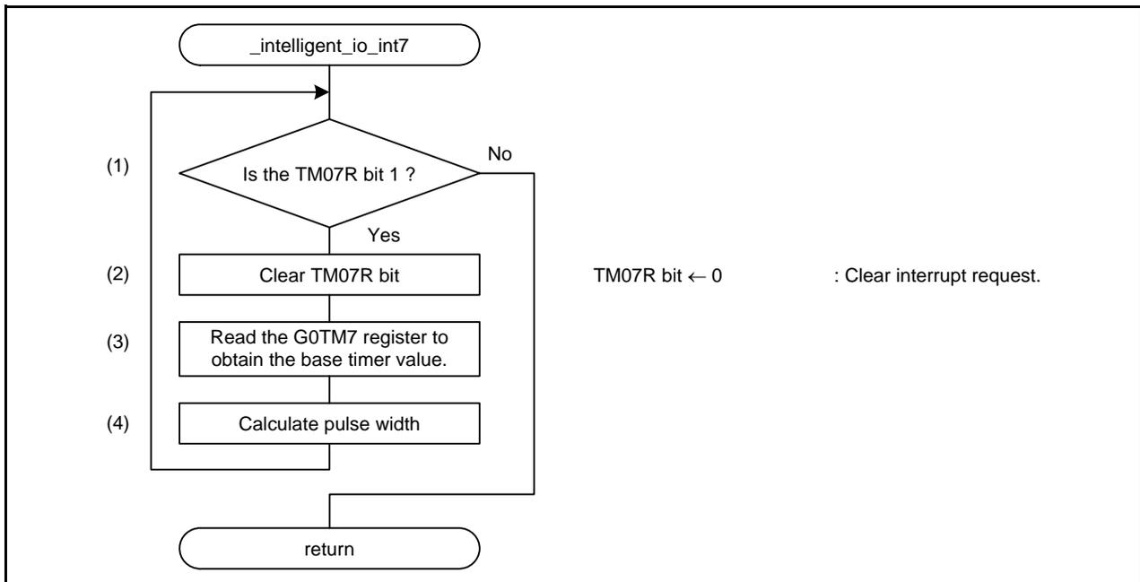
Figure 5.4 Intelligent I/O Interrupt 7 Handling
