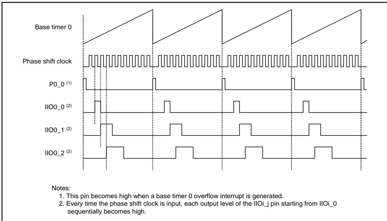
Figure 5.1 Waveform Output Timing Using the Sample Code
