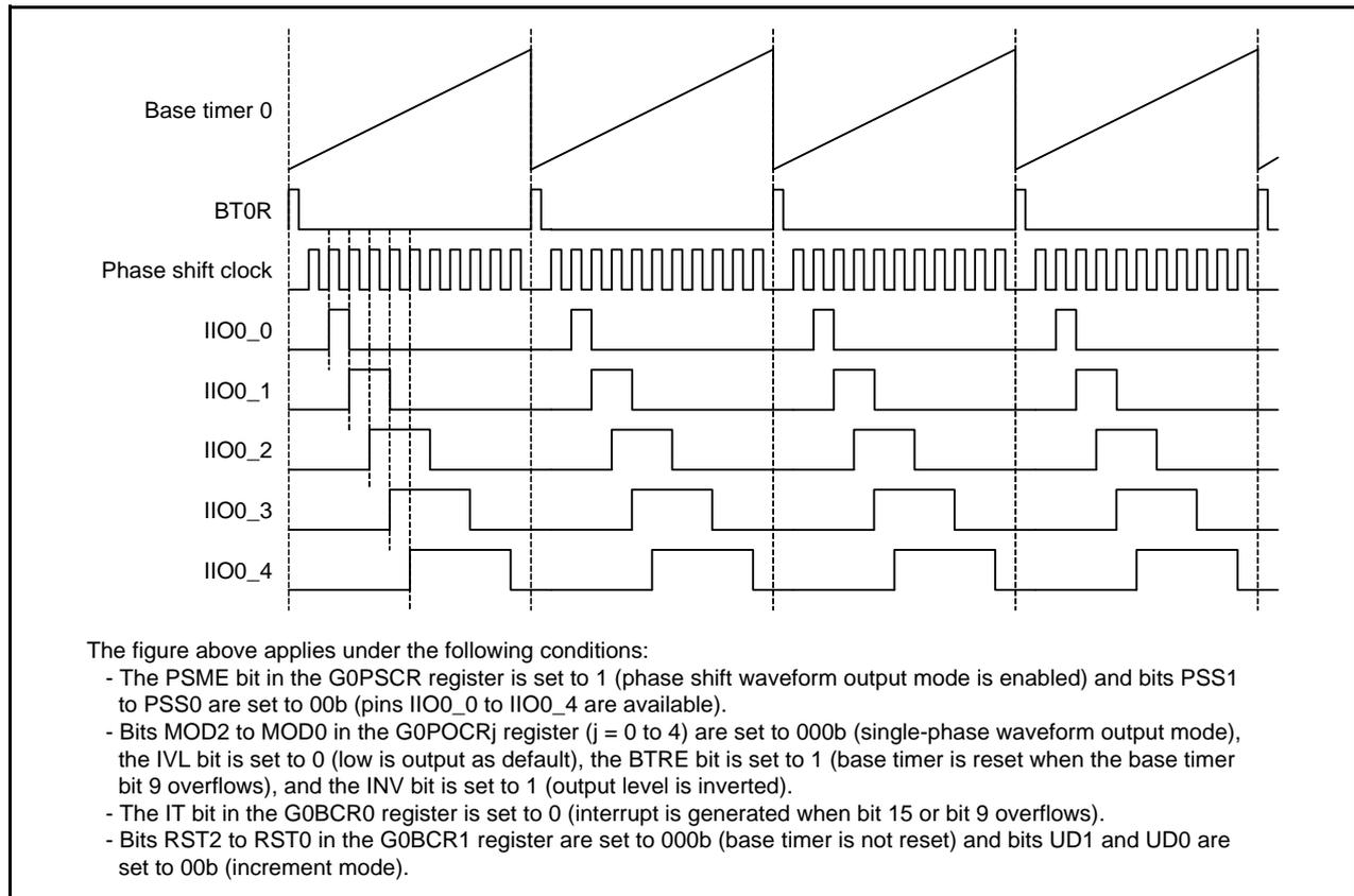
**Figure 1.1 Phase Shift Waveform Output Mode ( $i = 0, 1$ )**
