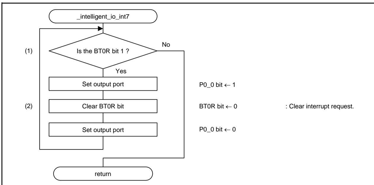
Figure 5.5 Intelligent I/O Interrupt Handling
