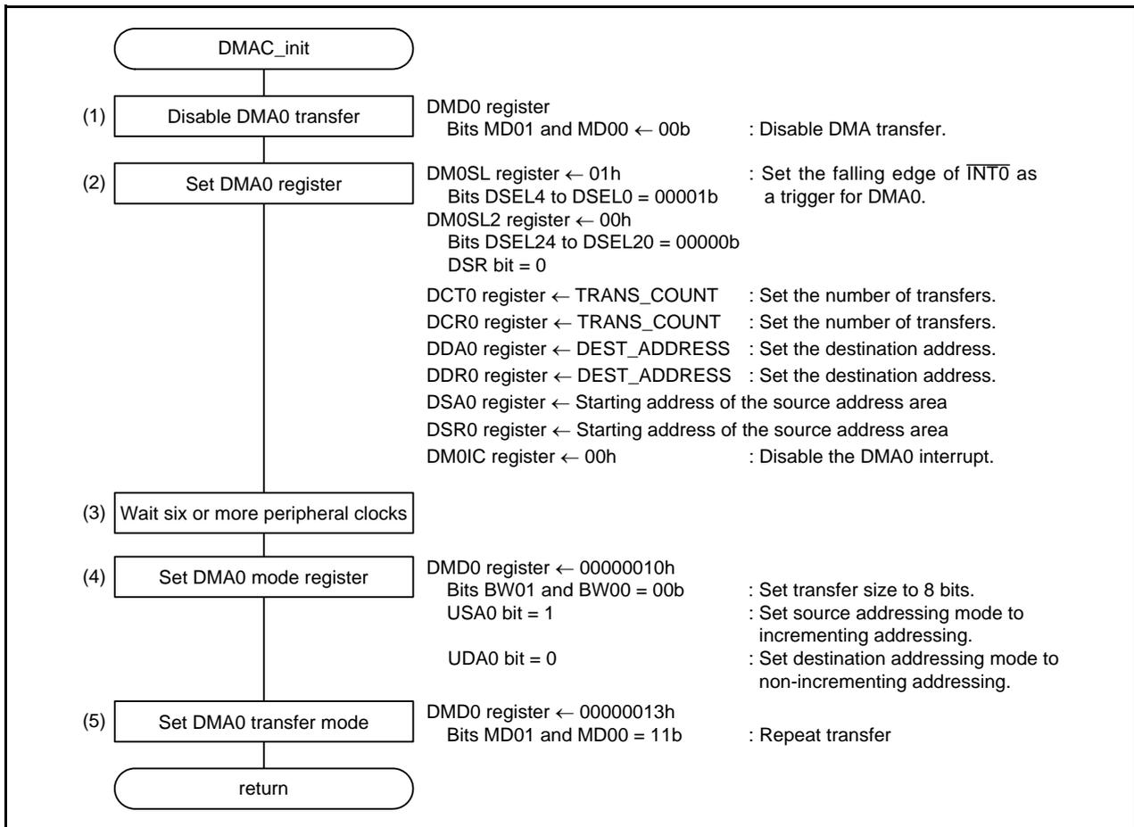
Figure 5.4 DMAC Initial Setting
