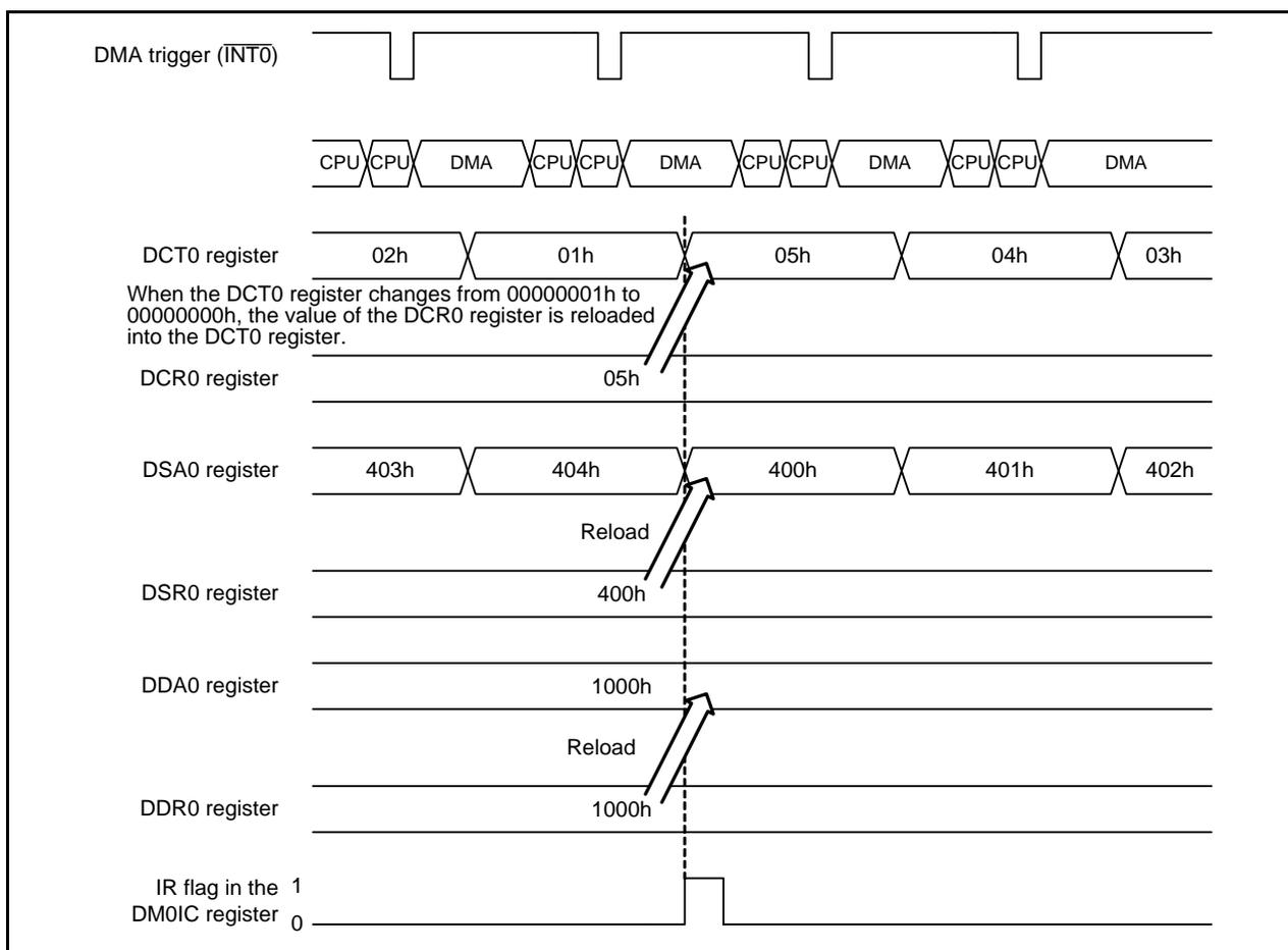
Figure 5.2 Repeat Transfer Timing Example
