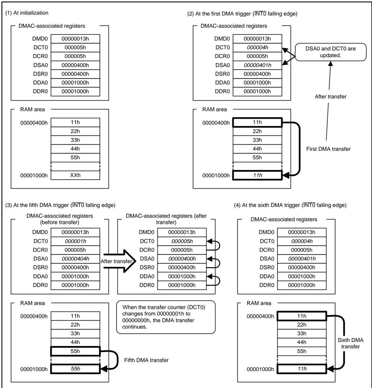
Figure 5.1 DMA Transfer Operation Example
