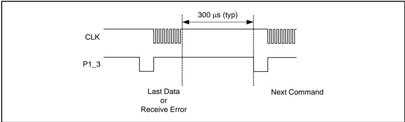
Figure 5.1 Serial Communication Provision
