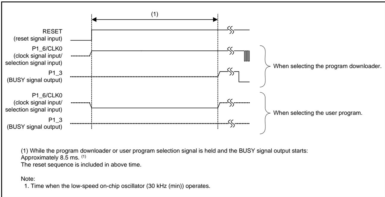
Figure 3.5 Signal Control Timing after Reset
