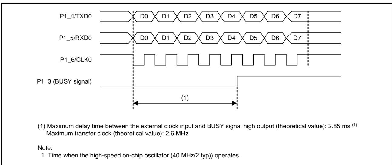
Figure 3.6 Timing between Transfer Clock Input and the BUSY Signal Becoming High
