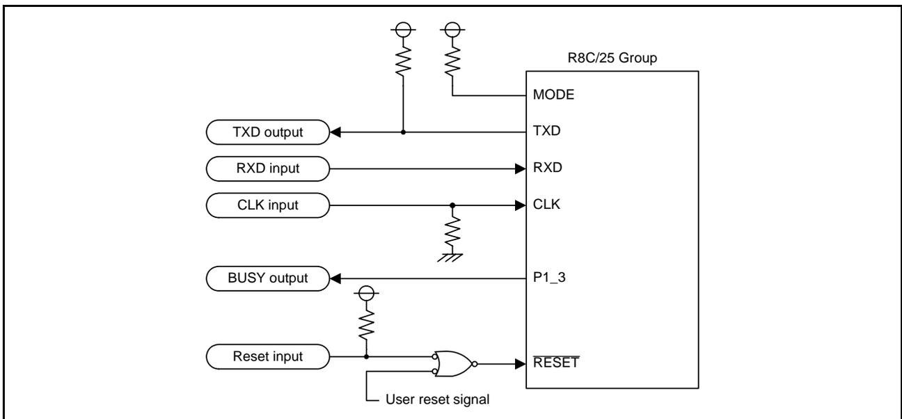
Figure 7.1 Programmer Configuration
