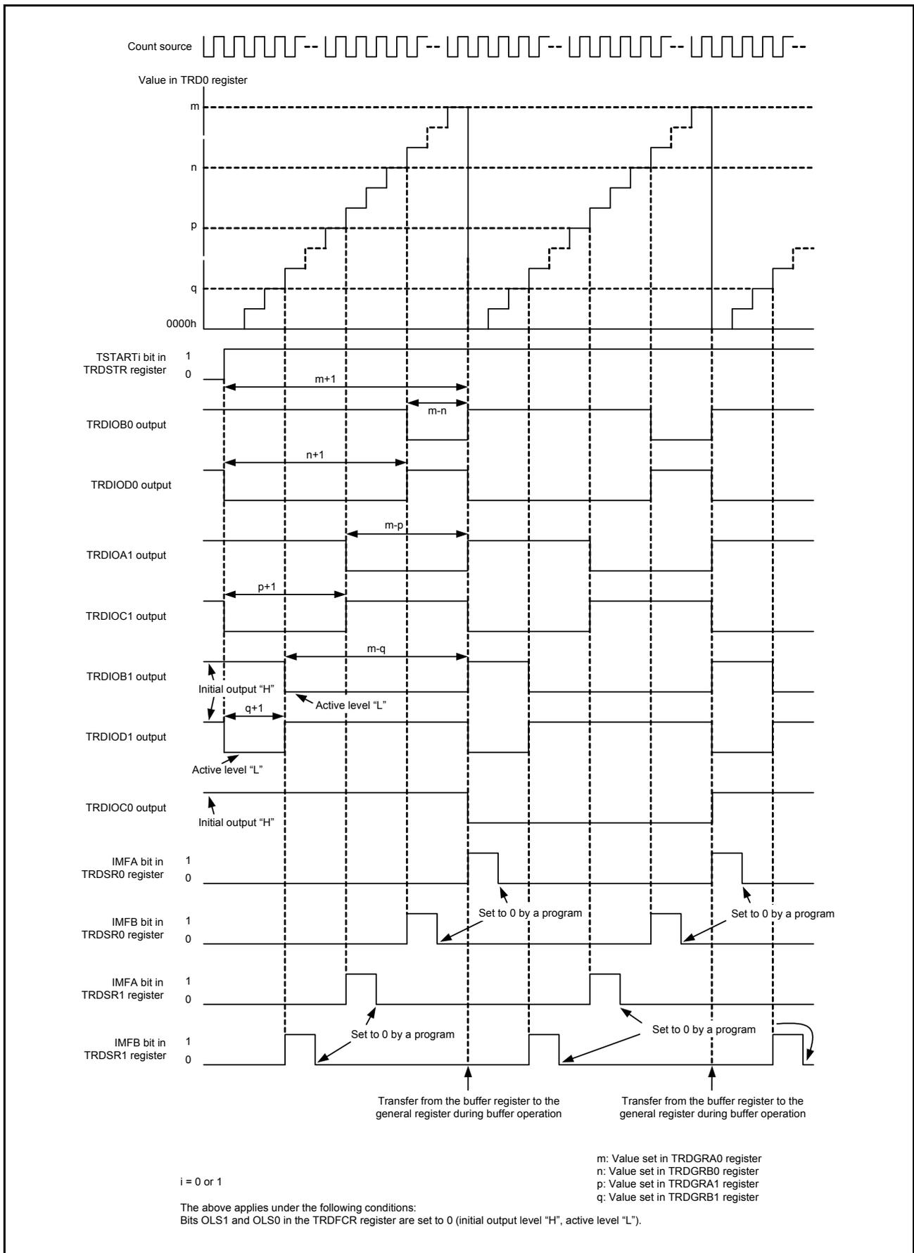
Figure 3.13 Operating Example of Reset Synchronous PWM Mode
