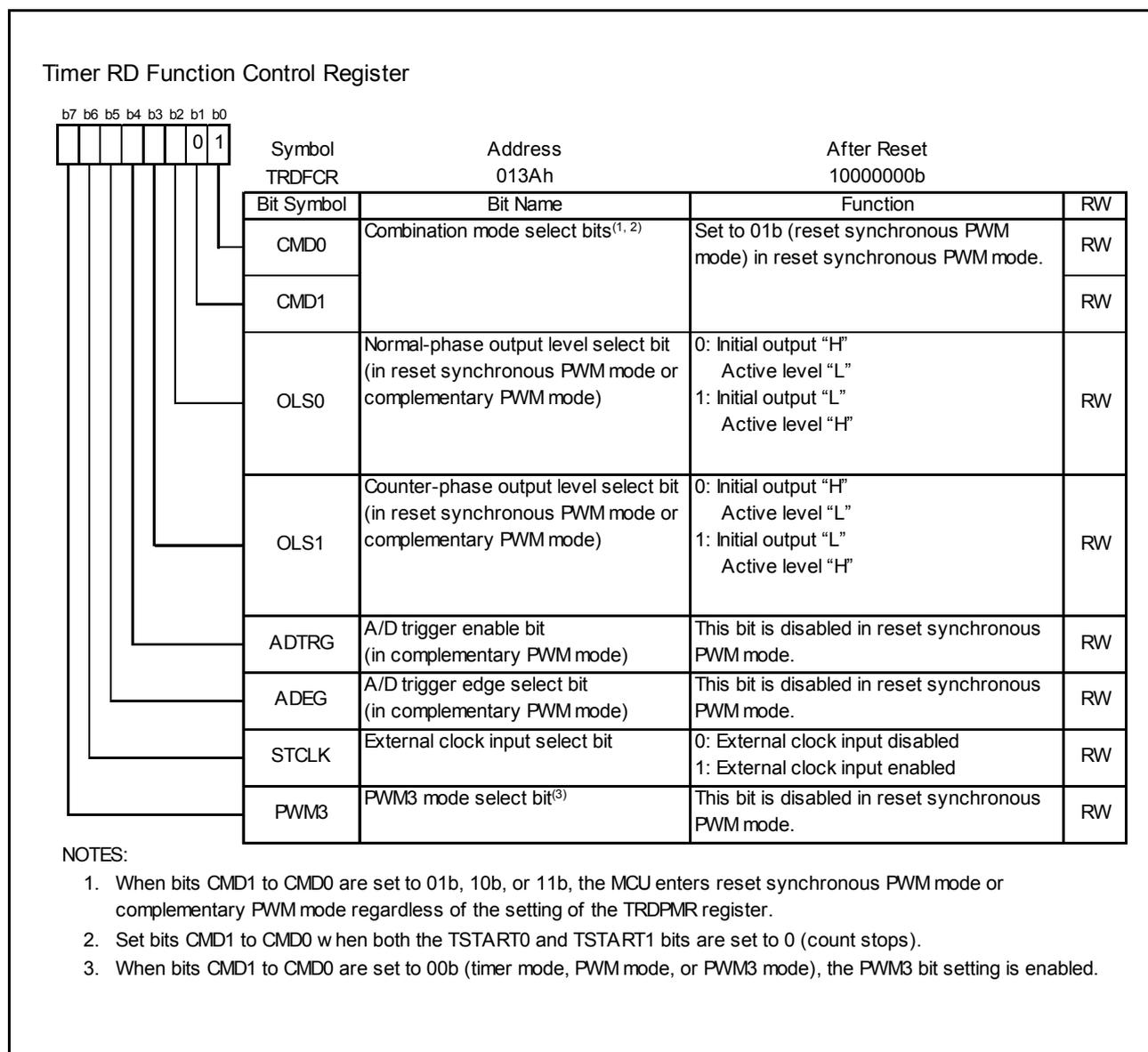
Figure 3.6 TRDFCR Register in Reset Synchronous PWM Mode
