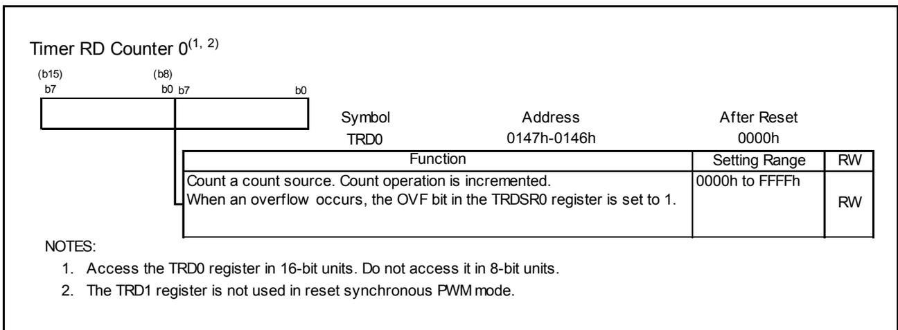
Figure 3.11 TRD0 Register in Reset Synchronous PWM Mode
