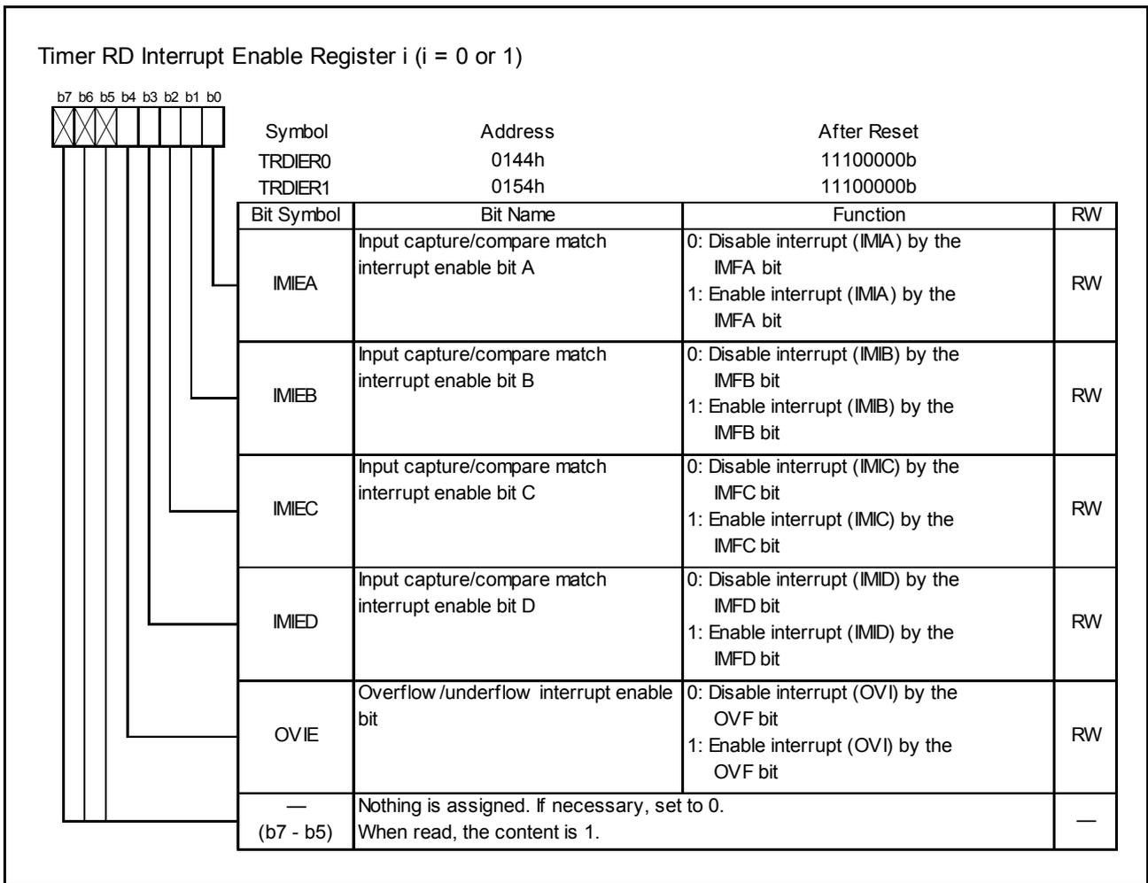
Figure 3.10 Registers TRDIER0 to TRDIER1 in Reset Synchronous PWM Mode
