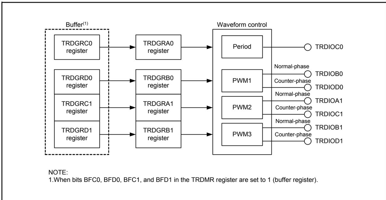
Figure 3.4 Block Diagram of Reset Synchronous PWM Mode
