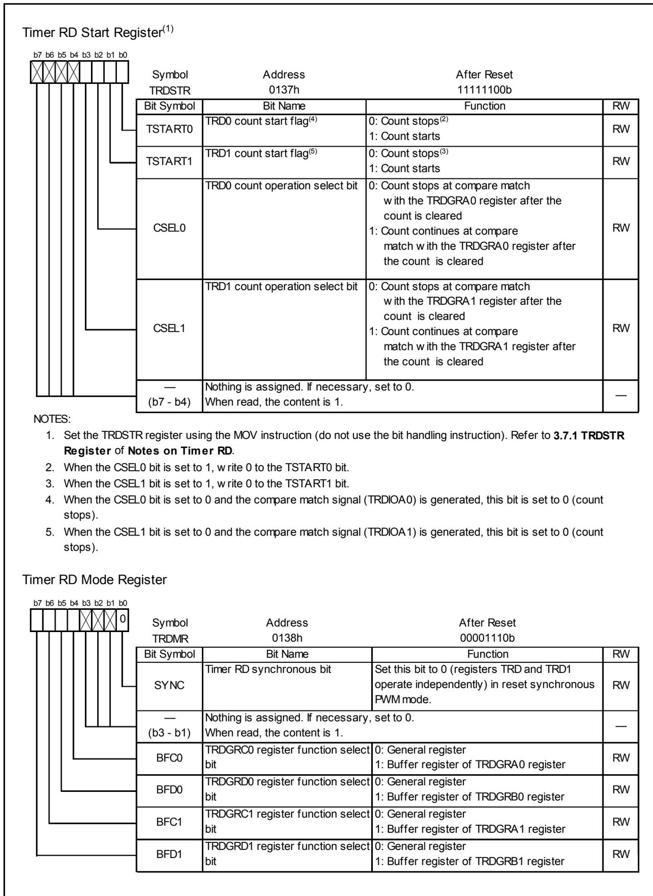
Figure 3.5 Registers TRDSTR and TRDMR in Reset Synchronous PWM Mode
