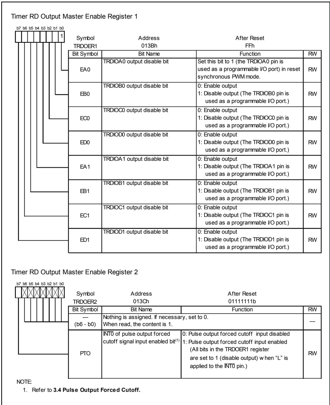
Figure 3.7 Registers TRDOER1 to TRDOER2 in Reset Synchronous PWM Mode
