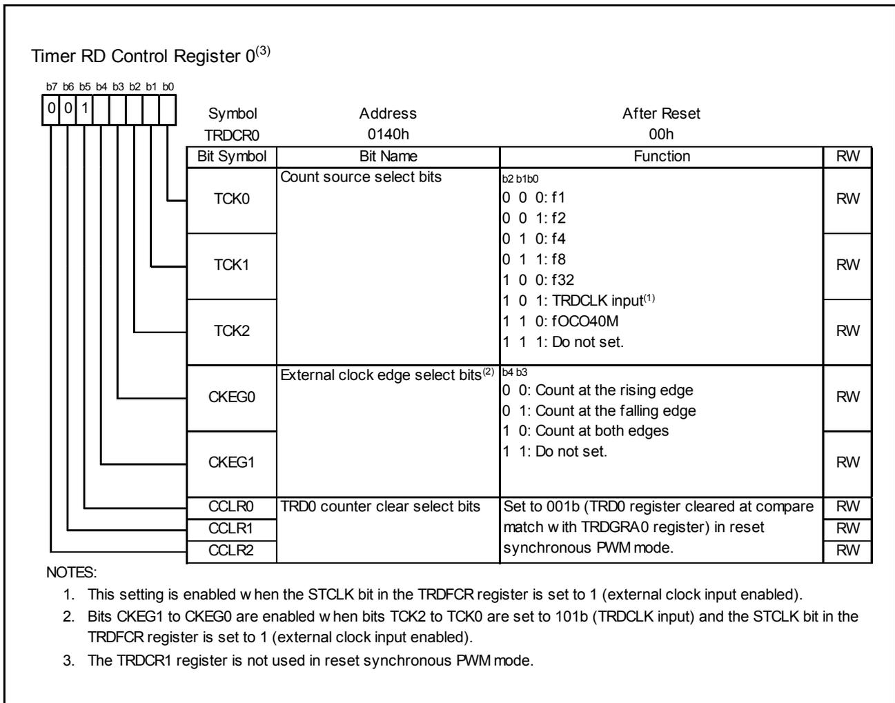
Figure 3.8 TRDCR0 Register in Reset Synchronous PWM Mode
