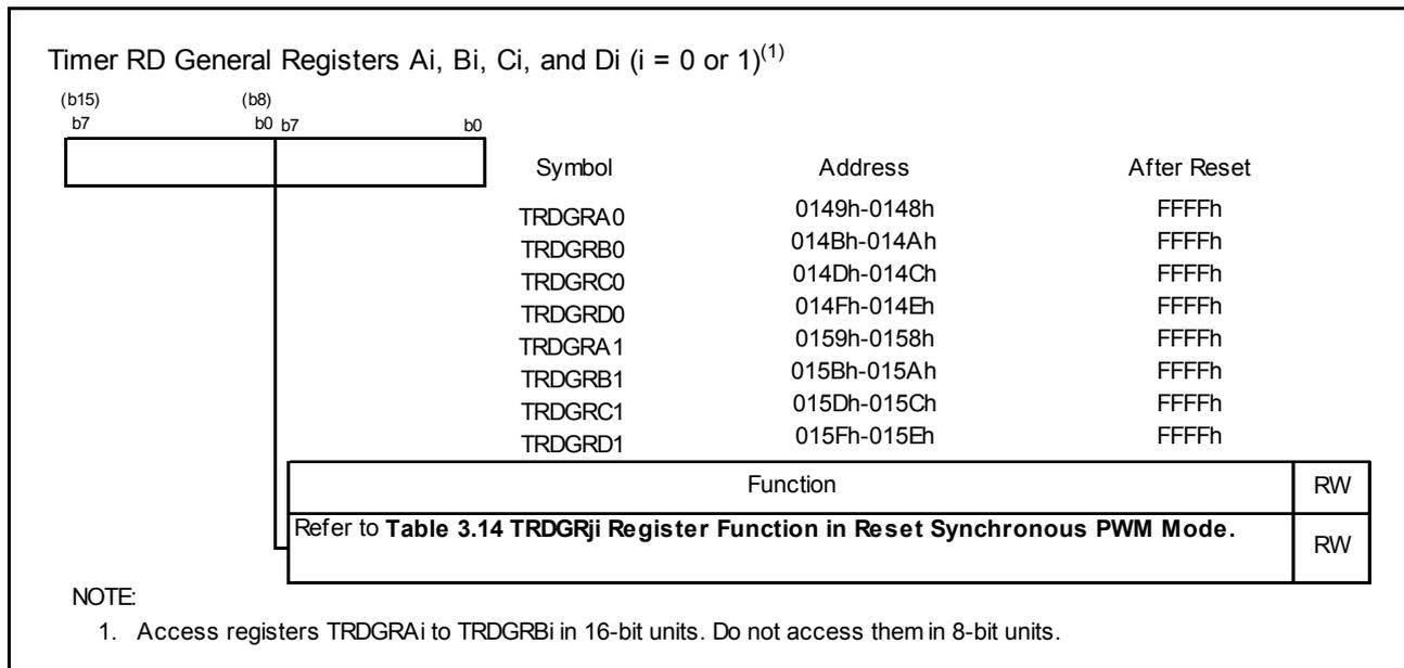
Figure 3.12 Registers TRDGRAi, TRDGRBi, TRDGRCi, and TRDGRDi in Reset Synchronous PWM Mode
