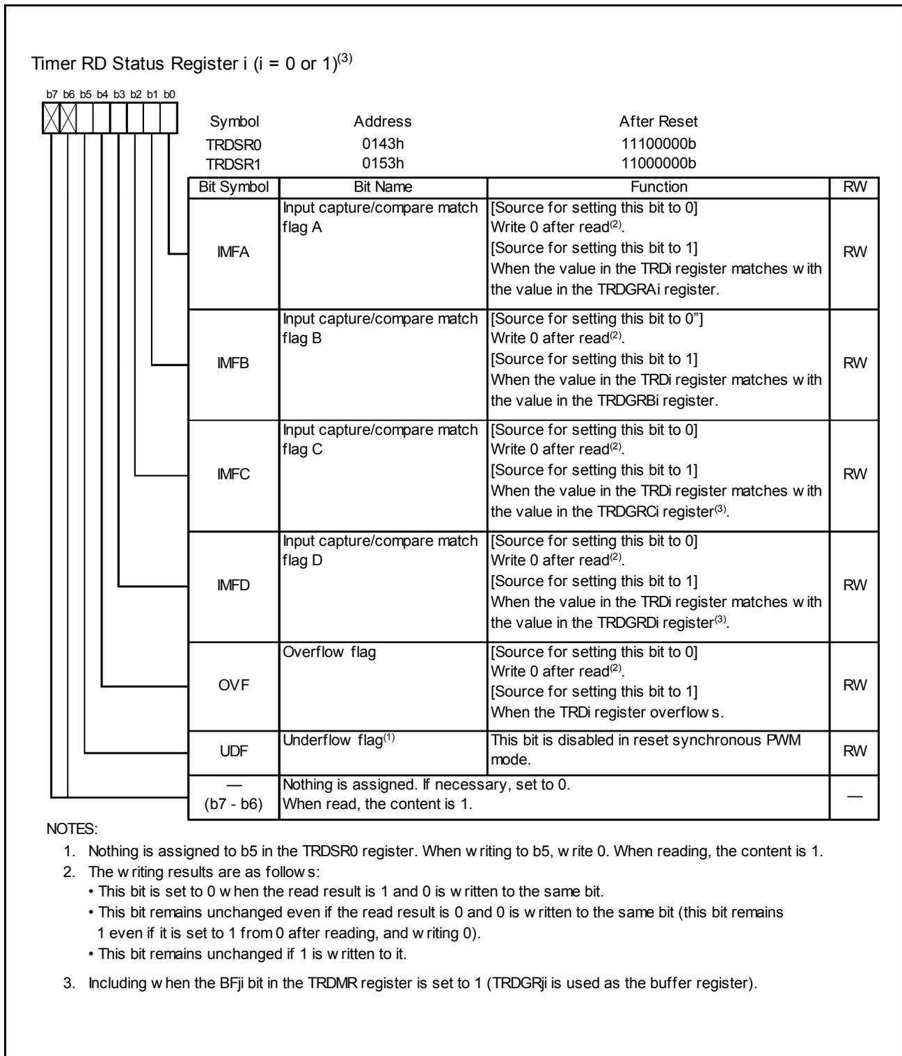
Figure 3.9 Registers TRDSR0 to TRDSR1 in Reset Synchronous PWM Mode
