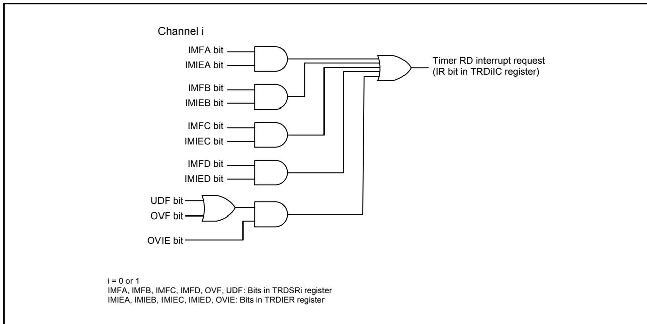
Figure 3.14 Block Diagram of Timer RD Interrupt
