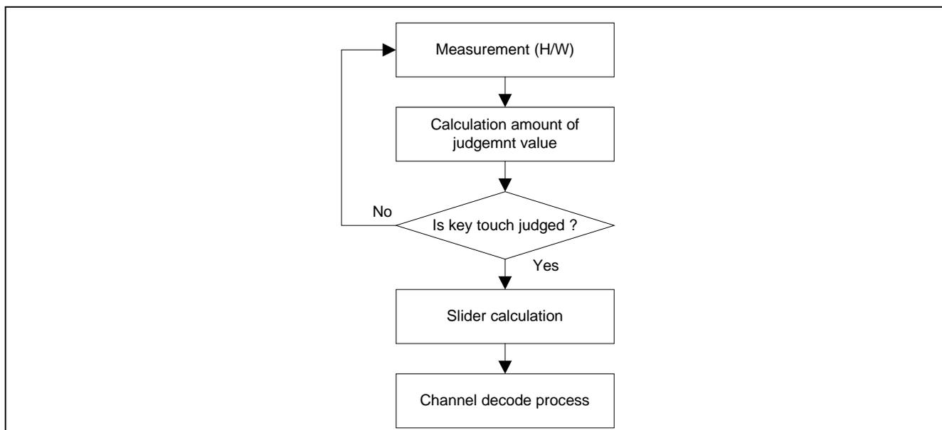
Figure 2-1 The flowchart of slider process
