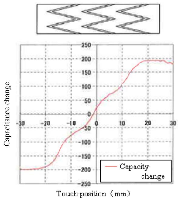
Figure 1-8 Electrodes with double 'V' shape
