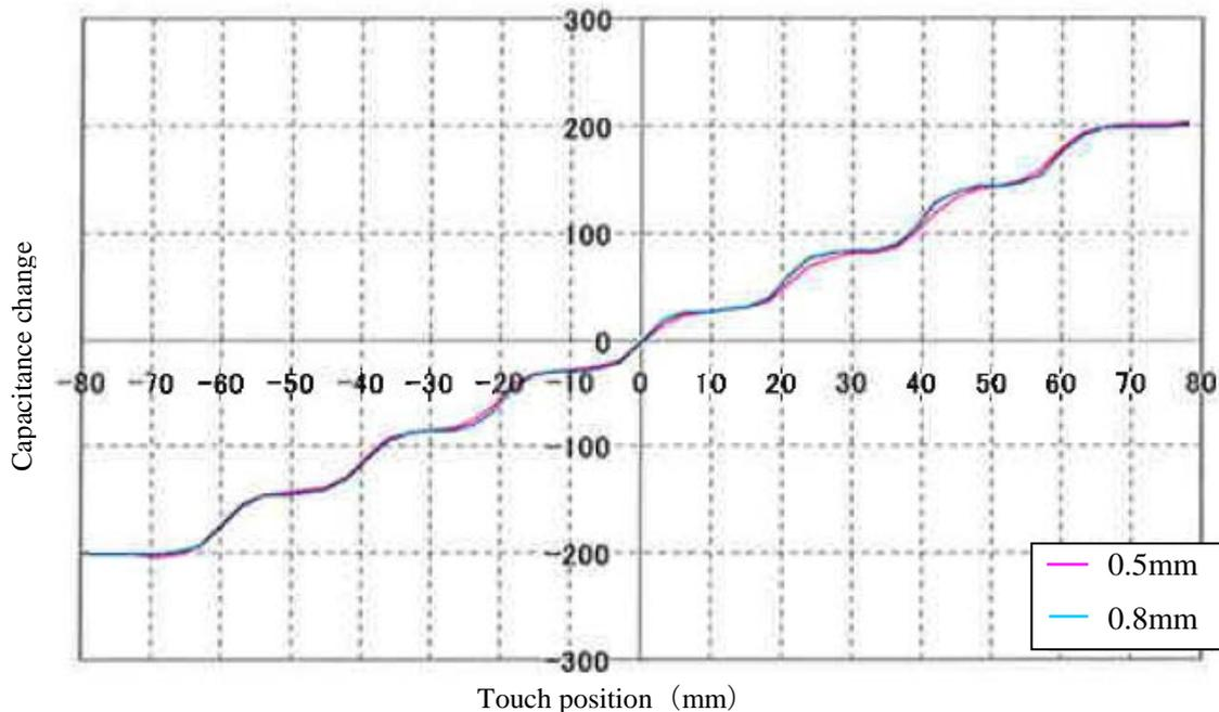
Figure 1-17 0.5mm,0.8mm gap characteristic
