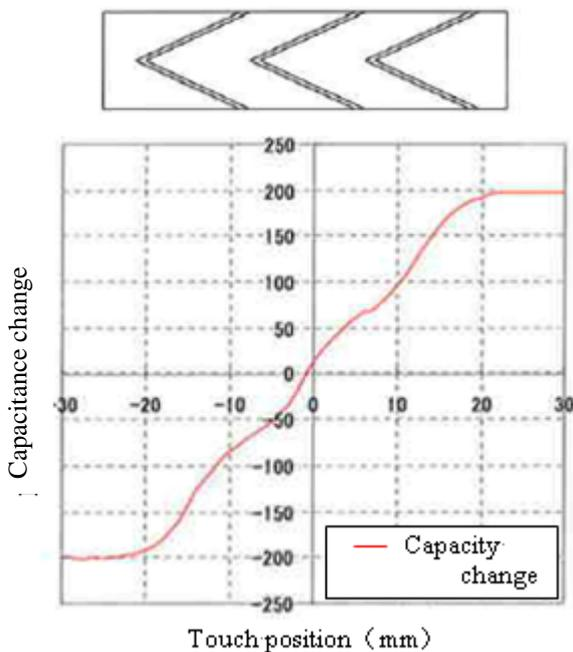
Figure 1-7 Electrodes with single 'V' shape
