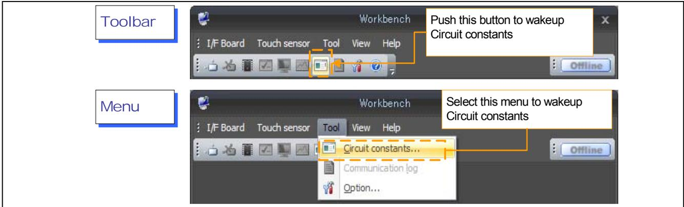
Figure 7-4 Circuit constants starting
