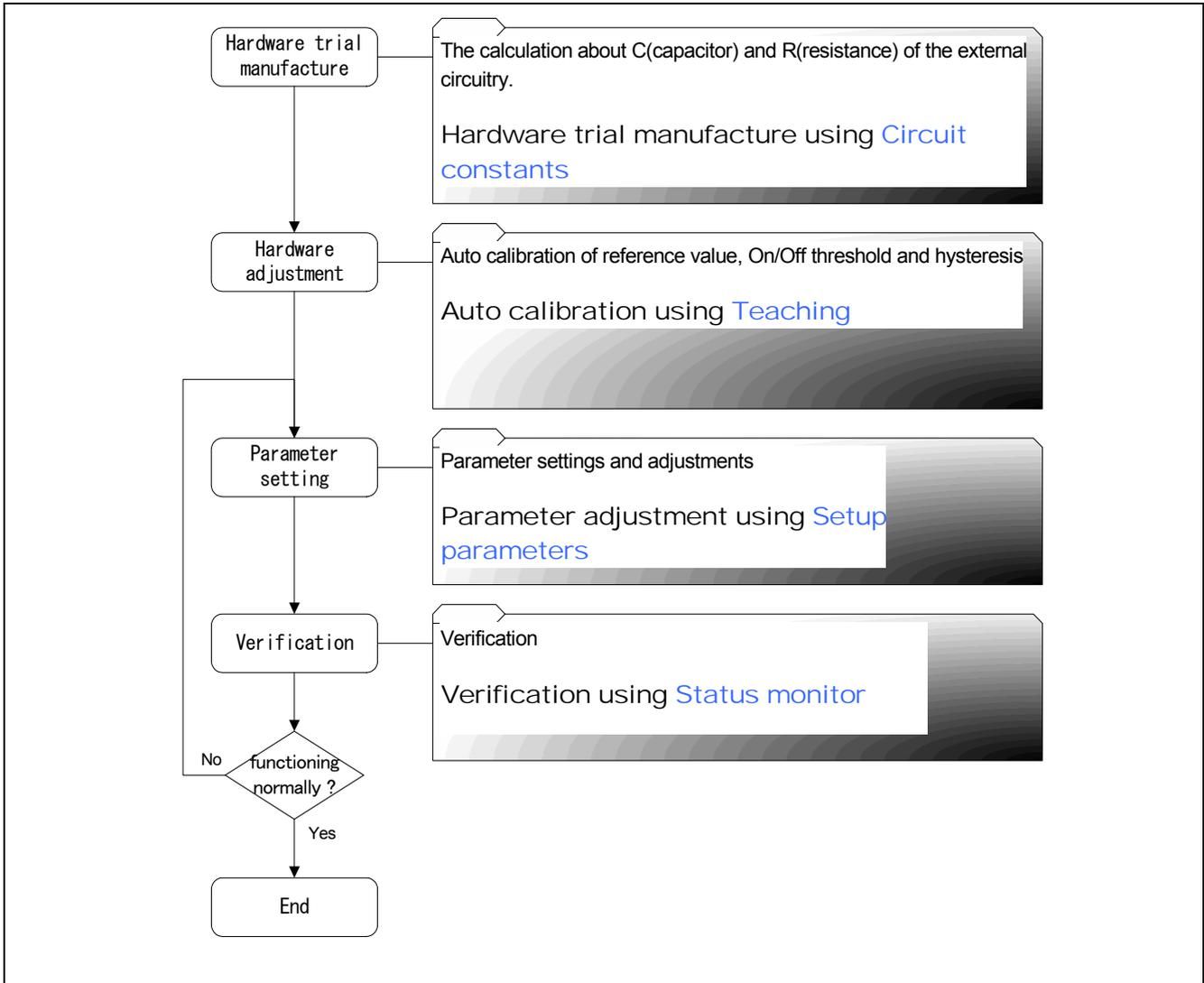
Figure 7-1 Adjustment flow chart
