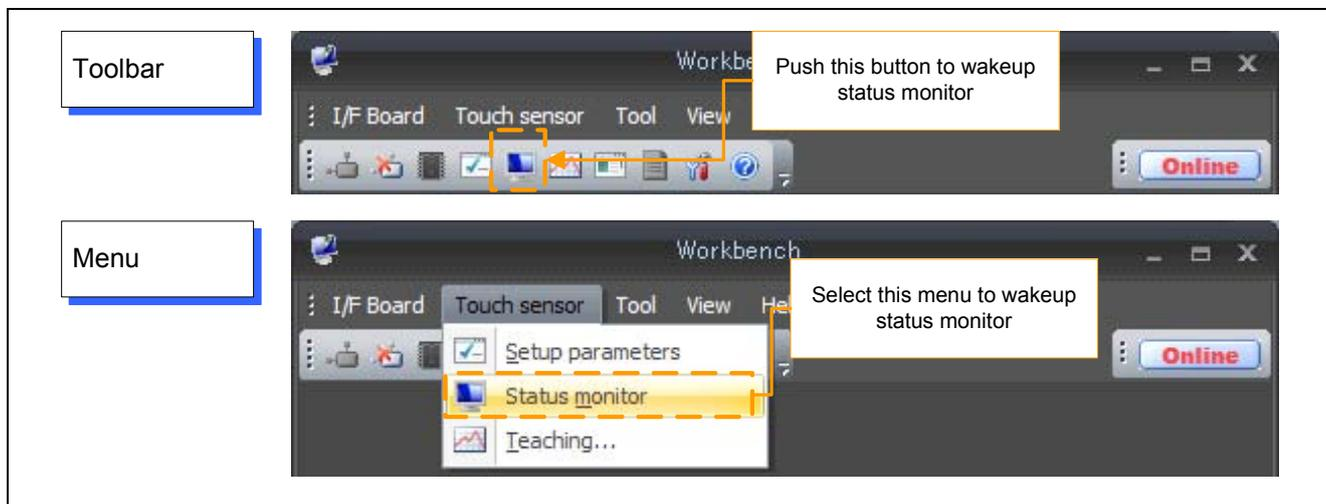
Figure 3-11 the method of starting “Status monitor”
