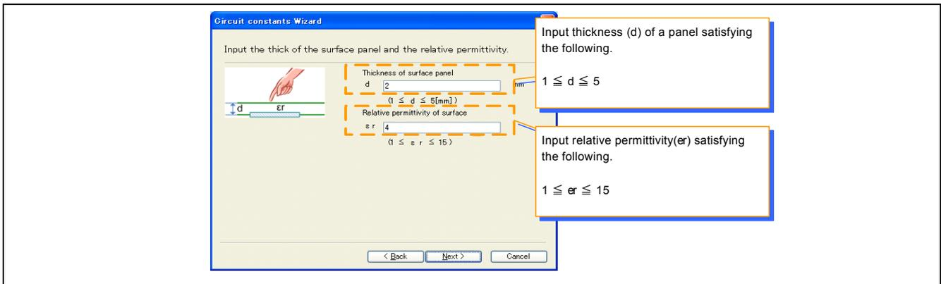
**Figure 7-8 Thickness and Relative permittivity of the panel settings**
