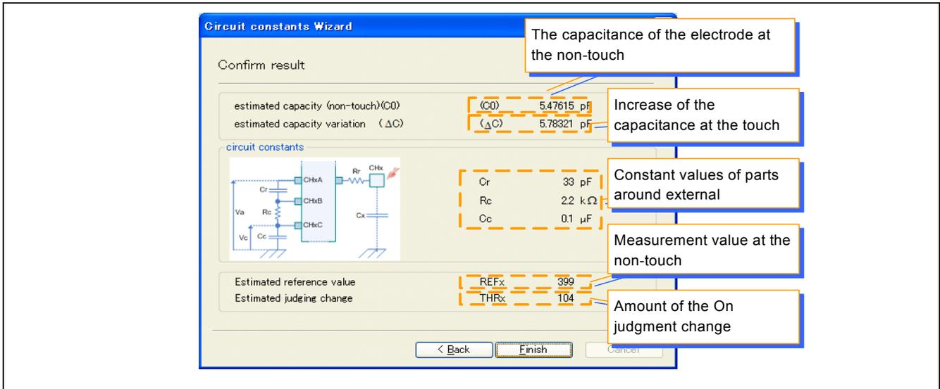
Figure 7-11 Result of calculation
