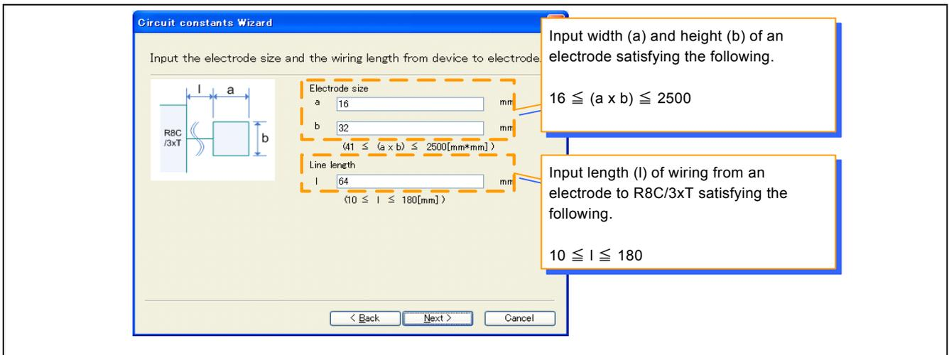
Figure 7-6 Width and Height of the electrode, wiring length settings
