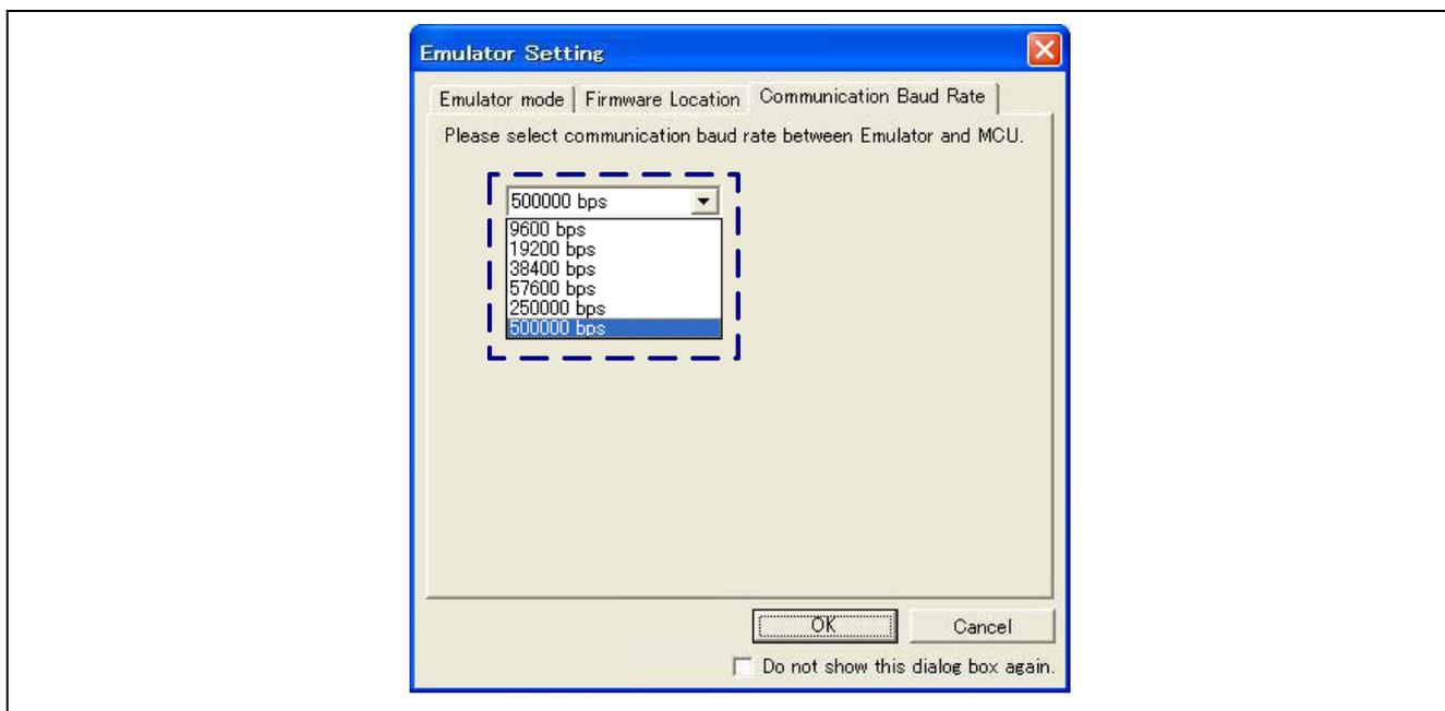
Figure 3-7 Emulator communication baud rate setting
