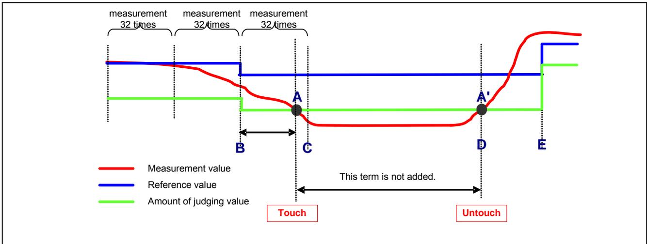
Figure 7-26 The timing of drift correction
