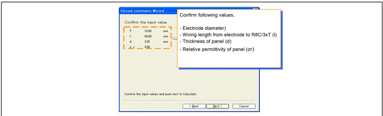
Figure 7-10 Confirmation of the input value (Electrode type is circle)
