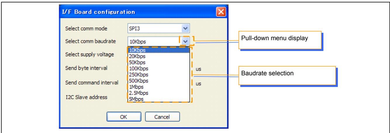
Figure 4-7 Communication baudrate(for SPI3/SPI4) selection
