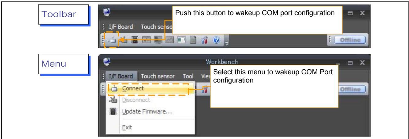
Figure 2-3 the method of starting COM Port configuration
