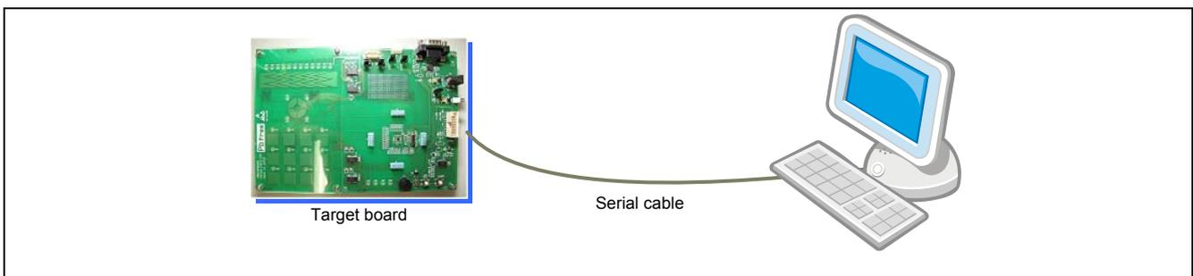
Figure 2-1 Connection between a target board and a PC using a serial cable
