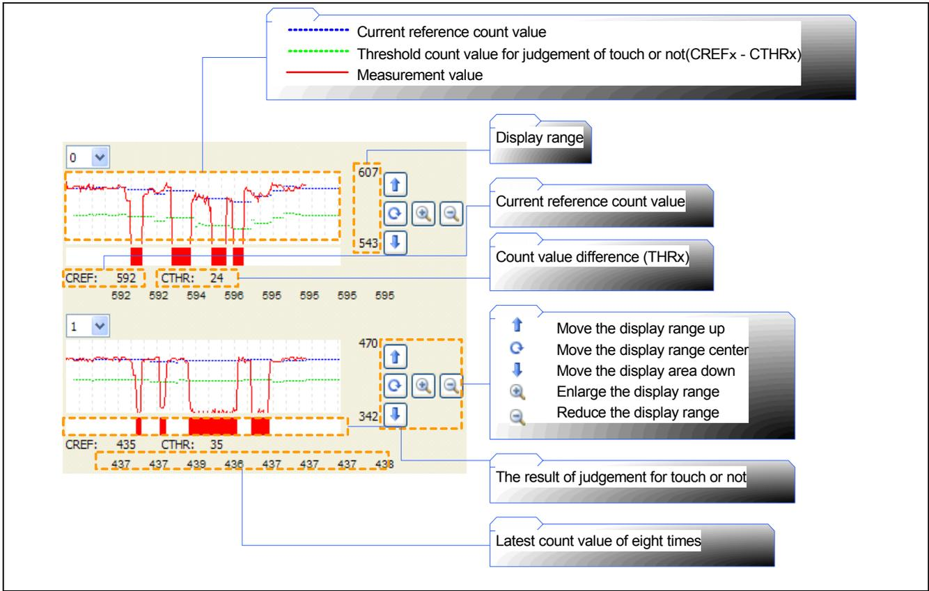
Figure 7-31 Detail explanation of graph display
