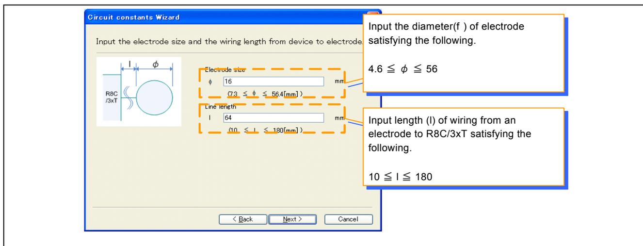
Figure 7-7 Diameter of the electrode, wiring length settings
