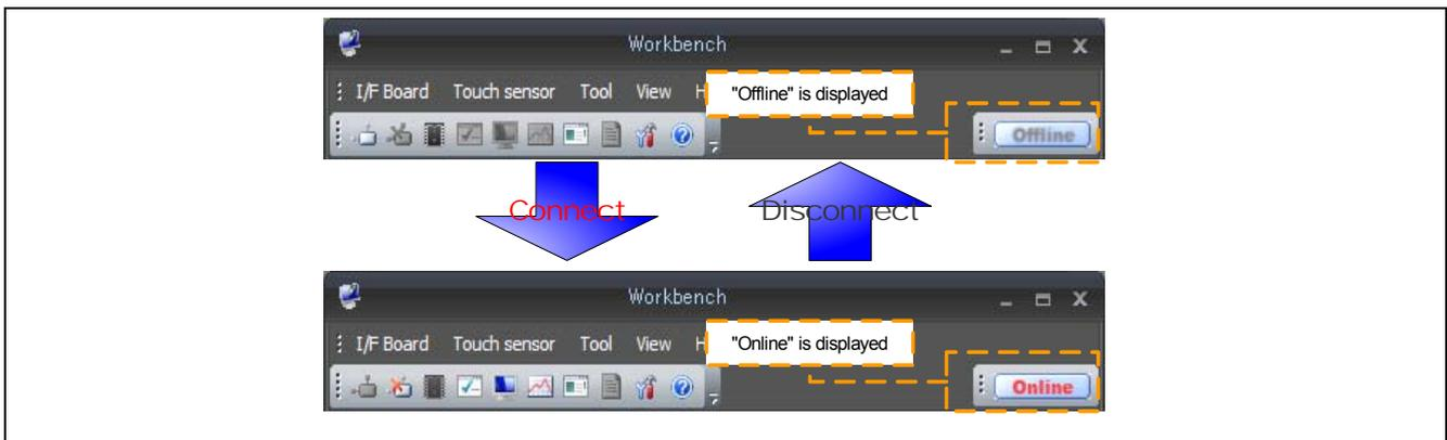
**Figure 4-12 The status of connection with target board**
