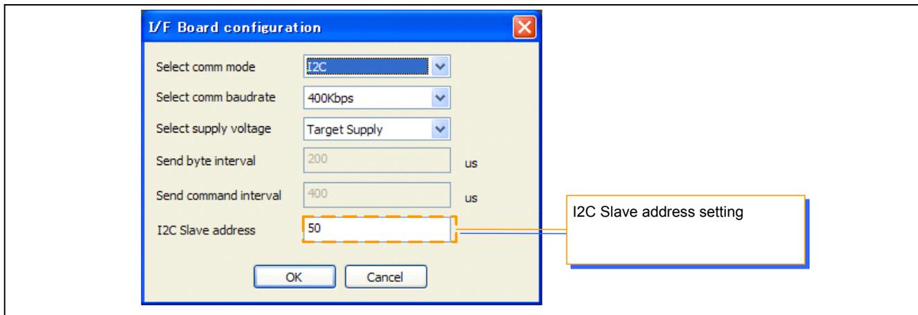
Figure 4-11 I2C Slave address setting
