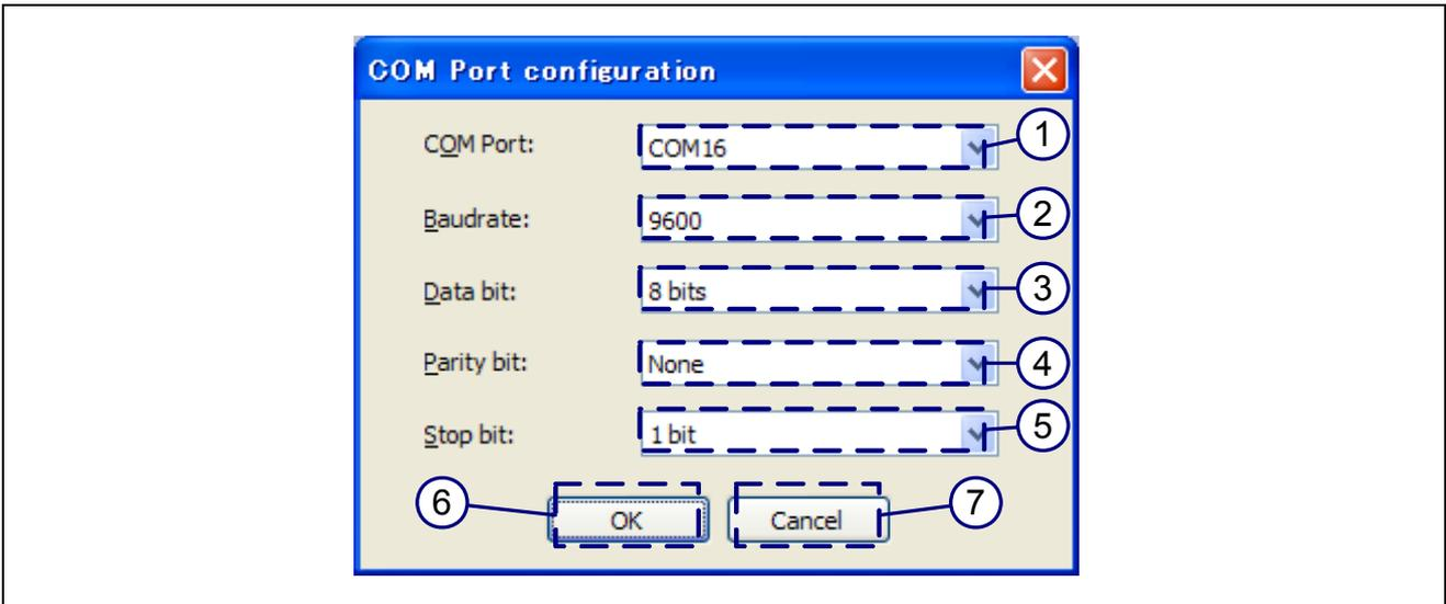
Figure 6-1 COM Port configuration
