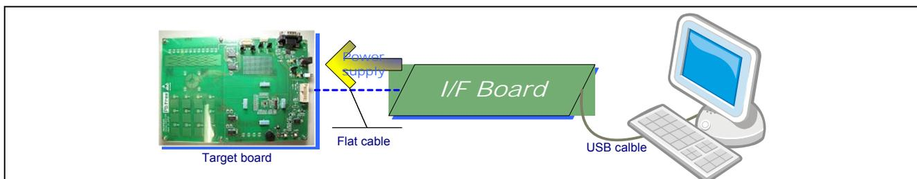
Figure 4-3 The example of power supply from the USB port
