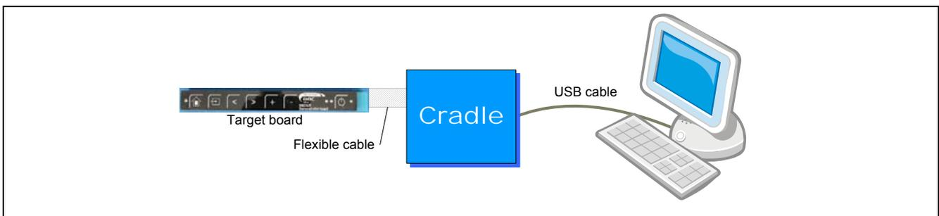
Figure 2-2 Connection between a target board and a PC using the Cradle board
