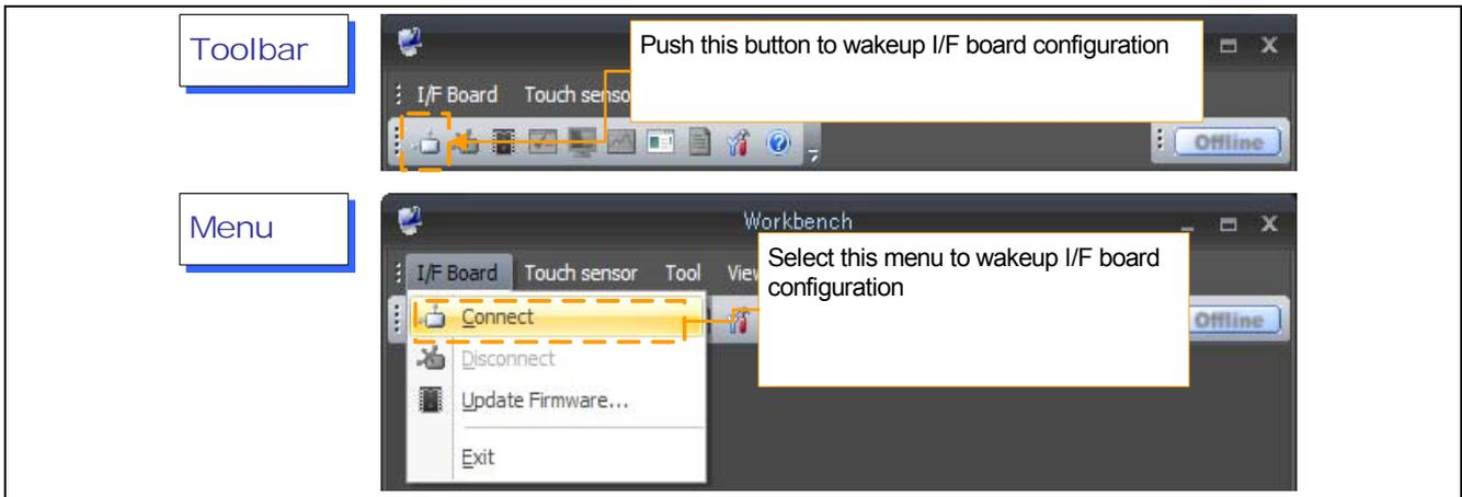
Figure 4-5 The method of starting I/F Board configuration
