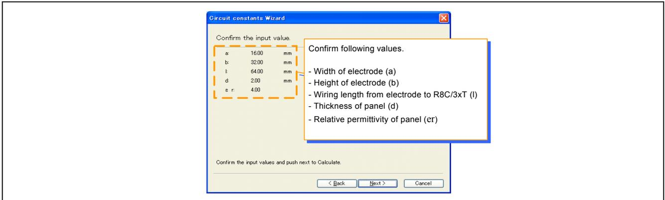
Figure 7-9 Confirmation of the input value (Electrode type is rectangle)
