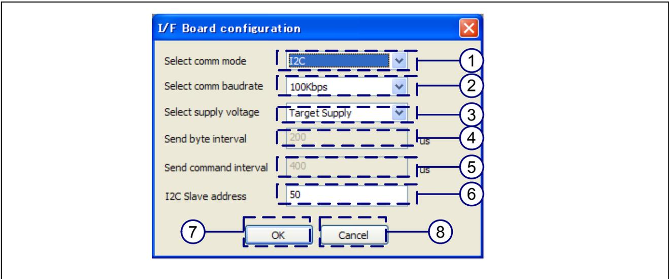
Figure 6-2 I/F Board configuration
