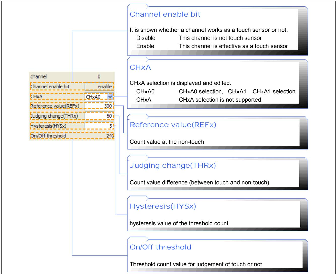
Figure 7-28 Parameters for each channels
