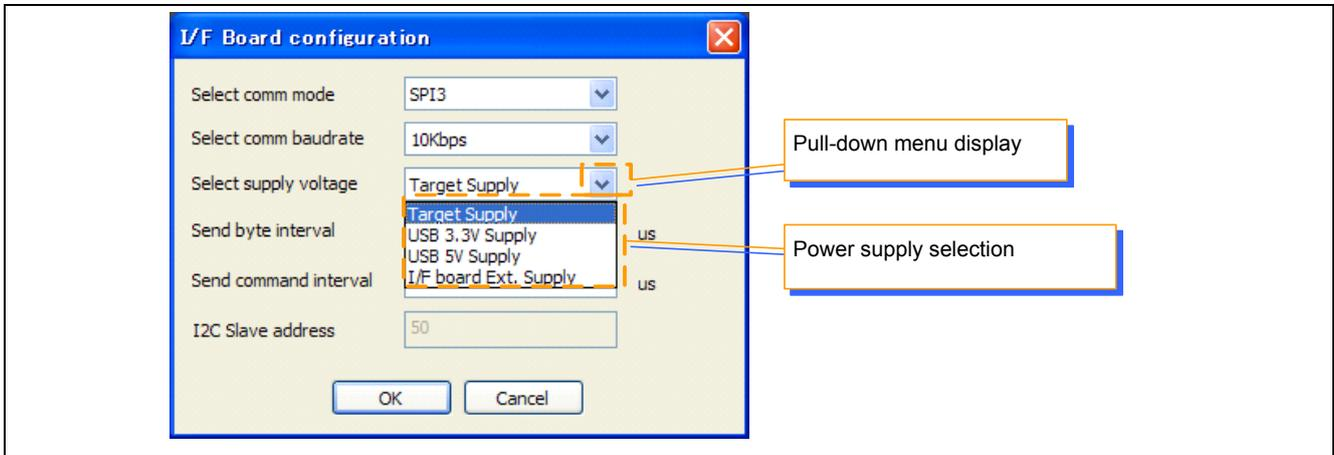
Figure 4-9 The method of supply power selection
