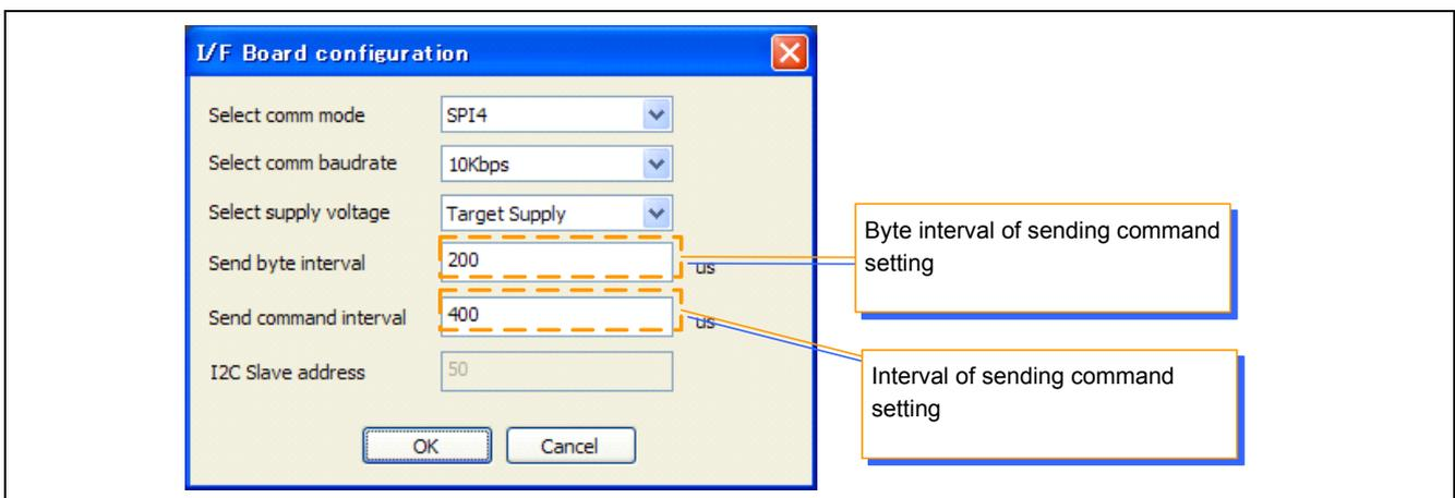
Figure 4-10 Communication timing setting
