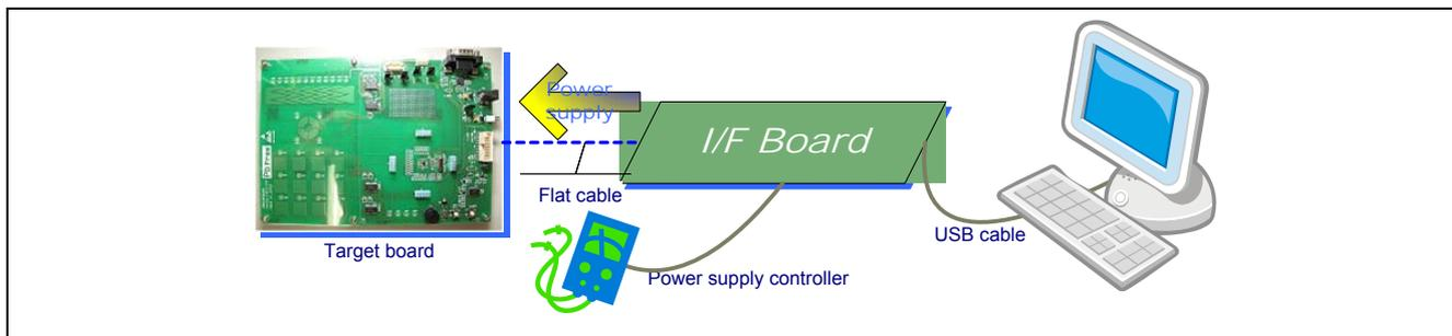
**Figure 4-4 The example which supplies a power from Power supply controller**
