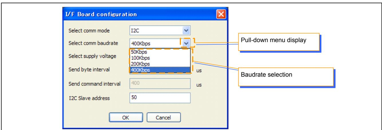
Figure 4-8 Communication baudrate(for I2C) selection
