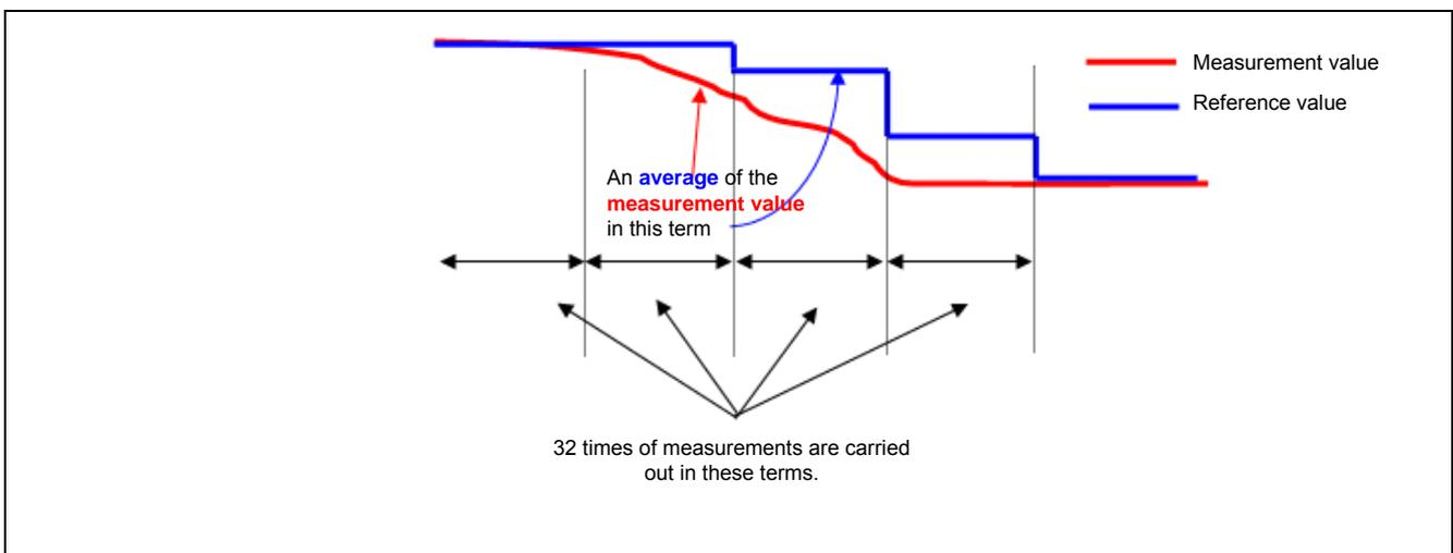
Figure 7-25 Drift correction for the reference count value
