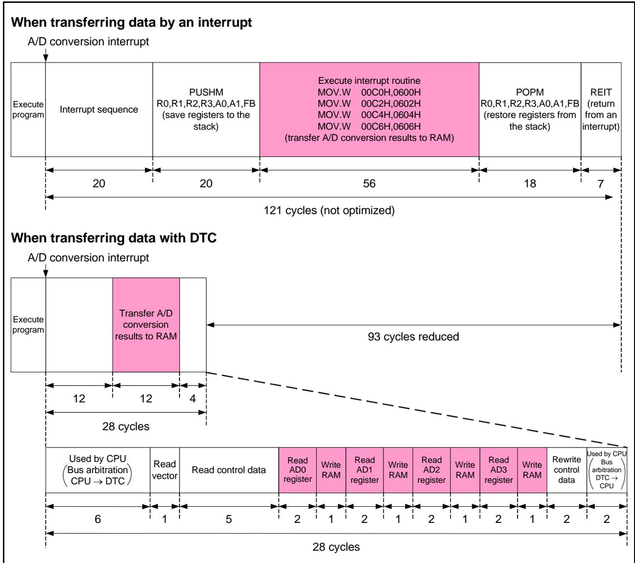
Figure 3.2 Numbers of Data Transfer Cycles
