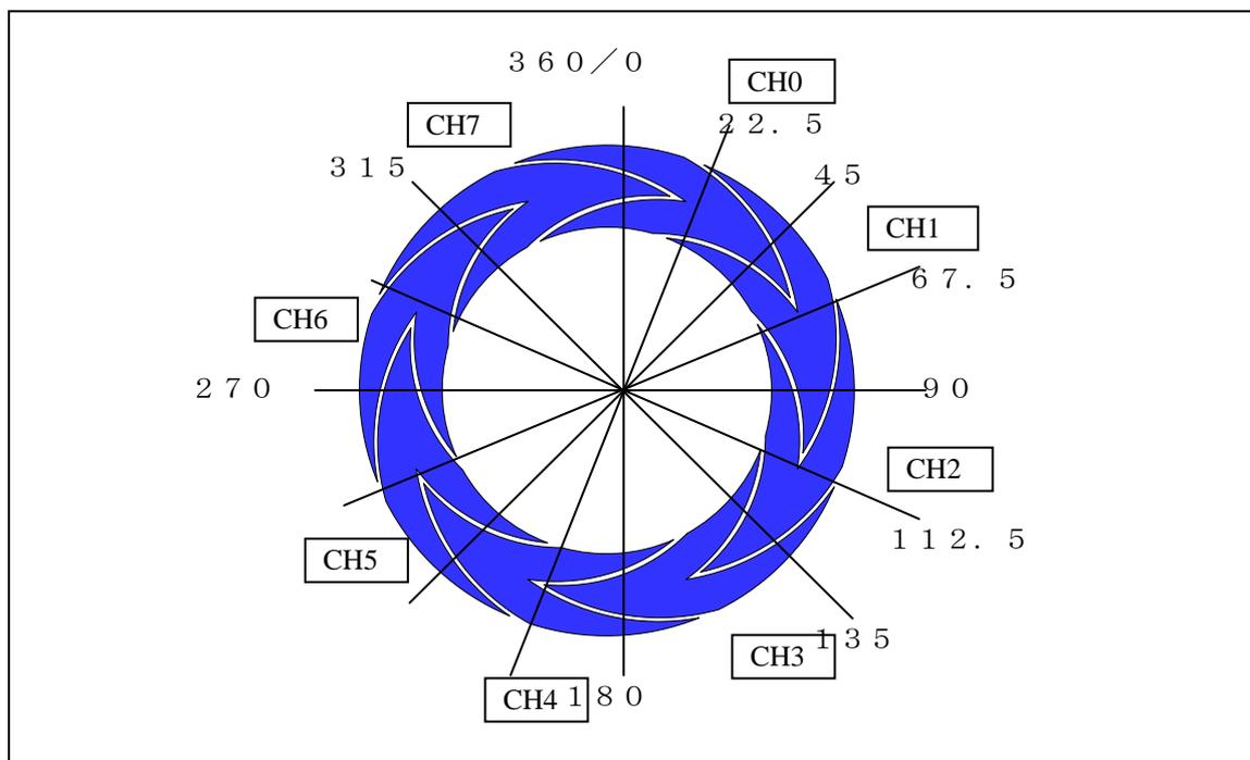
Figure 3-1- 1 Eight electrode wheel operation explanation chart
