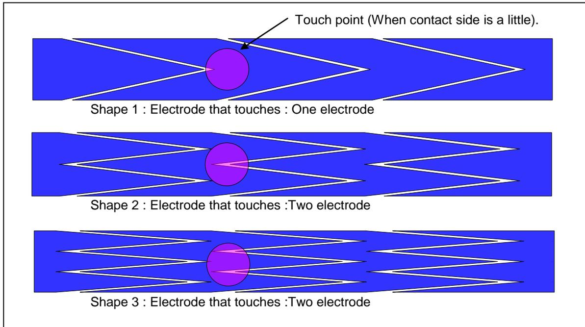
Figure 1-3- 3 Touch area and electrode geometry
