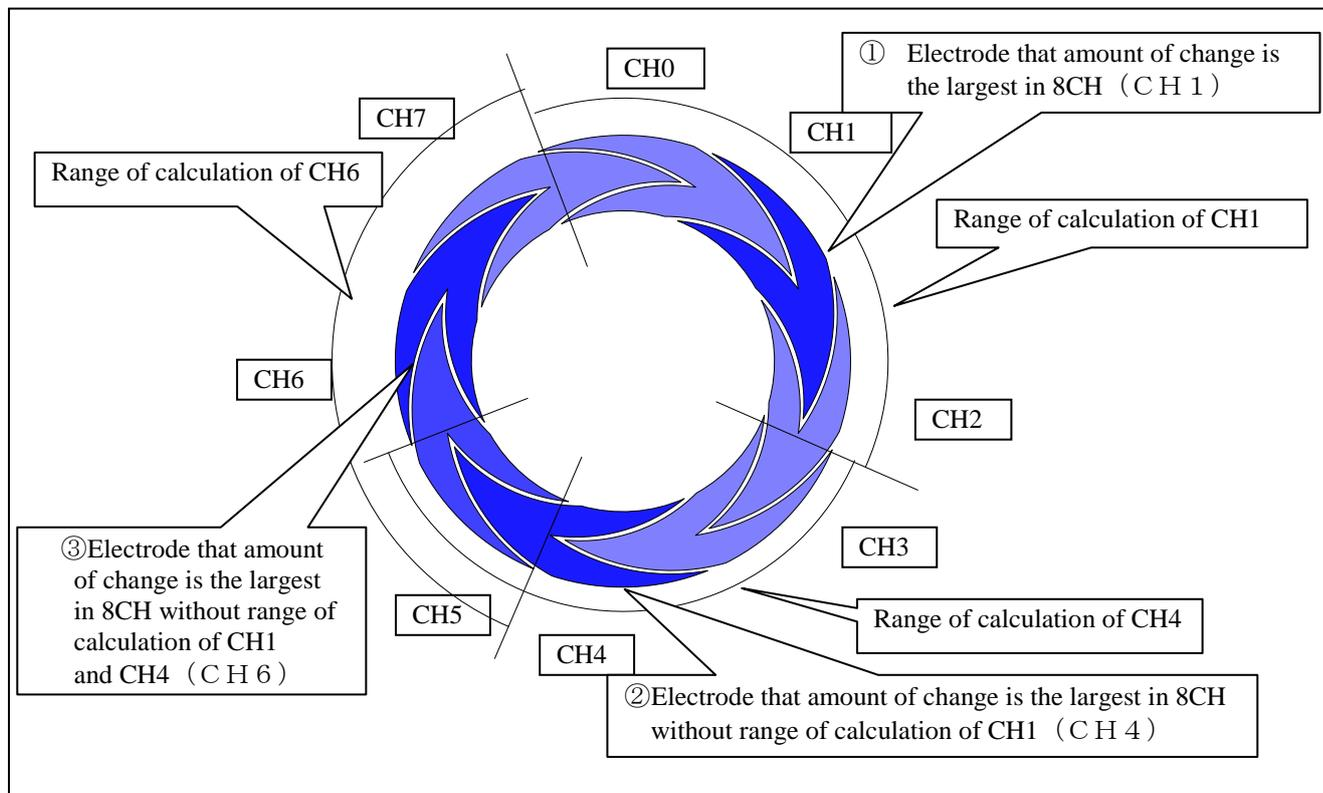
Figure 3-2- 1 Multi positioning operation explanation chart in eight electrode wheel
