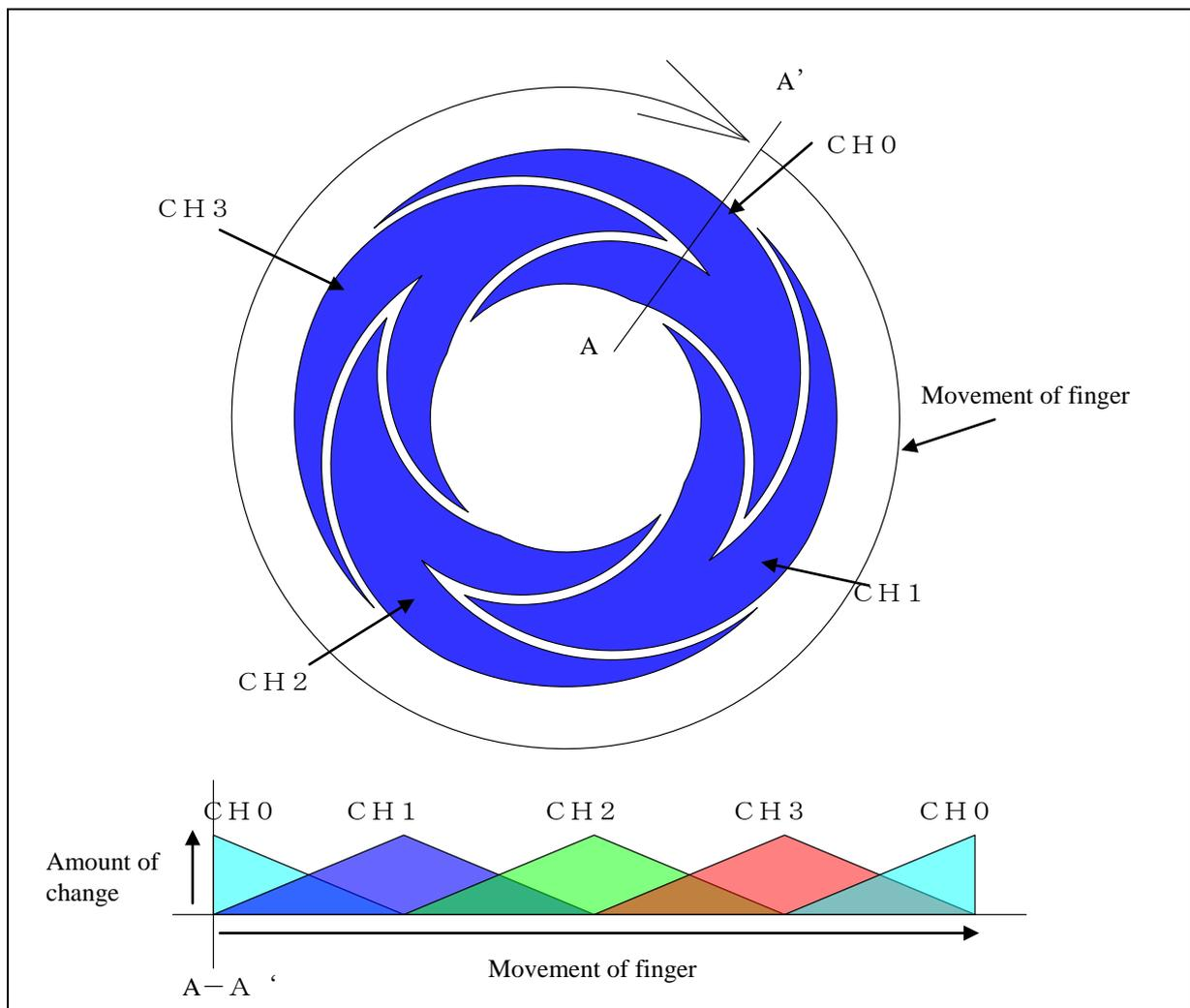
Figure 1-2- 1 Example of composing wheel by four electrodes
