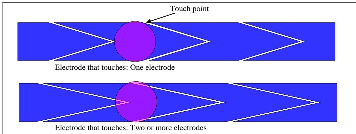
Figure 1-3-2 Touch area and electrode geometry
