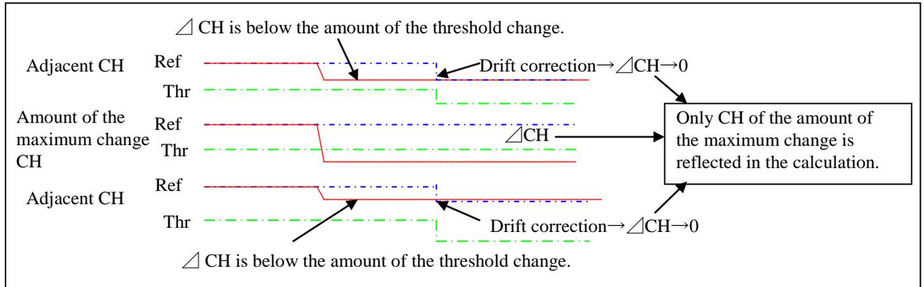
Figure 4-1- 1 Drift correction operation explanation chart
