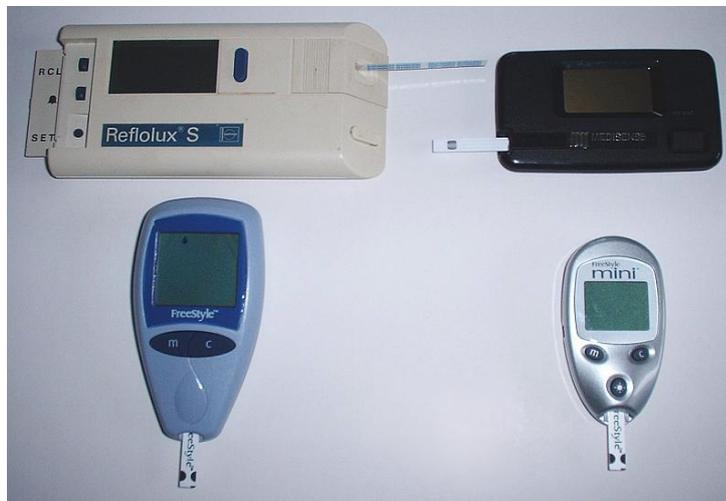
Figure 1: Example Blood Glucose Meters- Four Generations
