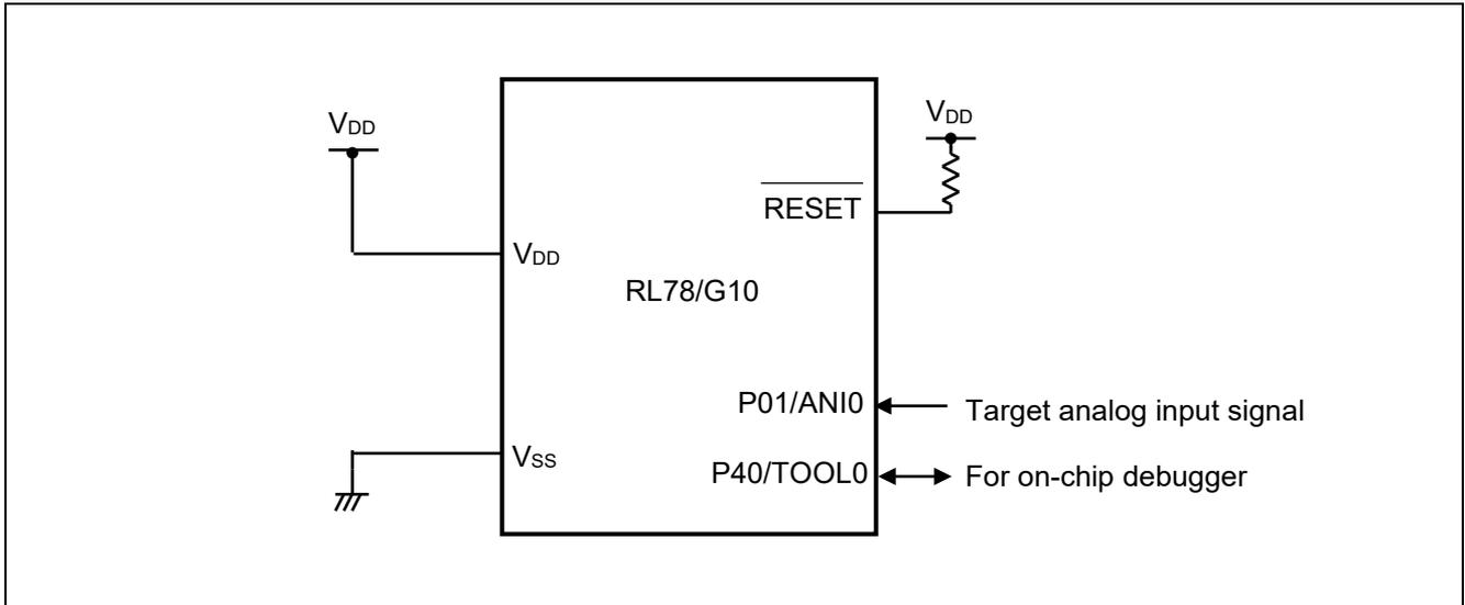
**Figure 4.1 Hardware Configuration**
