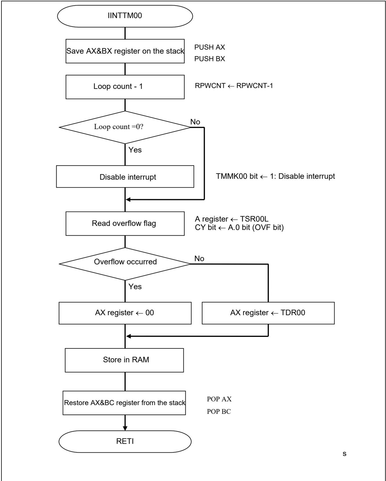
**Figure 5.8 INTTM00 Interrupt Processing**
