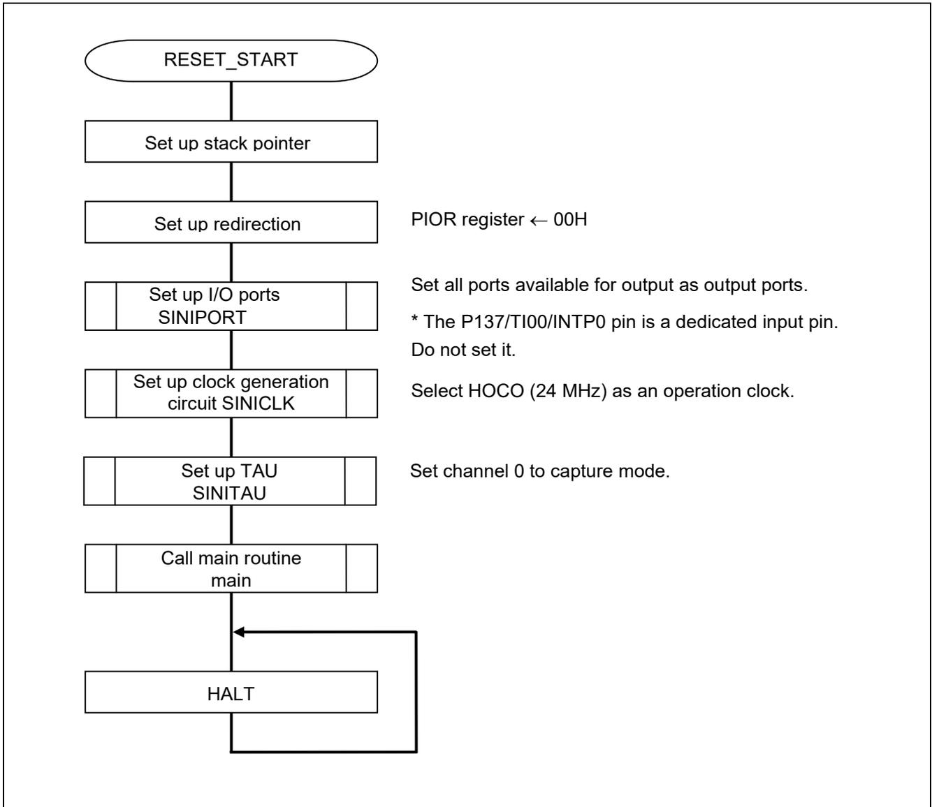
**Figure 5.2 CPU Initialization Function**
