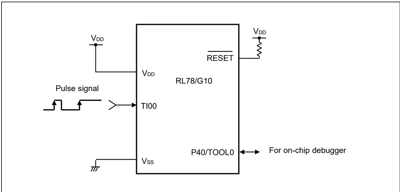
**Figure 4.1 Hardware Configuration**
