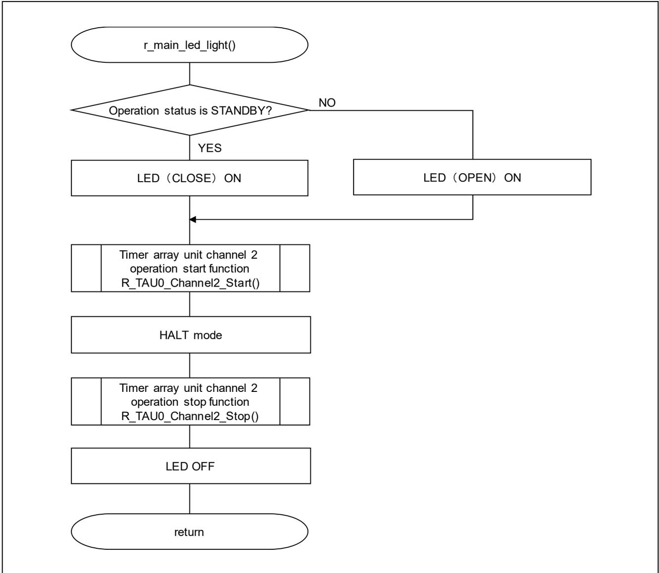
Figure 5.18 LED Blinking Processing
