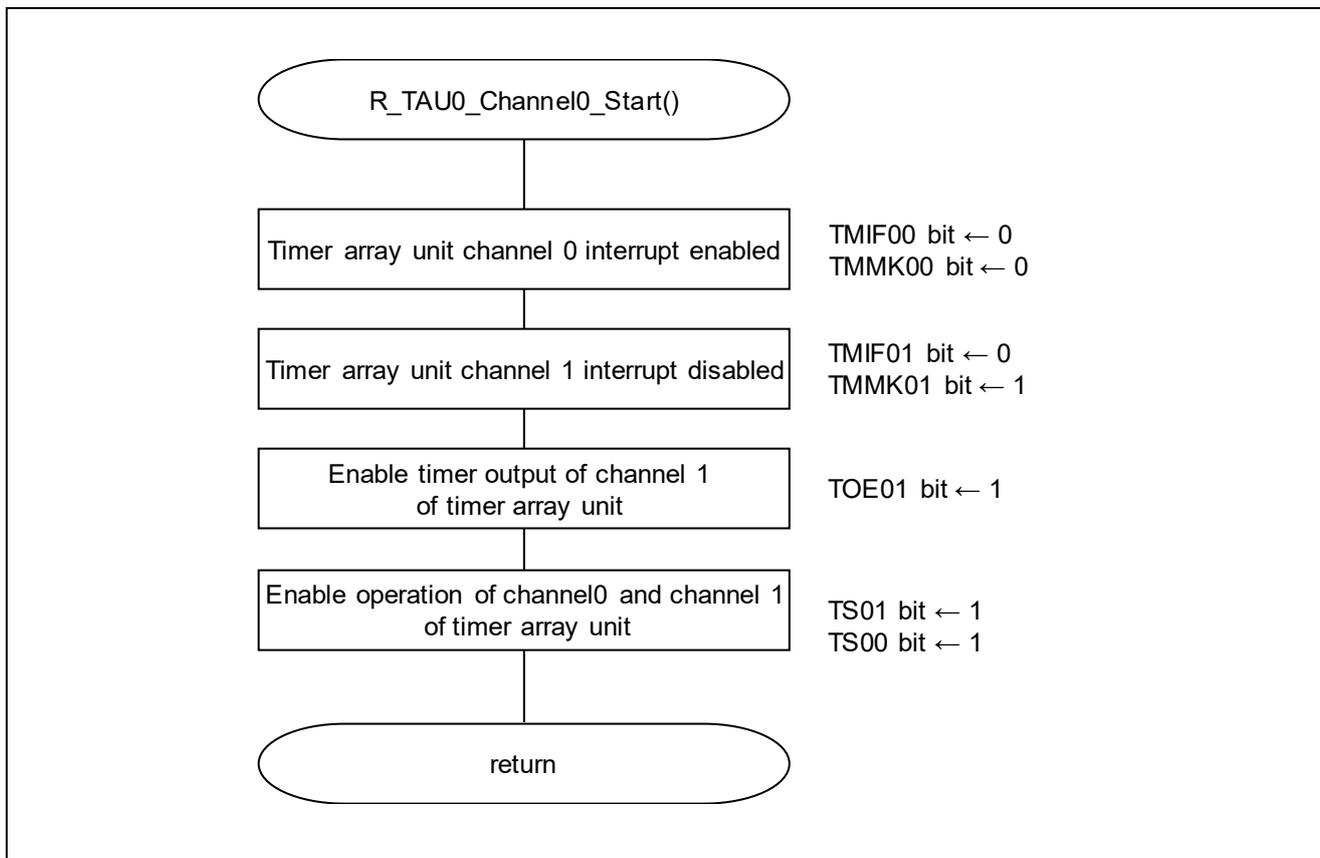
Figure 5.22 Timer Array Unit Channel0 Operation Start Function
