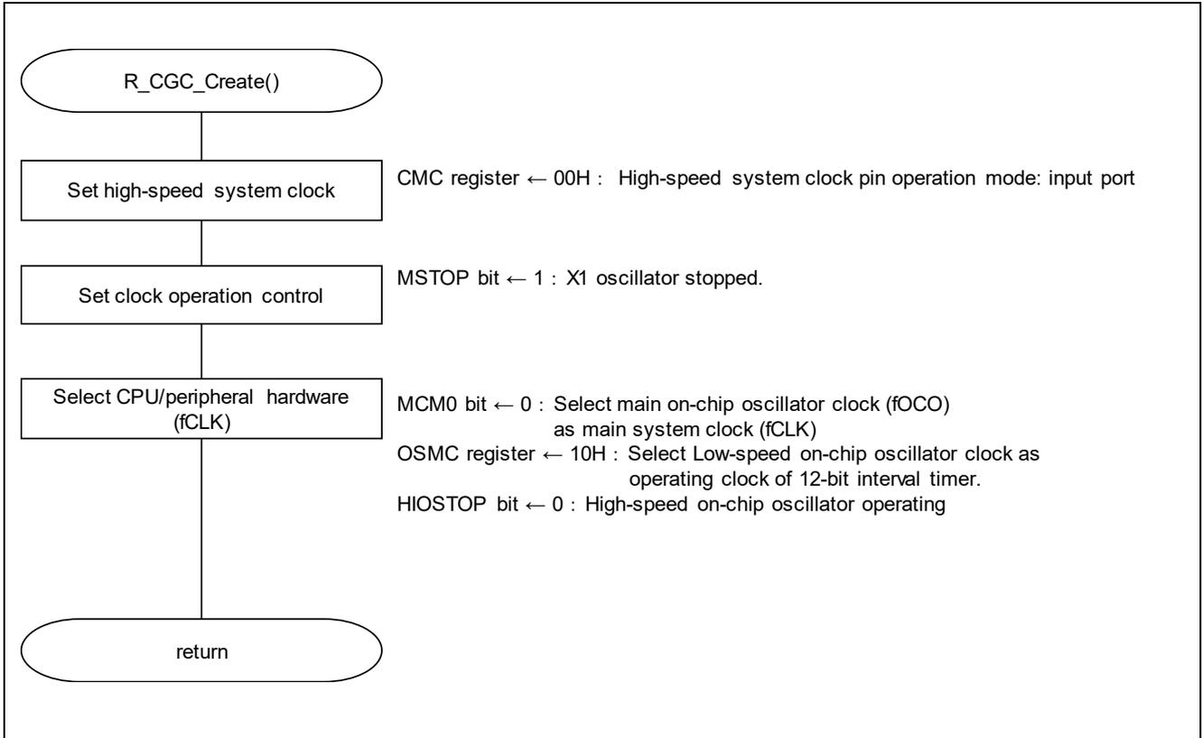
Figure 5.5 CPU Initial Setting
