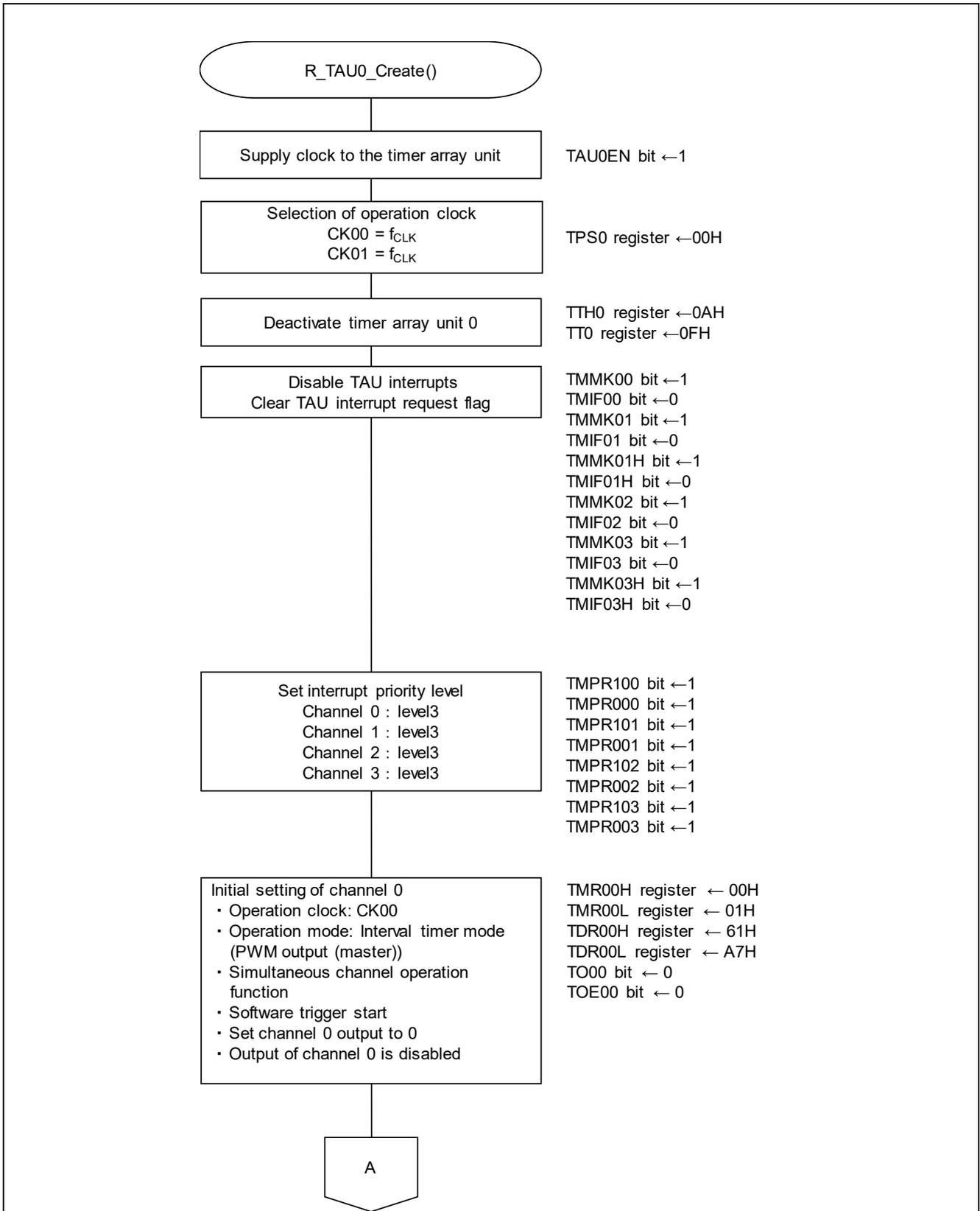
Figure 5.6 Timer Array Unit Initial Setting (1/2)
