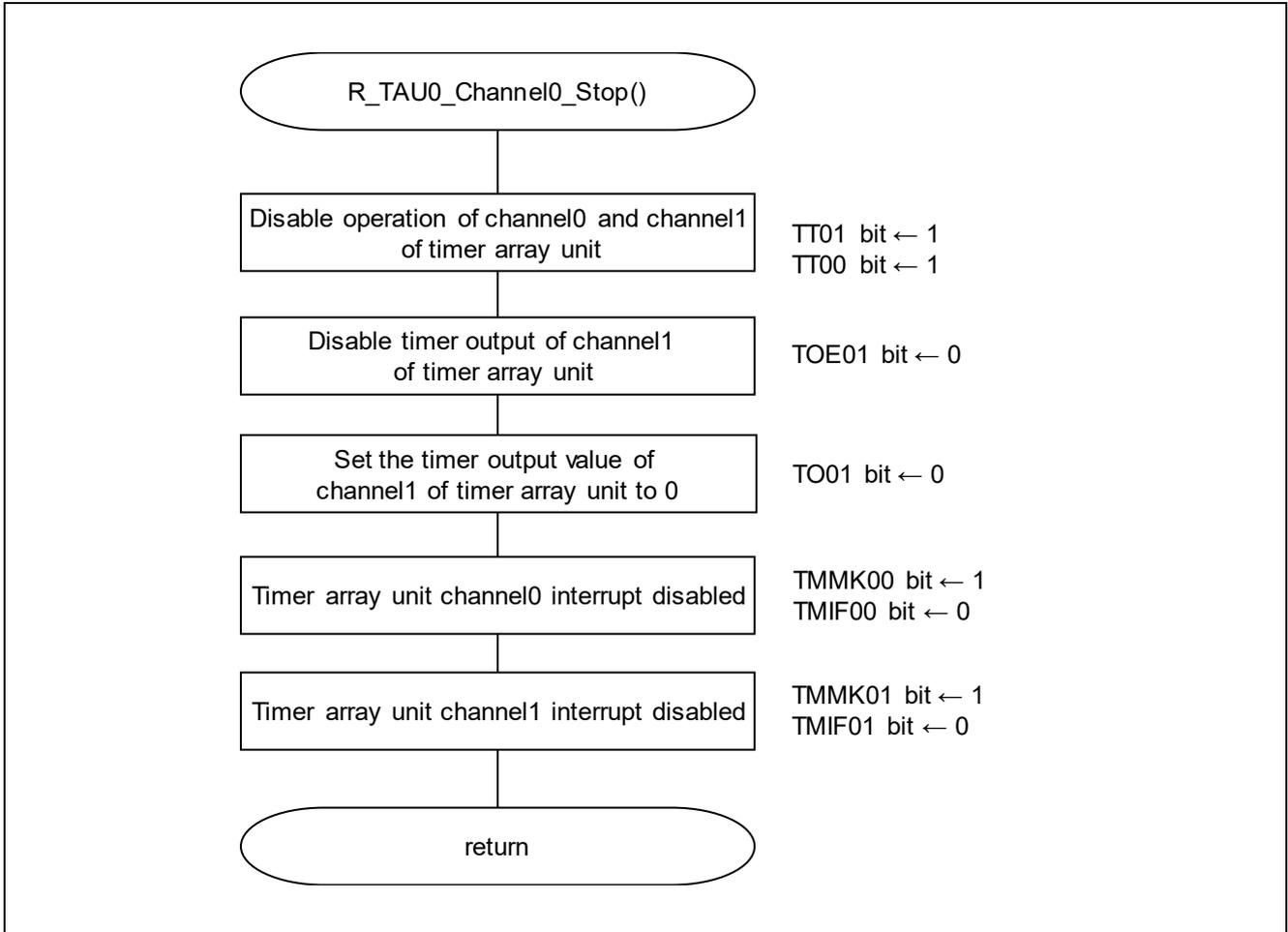
Figure 5.23 Timer Array Unit Channel0 Operation Stop Function
