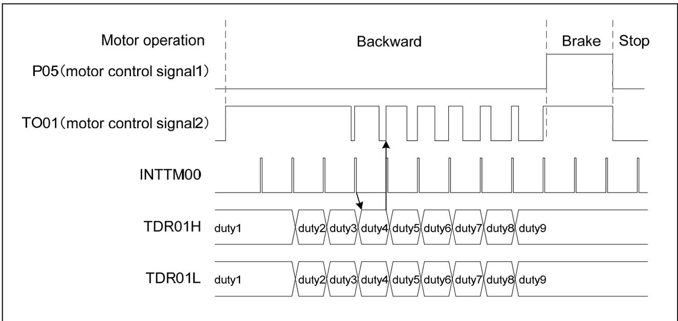
Figure 1.4 Motor Control to Open the Lid
