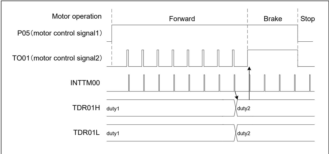
Figure 1.3 Motor Control to Close the Lid
