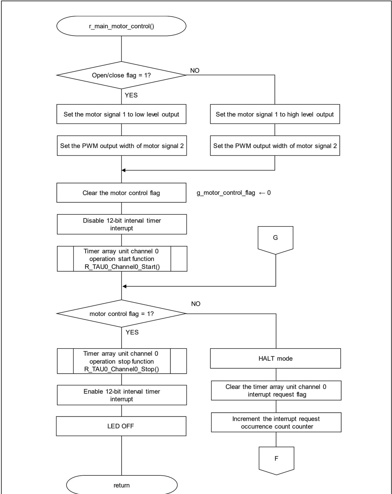
Figure 5.14 Motor Control Function (1/2)
