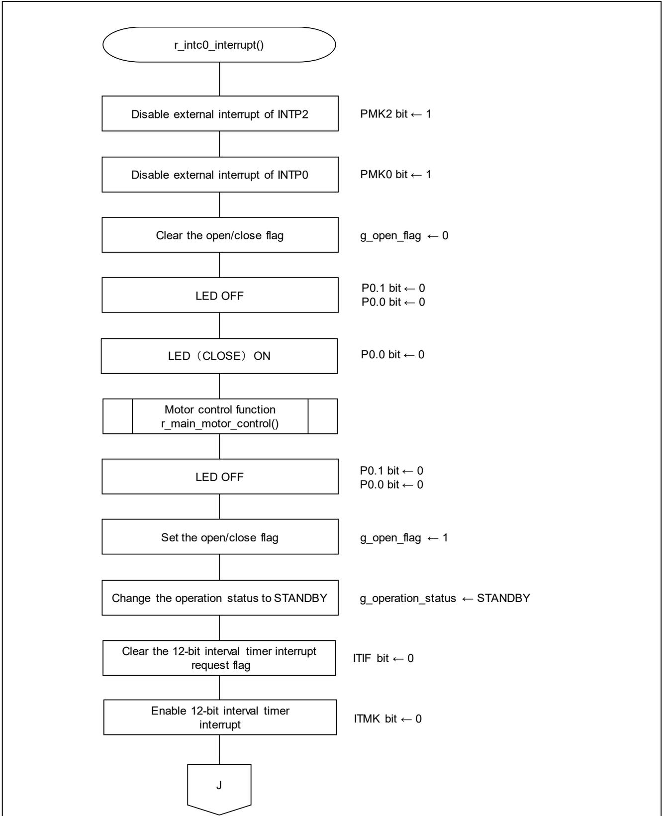
Figure 5.29 External Interrupt Processing of INTP0 (1/2)
