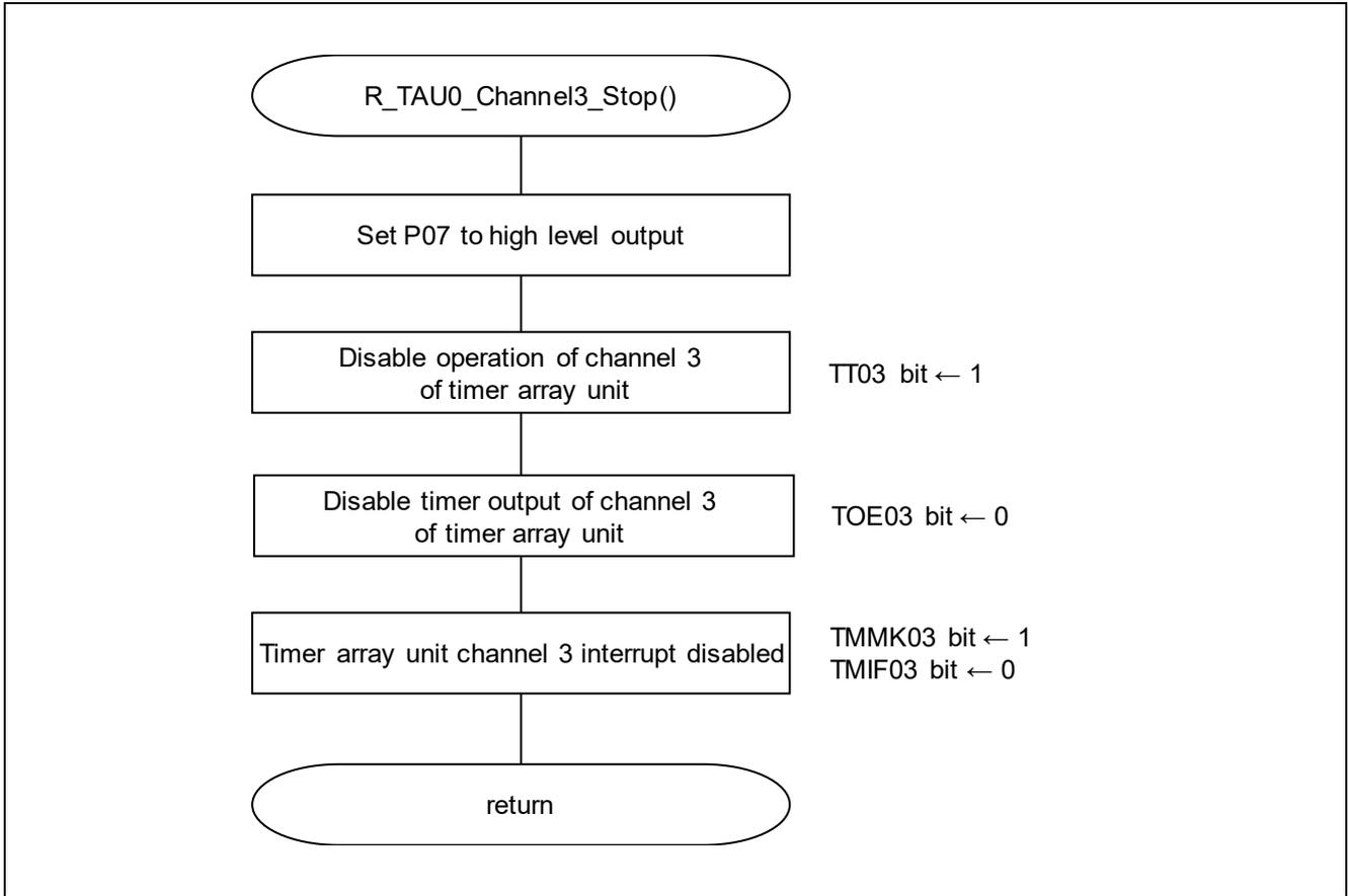
Figure 5.27 Timer Array Unit Channel3 Operation Stop Function
