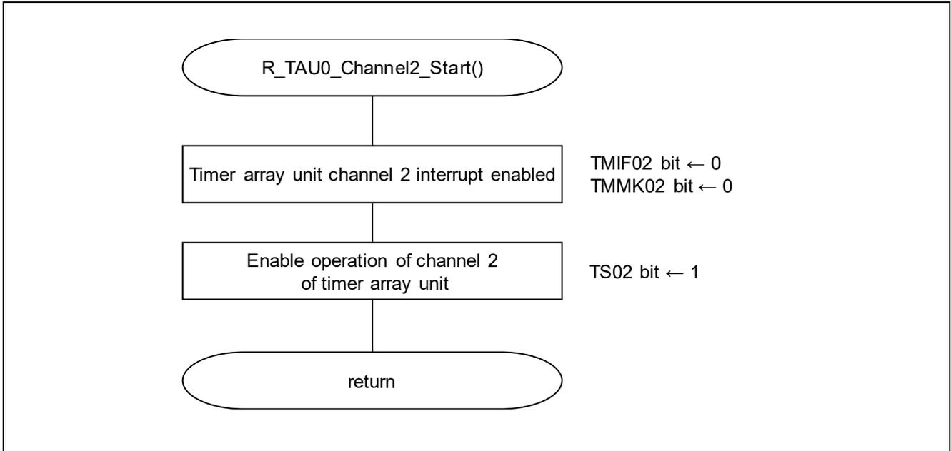
Figure 5.24 Timer Array Unit Channel2 Operation Start Function
