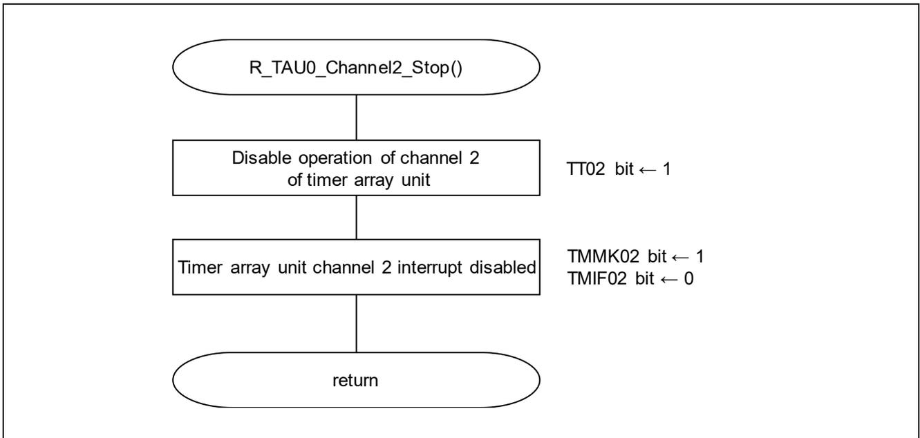
Figure 5.25 Timer Array Unit Channel2 Operation Stop Function
