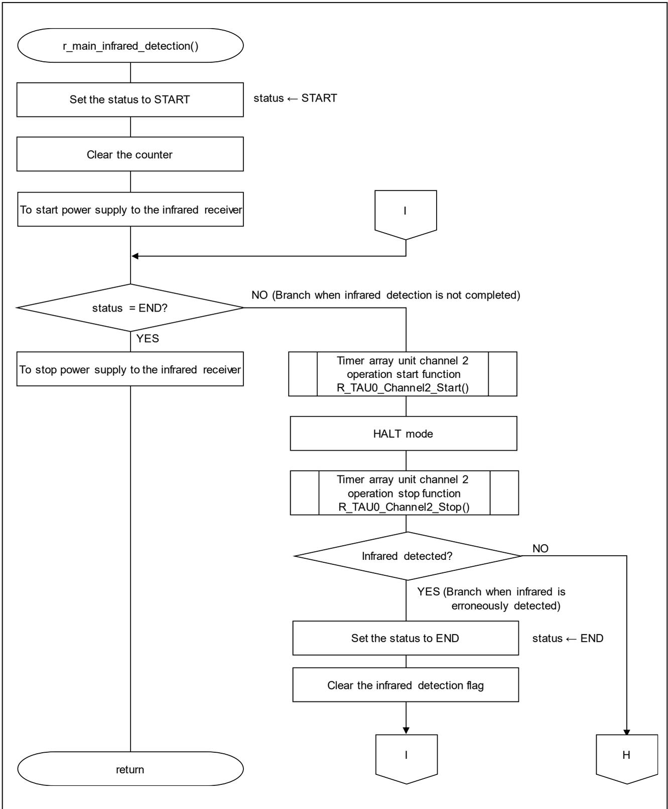
Figure 5.16 Infrared Detection Processing (1/2)
