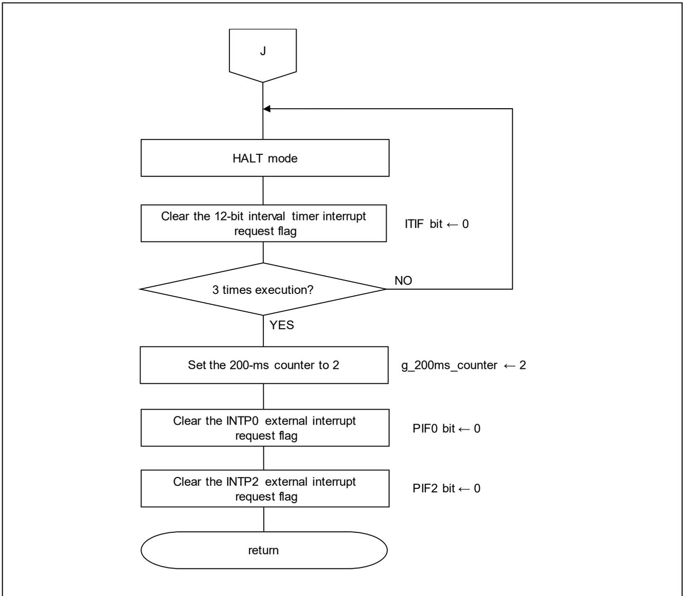
Figure 5.30 External Interrupt Processing of INTP0 (2/2)
