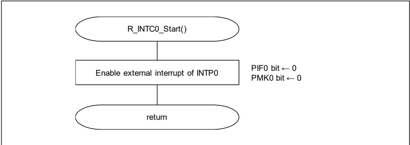
Figure 5.19 External Interrupt Processing of INTP0
