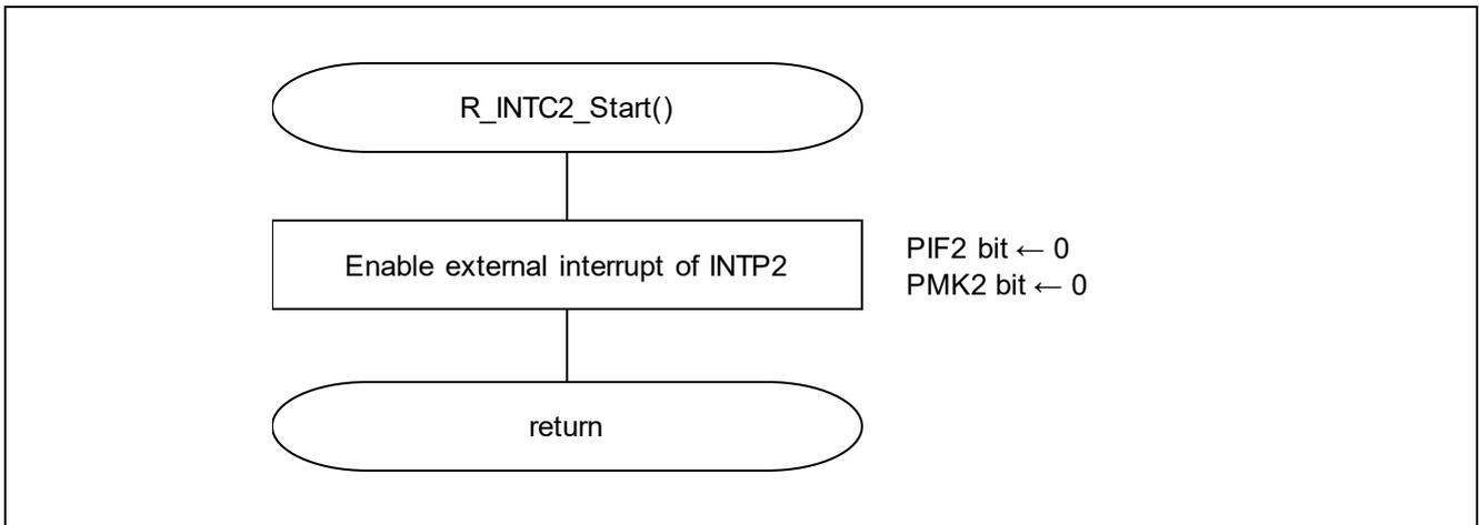
Figure 5.20 External Interrupt Processing of INTP2
