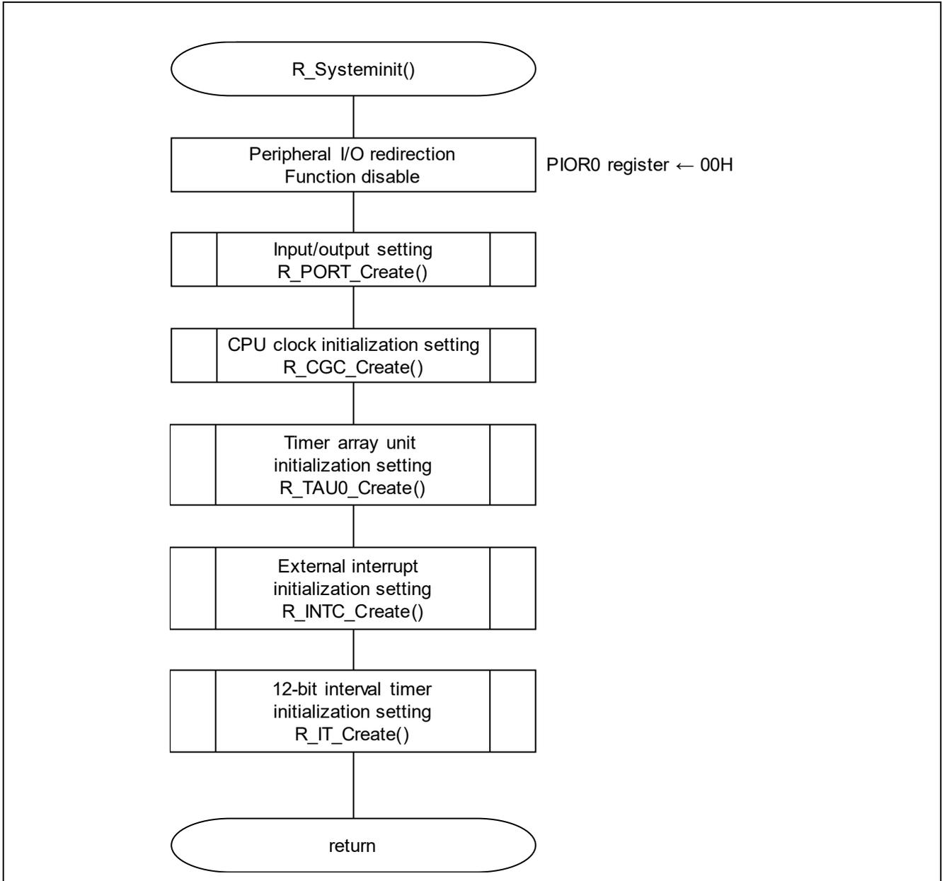
Figure 5.3 System Initial Setting
