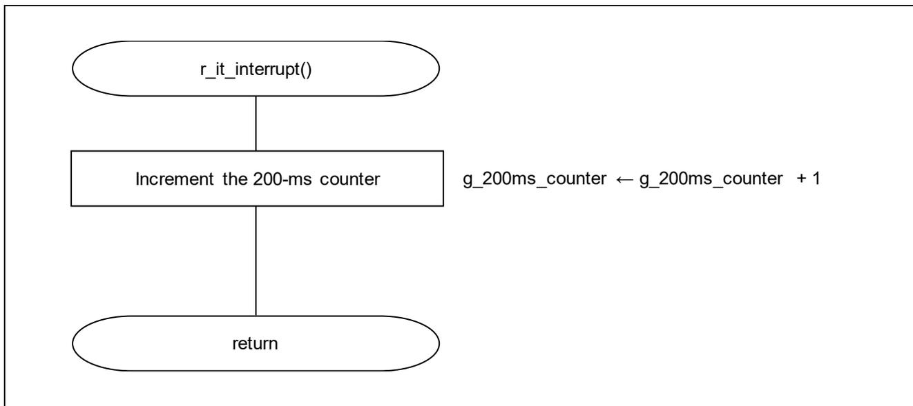
Figure 5.28 Interval Timer Signal Detection Interrupt Function
