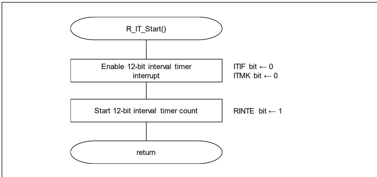
Figure 5.21 12-bit Interval Timer Operation Start
