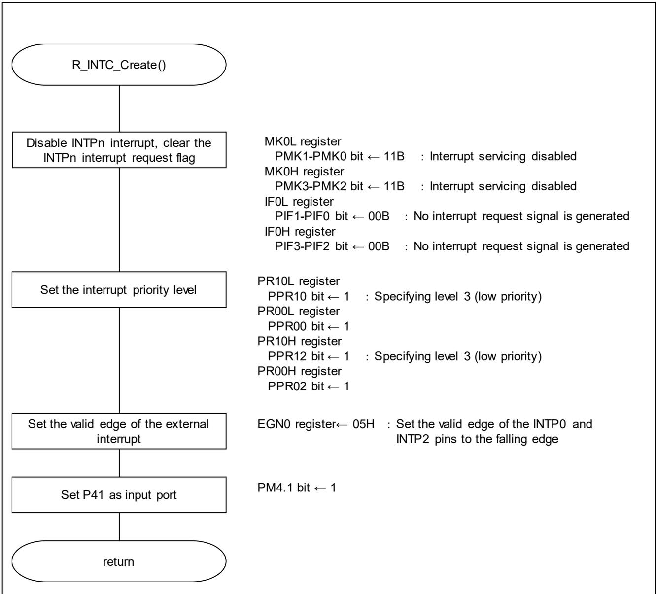
Figure 5.8 External Interrupt Setting
