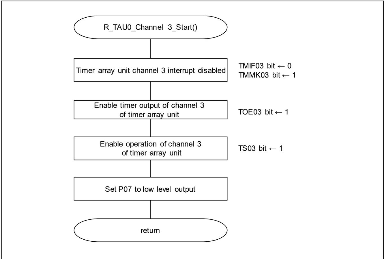
Figure 5.26 Timer Array Unit Channel3 Operation Start Function
