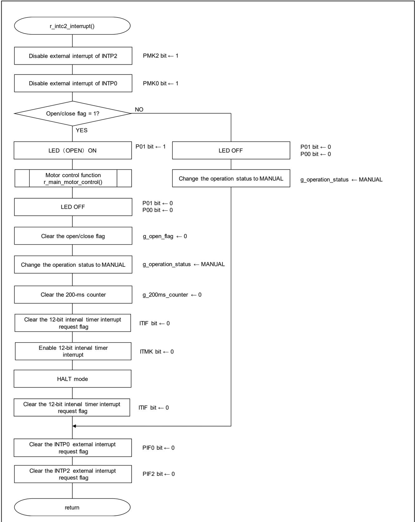
Figure 5.31 External Interrupt Processing of INTP2
