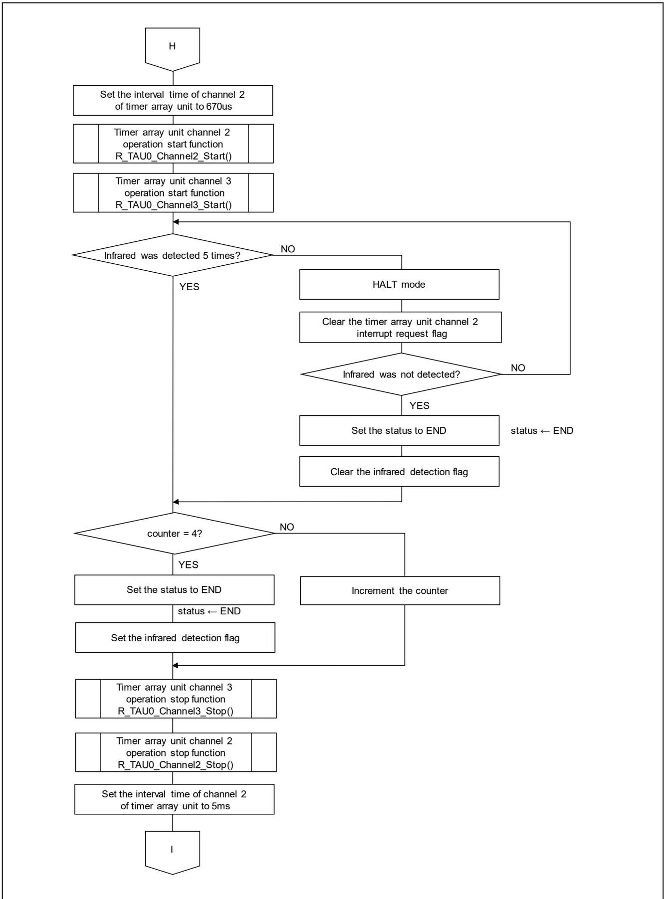
Figure 5.17 Infrared Detection Processing (2/2)
