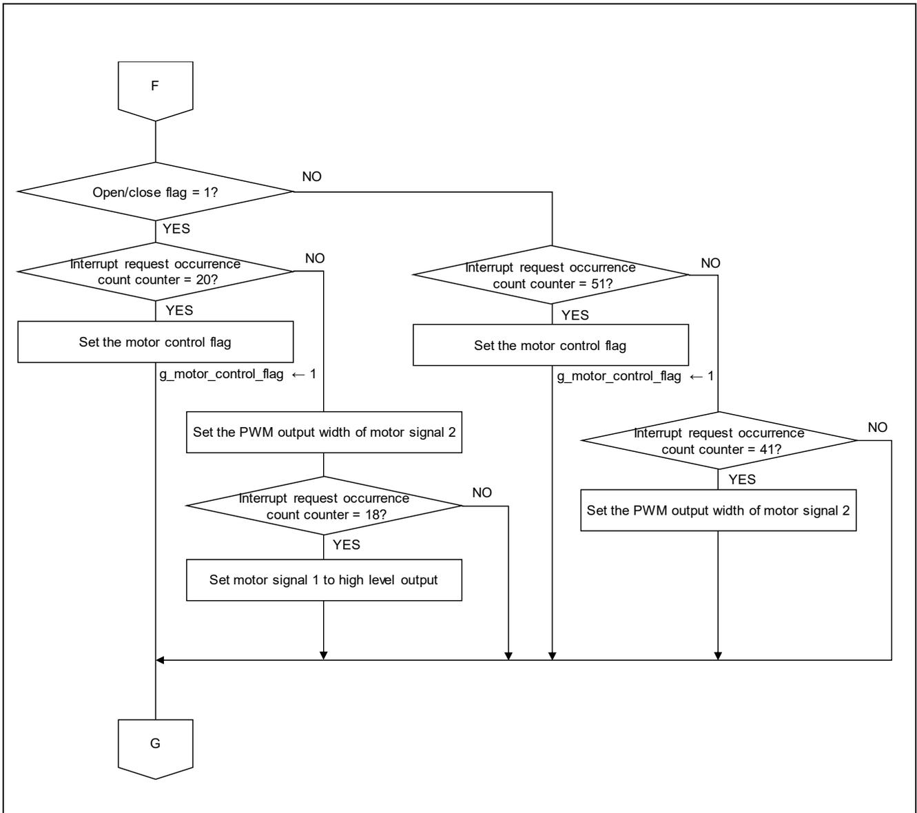
Figure 5.15 Motor Control Function (2/2)
