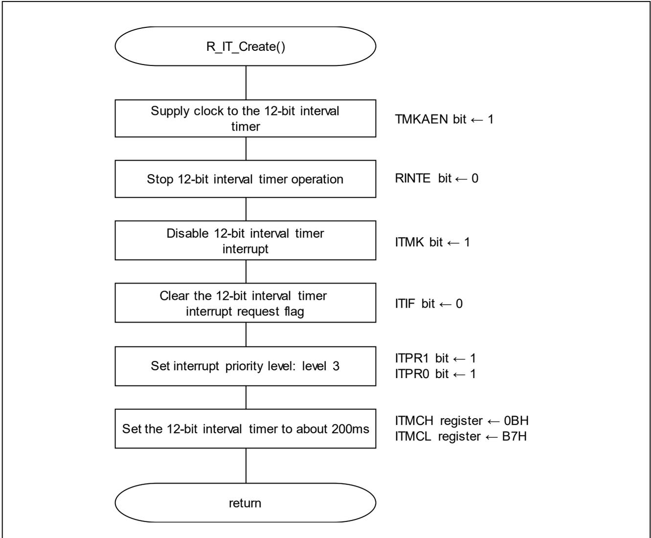
Figure 5.9 12-bit Interval Timer Initial Setting
