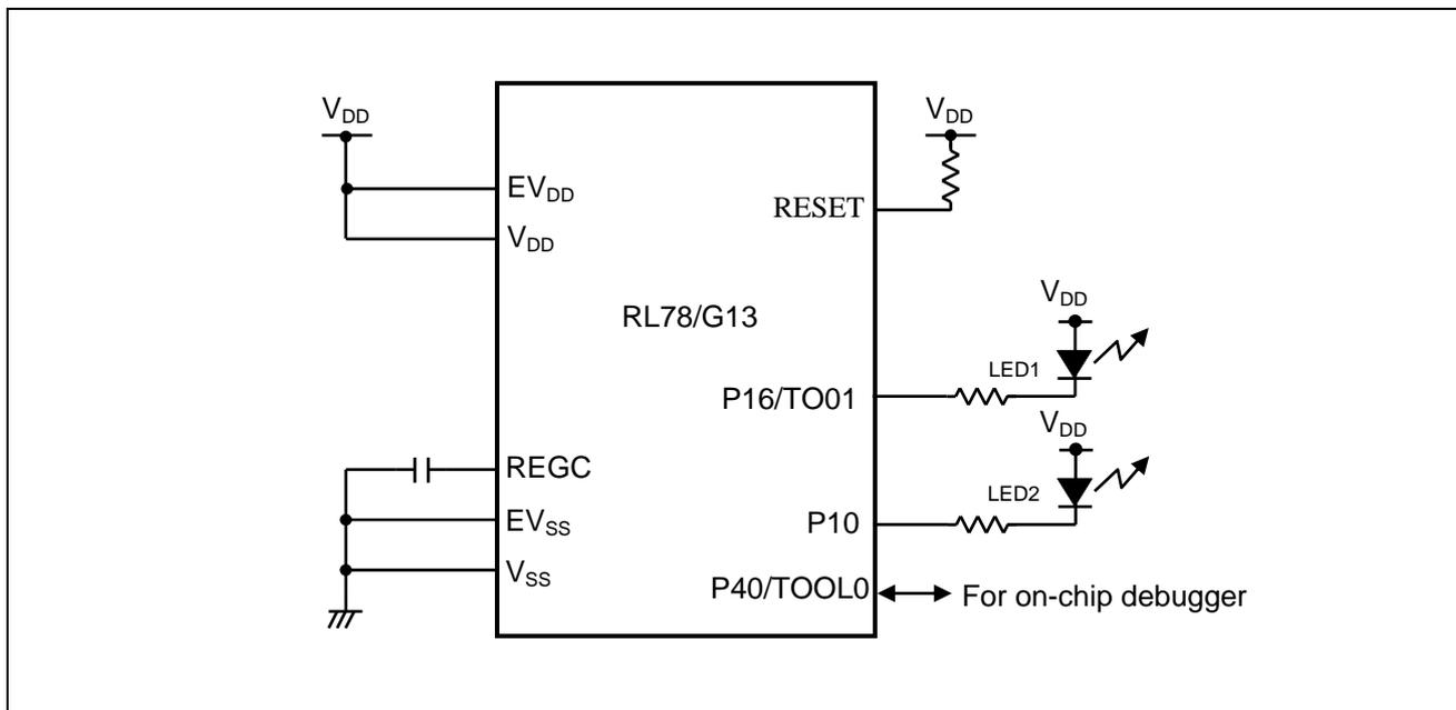
**Figure 4.1 Hardware Configuration**
