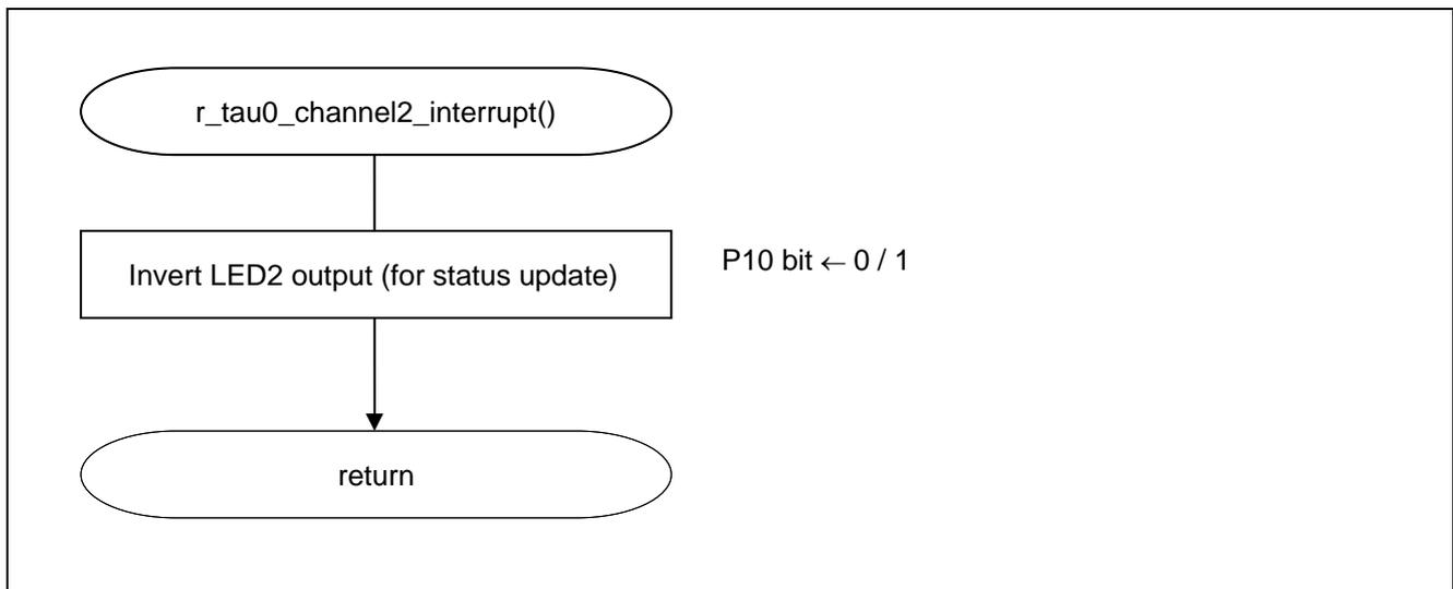
Figure 5.13 TAU0 Timer Interrupt Processing (Channel 2)
