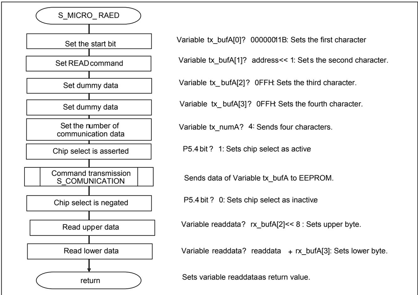
**Figure 5.17 Reading Data from Specified Address of EEPROM**
