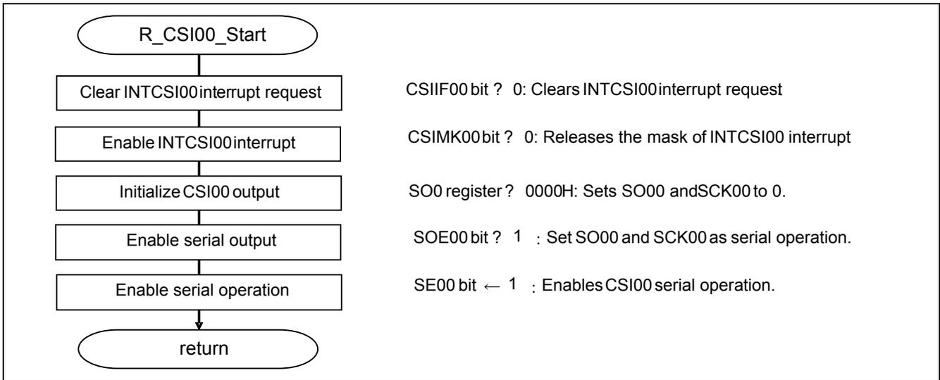
**Figure 5.12 Setting CSI00 to the Communication Standby Status**
