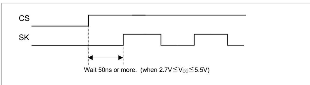
**Figure 1.2 Digital Timing Diagram of CS Pin**
