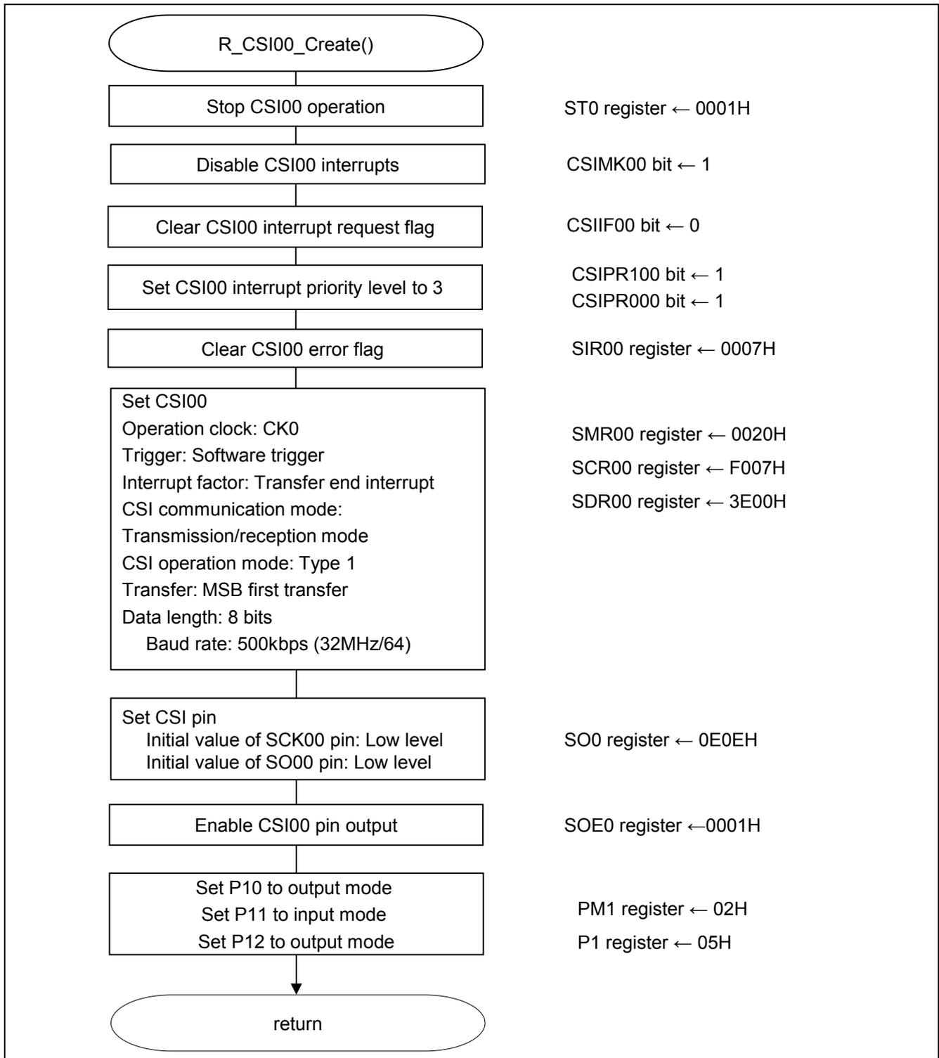
Figure 5.9 SAU0 Channel 0 (CSI00) Operation Setup
