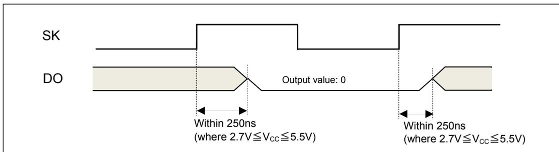
**Figure 1.4 Digital Timing Diagram of DO Pin**
