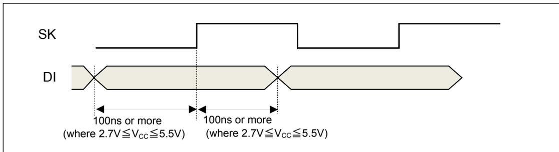
**Figure 1.3 Digital Timing Diagram of DI Pin**
