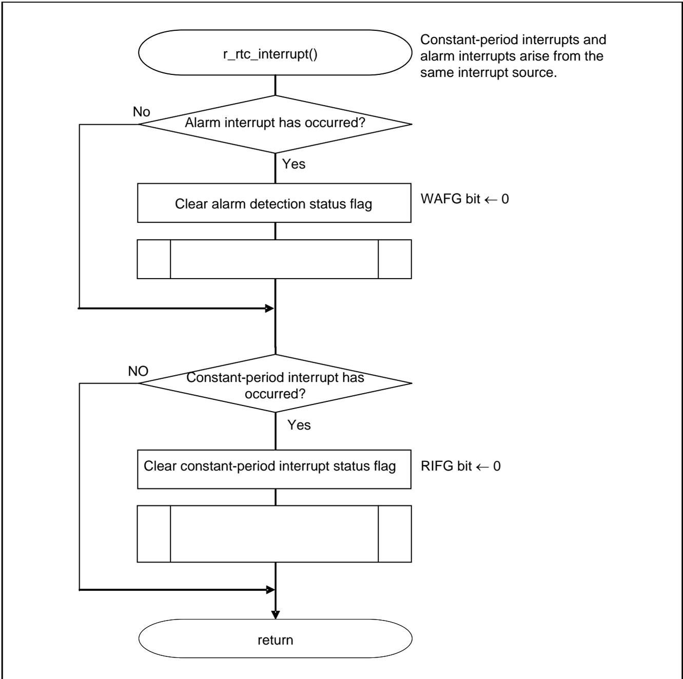
Figure 5.15 RTC Interrupt (INTRTC) Processing
