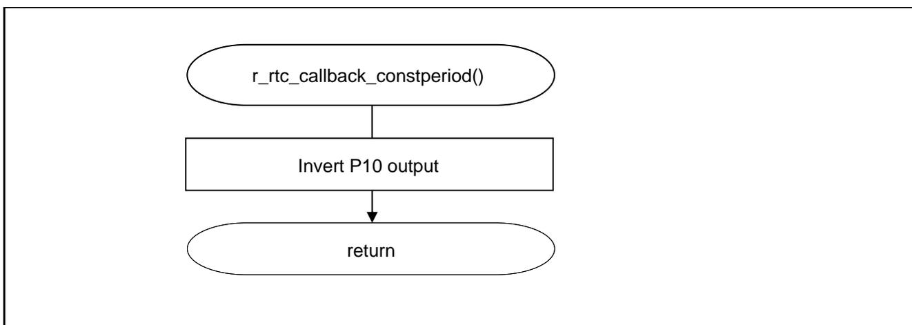
Figure 5.17 Constant-period Interrupt Processing
