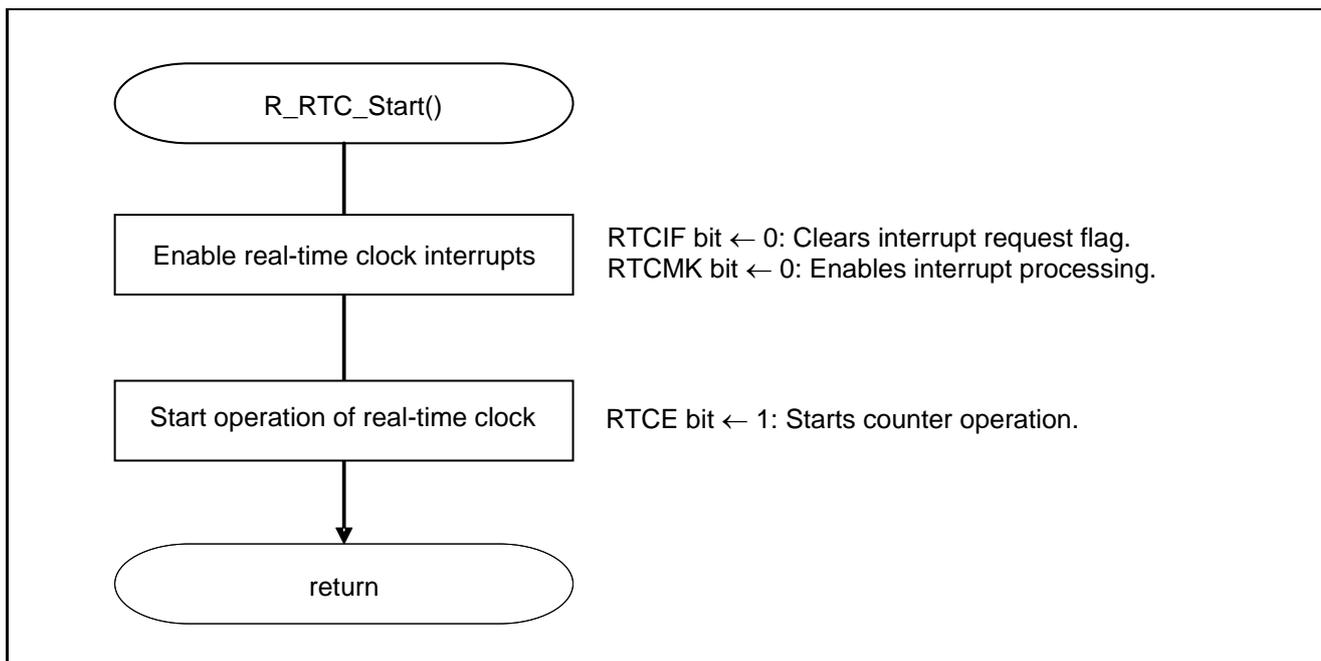
Figure 5.11 RTC Startup
