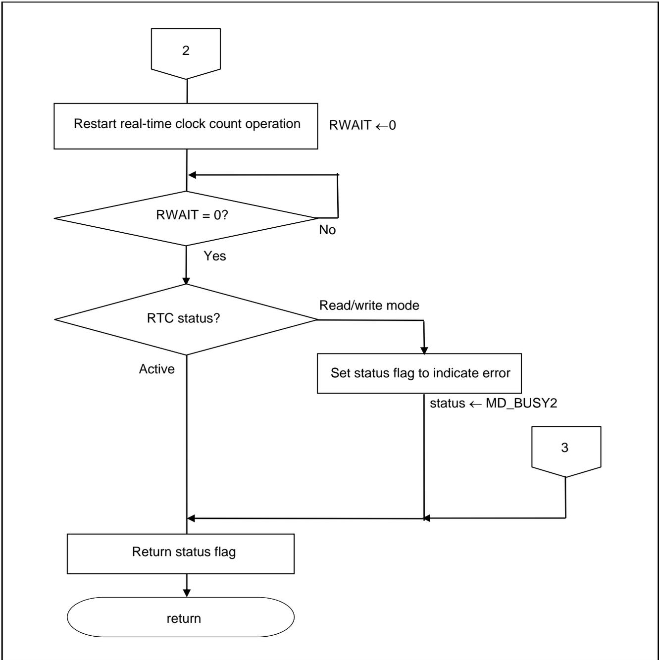
Figure 5.13 RTC Time Setup (2/2)
