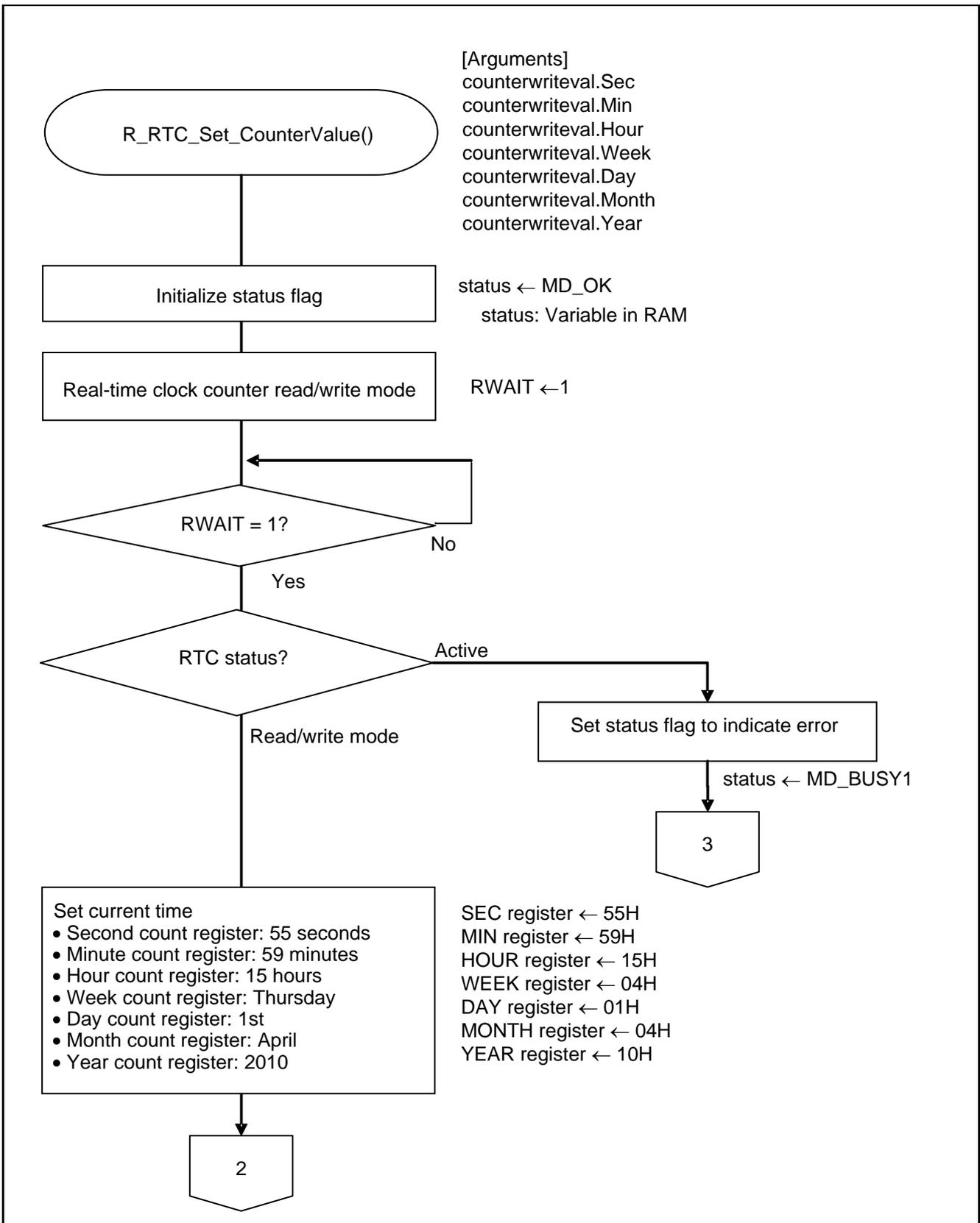
Figure 5.12 RTC Time Setup (1/2)
