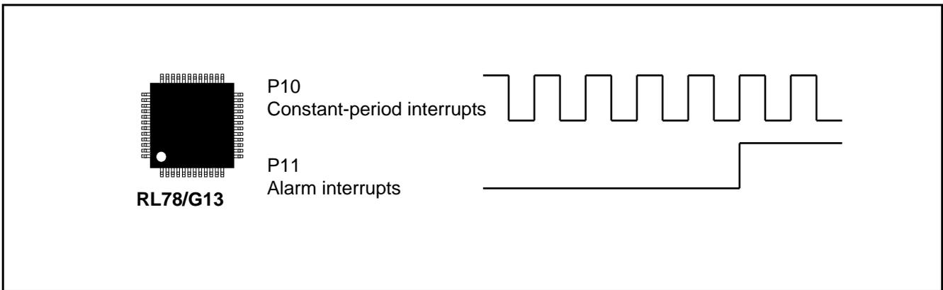
**Figure 1.1 Overview of Sample Code Operation**
