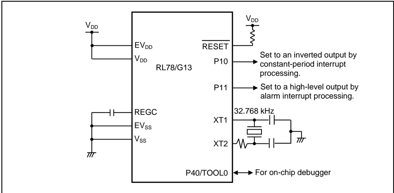
**Figure 4.1 Hardware Configuration**
