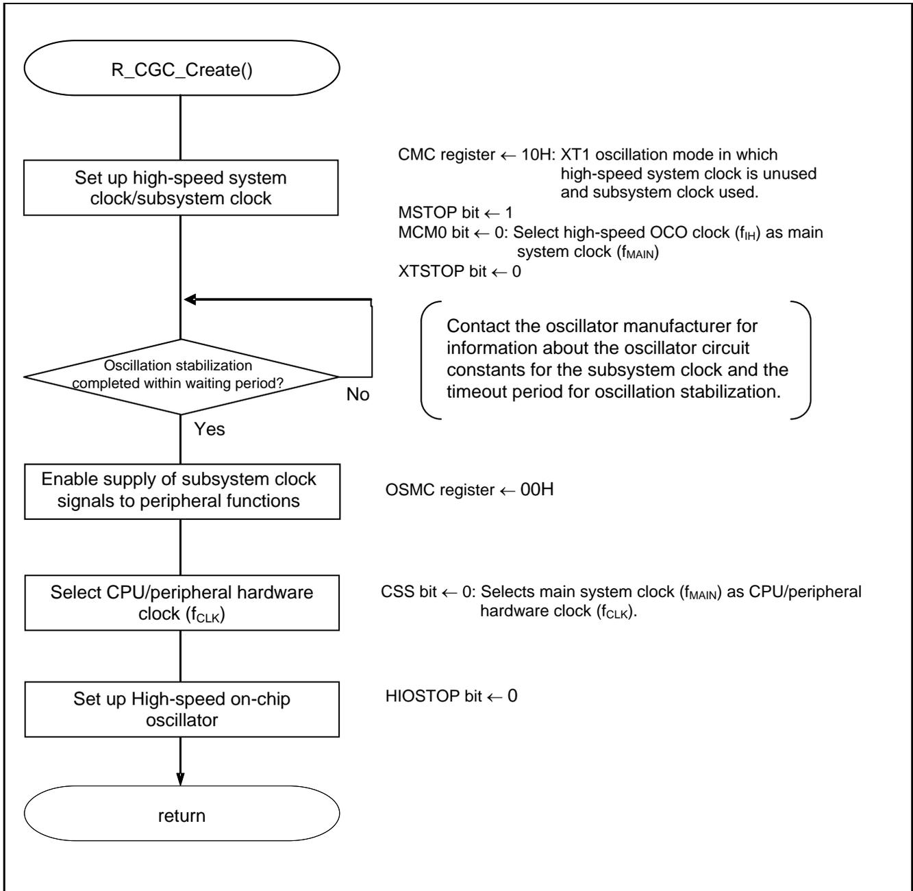
Figure 5.5 CPU Clock Setup
