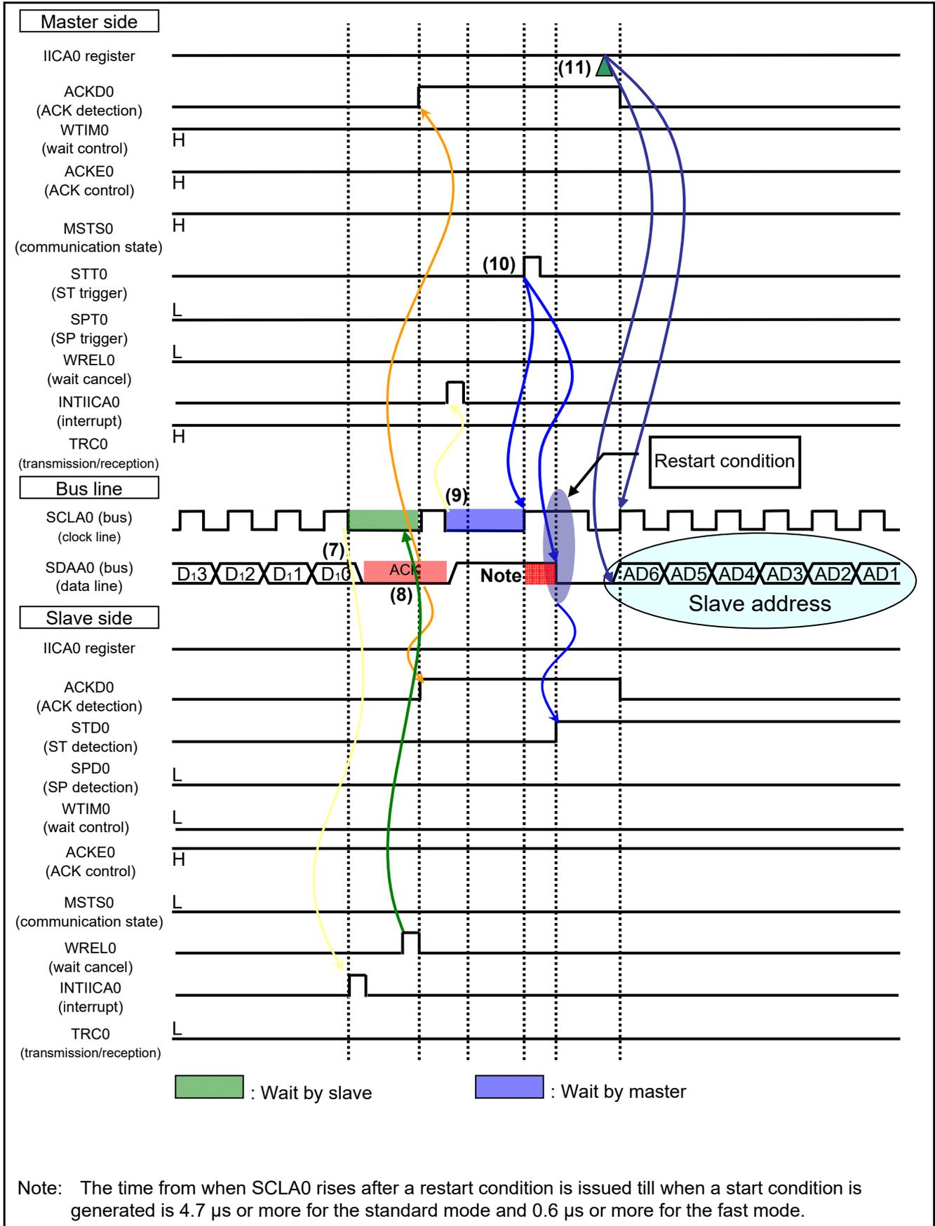
Figure 1.5 IIC Communication Timing Chart (Master-to-Slave Communication Example) (4/4)
