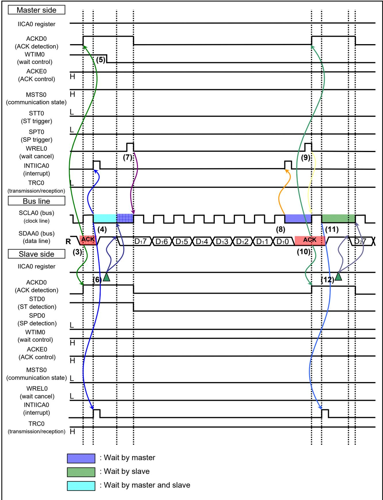
Figure 1.7 IIC Communication Timing Chart (Slave-to-Master Communication Example) (2/3)
