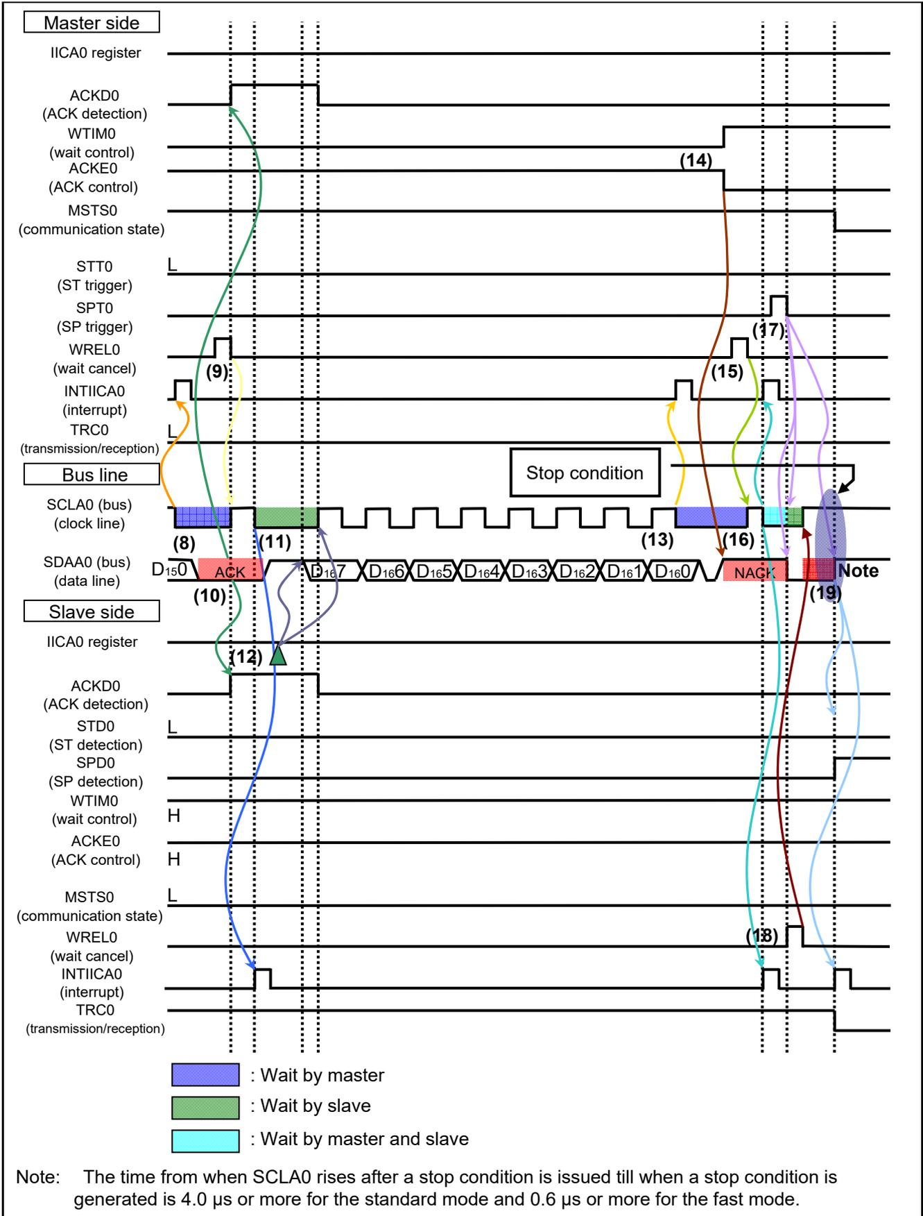
Figure 1.8 IIC Communication Timing Chart (Slave-to-Master Communication Example) (3/3)
