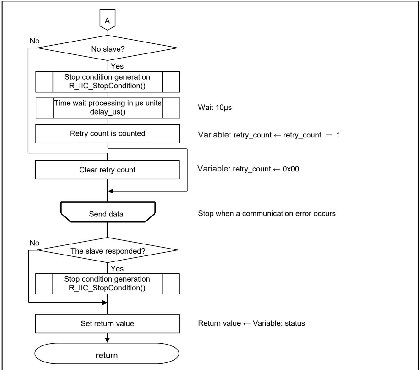
Figure 5.17 Processing of sending data to slave (2/2)
