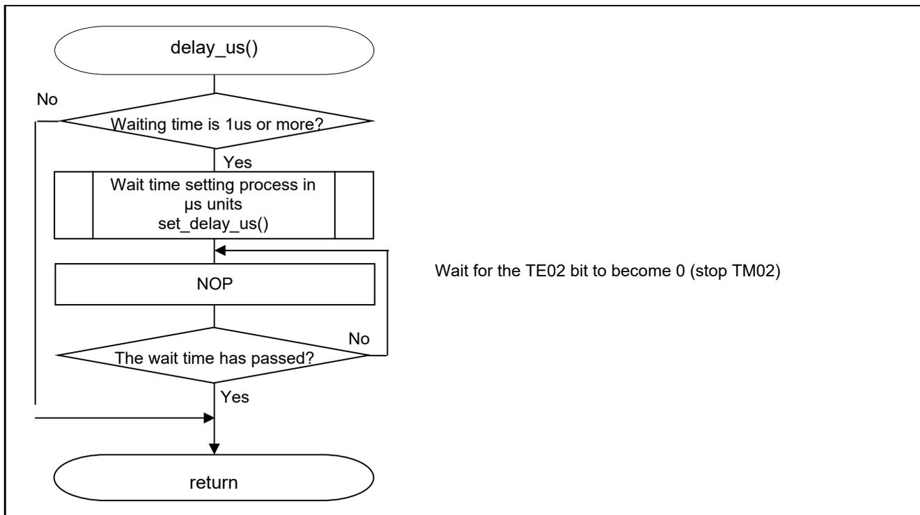
Figure 5.29 Time Wait Processing In  $\mu$ s units
