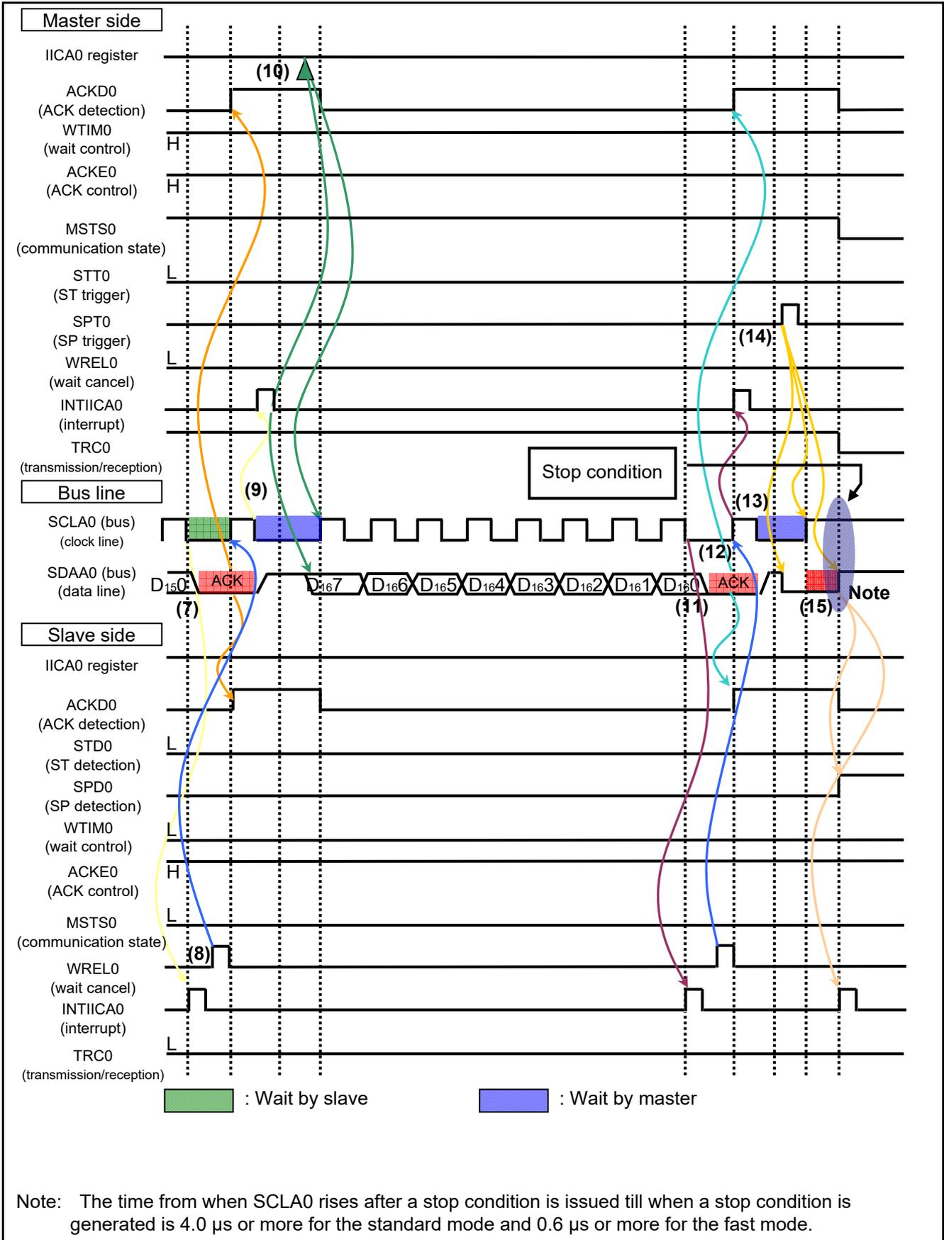
Figure 1.4 IIC Communication Timing Chart (Master-to-Slave Communication Example) (3/4)
