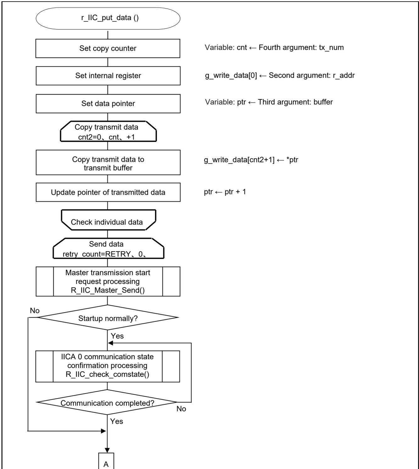
Figure 5.16 Processing of sending data to slave (1/2)
