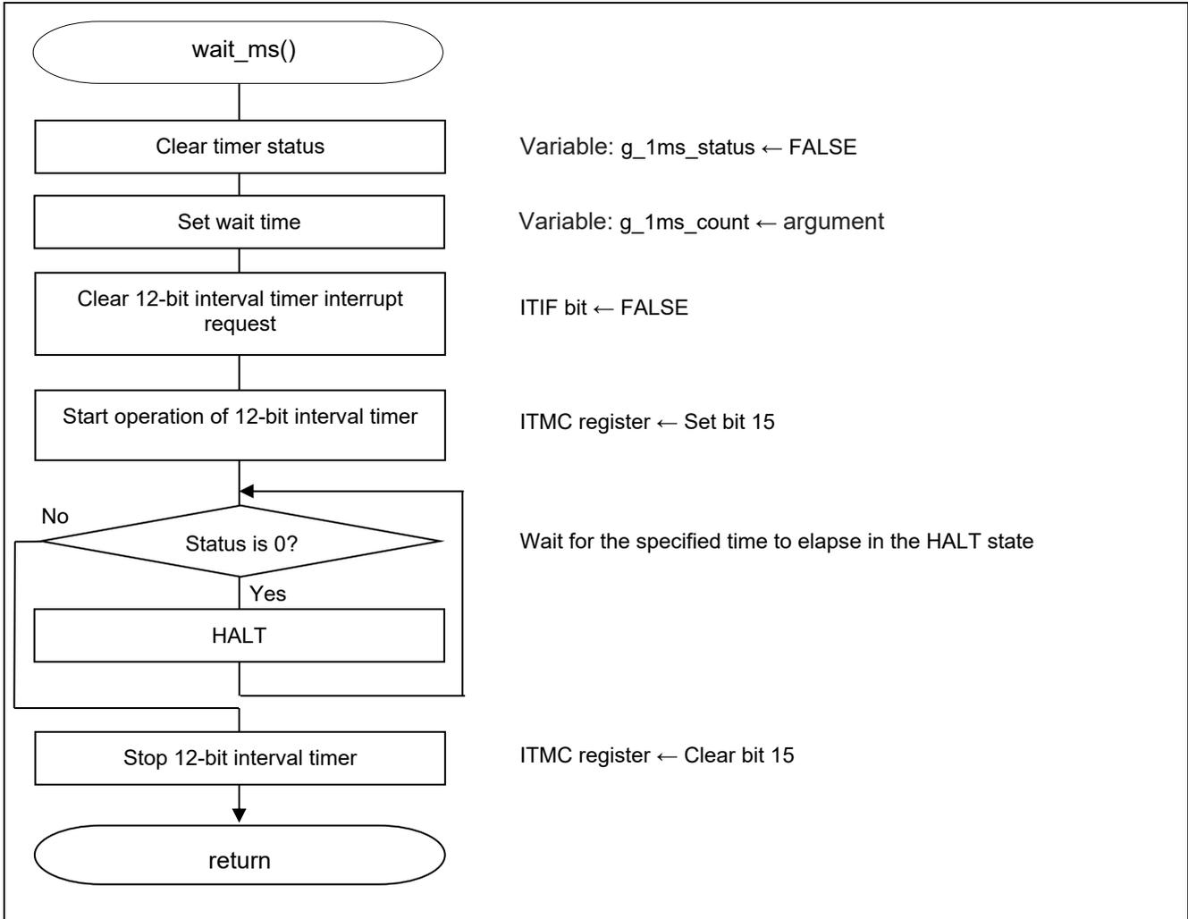
Figure 5.14 Time Wait Processing in ms units
