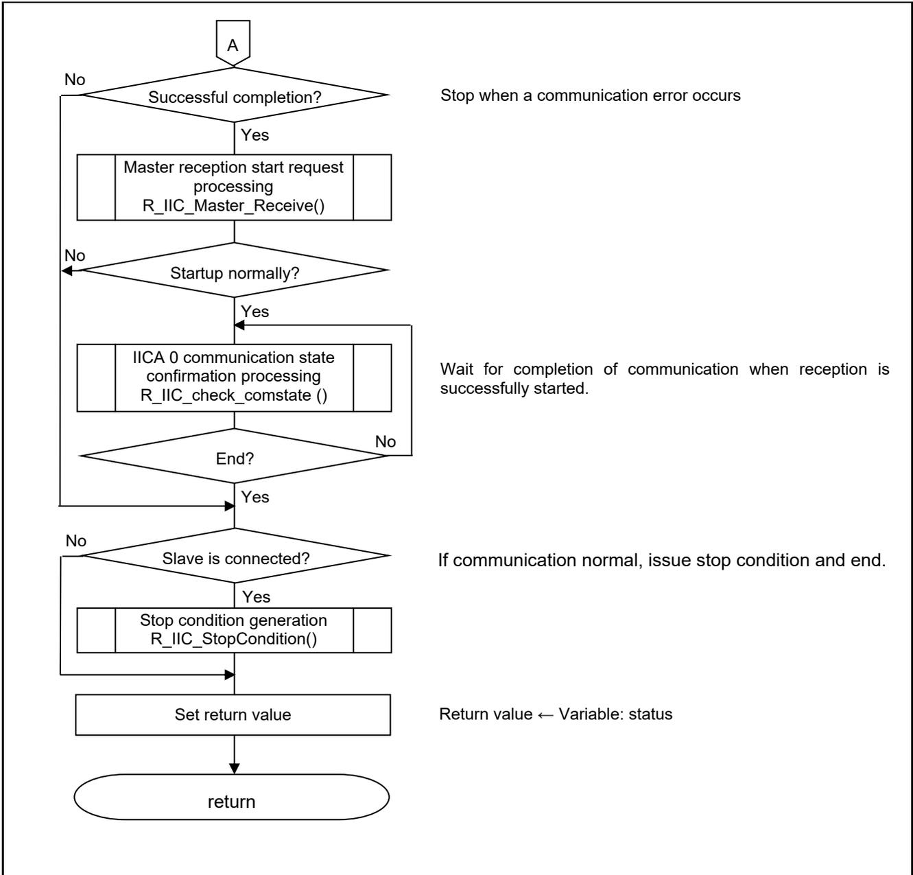
Figure 5.19 processing to receive data from slave (2/2)
