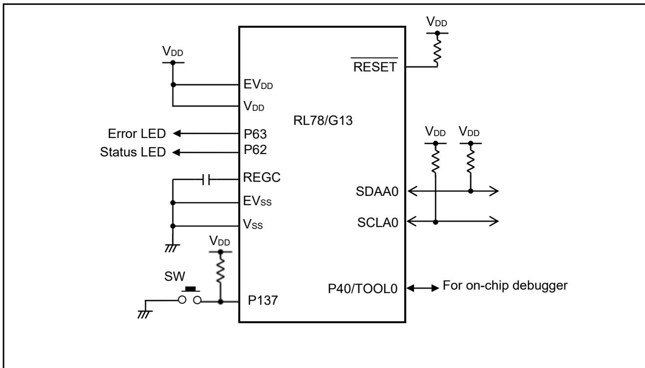
Figure 4.1 Hardware Configuration
