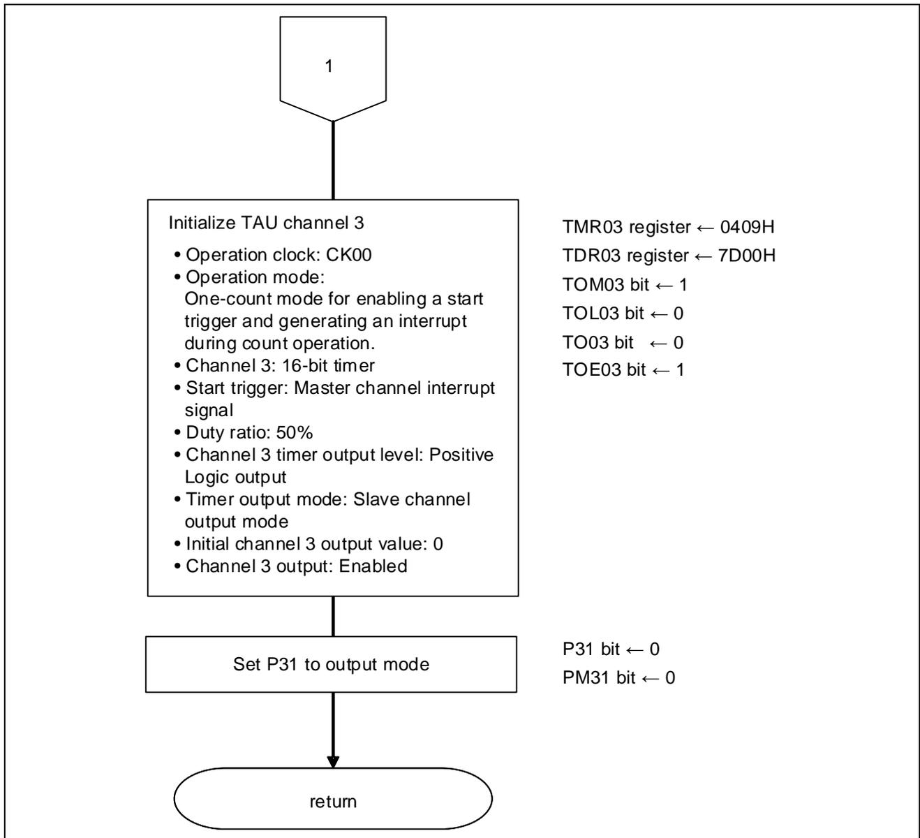
Figure 5.10 Timer Array Unit Setup (2/2)
