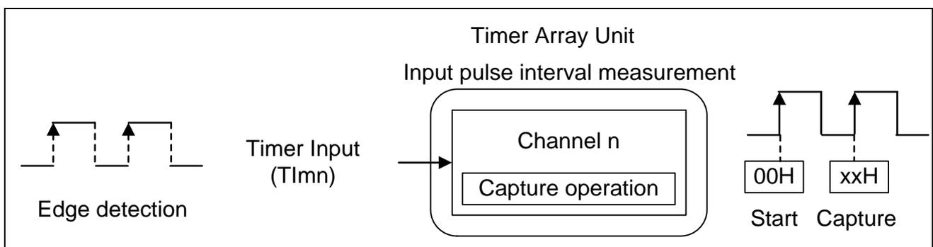
**Figure 4.1 Operation Overview (Example of Migration from Input Capture Mode)**
