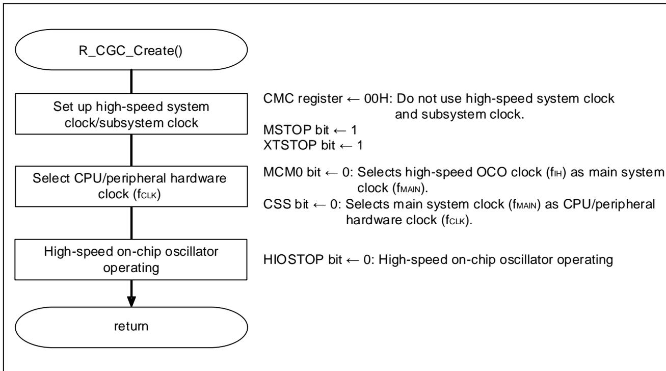
Figure 5.7 CPU Clock Setup
