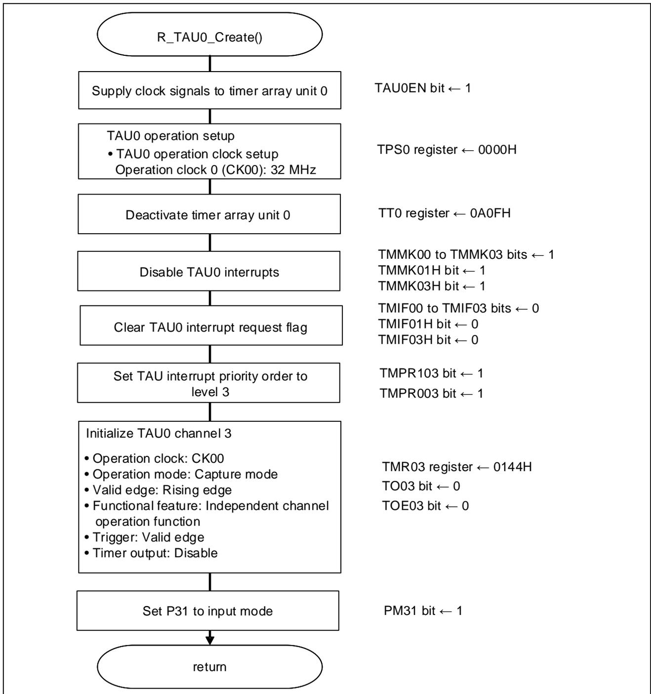
Figure 4.9 Timer Array Unit Setup
