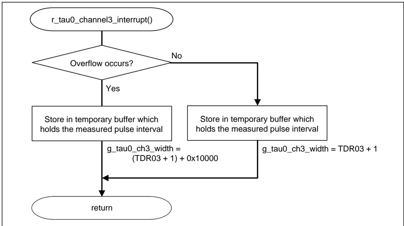
Figure 4.12 INTTM03 Interrupt Processing
