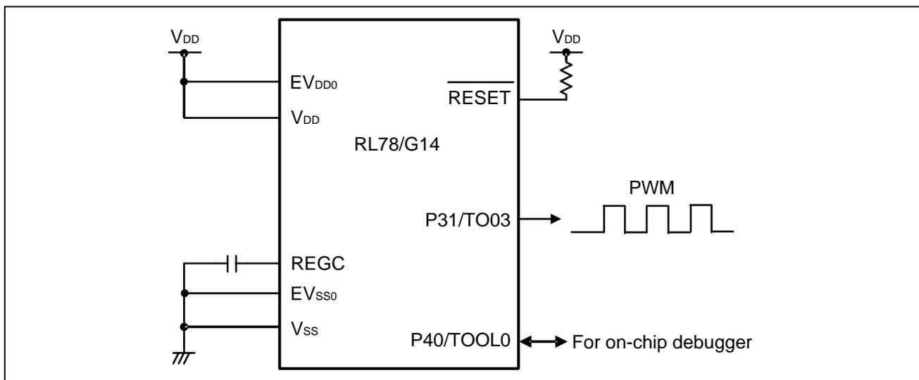
**Figure 5.2 Hardware Configuration**
