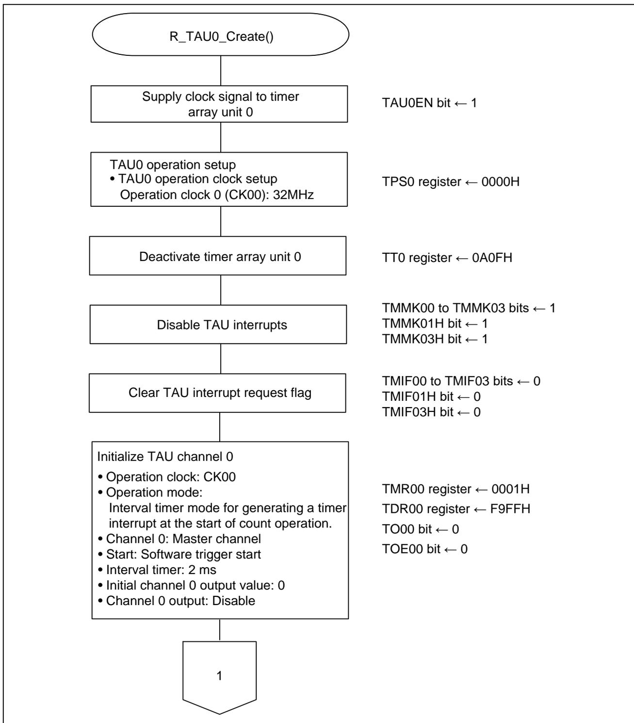
Figure 5.9 Timer Array Unit Setup (1/2)
