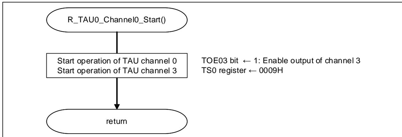
Figure 5.12 Timer Array Unit Startup
