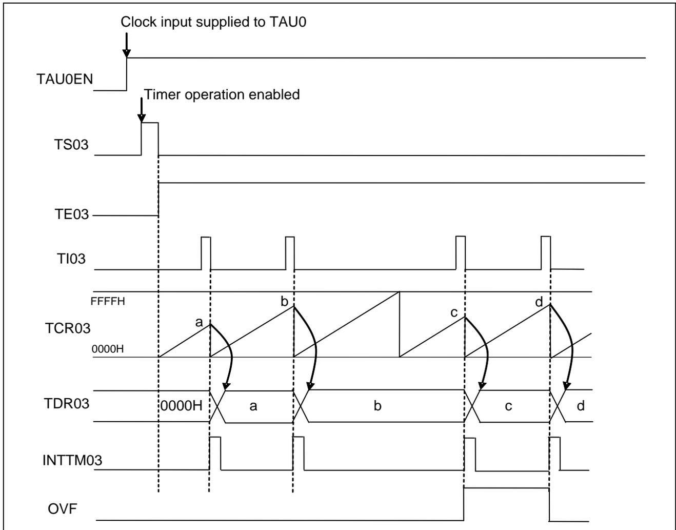
Figure 4.3 Overview of Timer Operation and Interrupts
