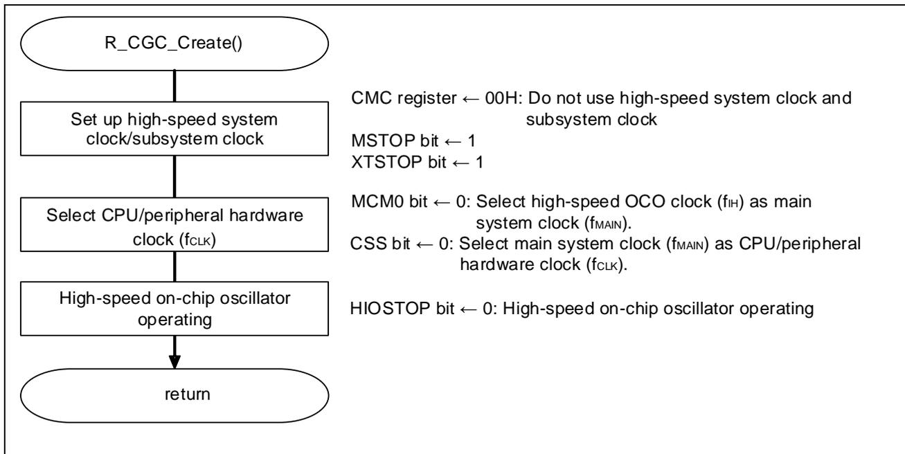
Figure 4.7 CPU Clock Setup
