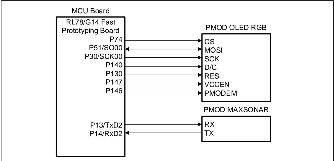
Figure 3.3 Connection of RL78/G14 FPB, PMOD OLED RGB and the Digilent PMOD MAXSONAR
