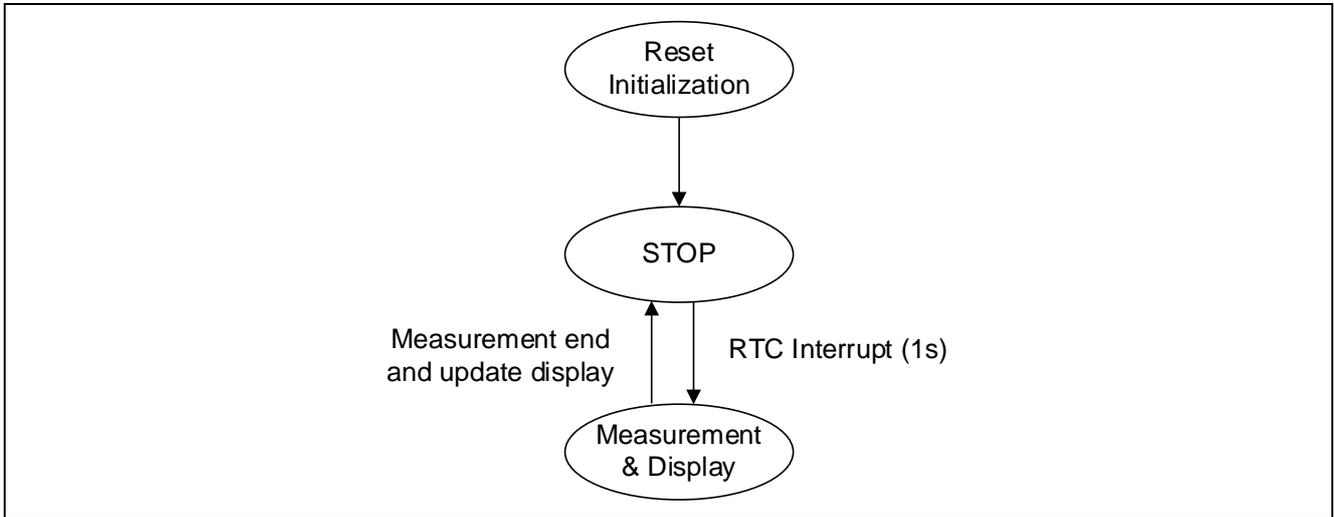
Figure 5.1 Tasks Transition Block Diagram
