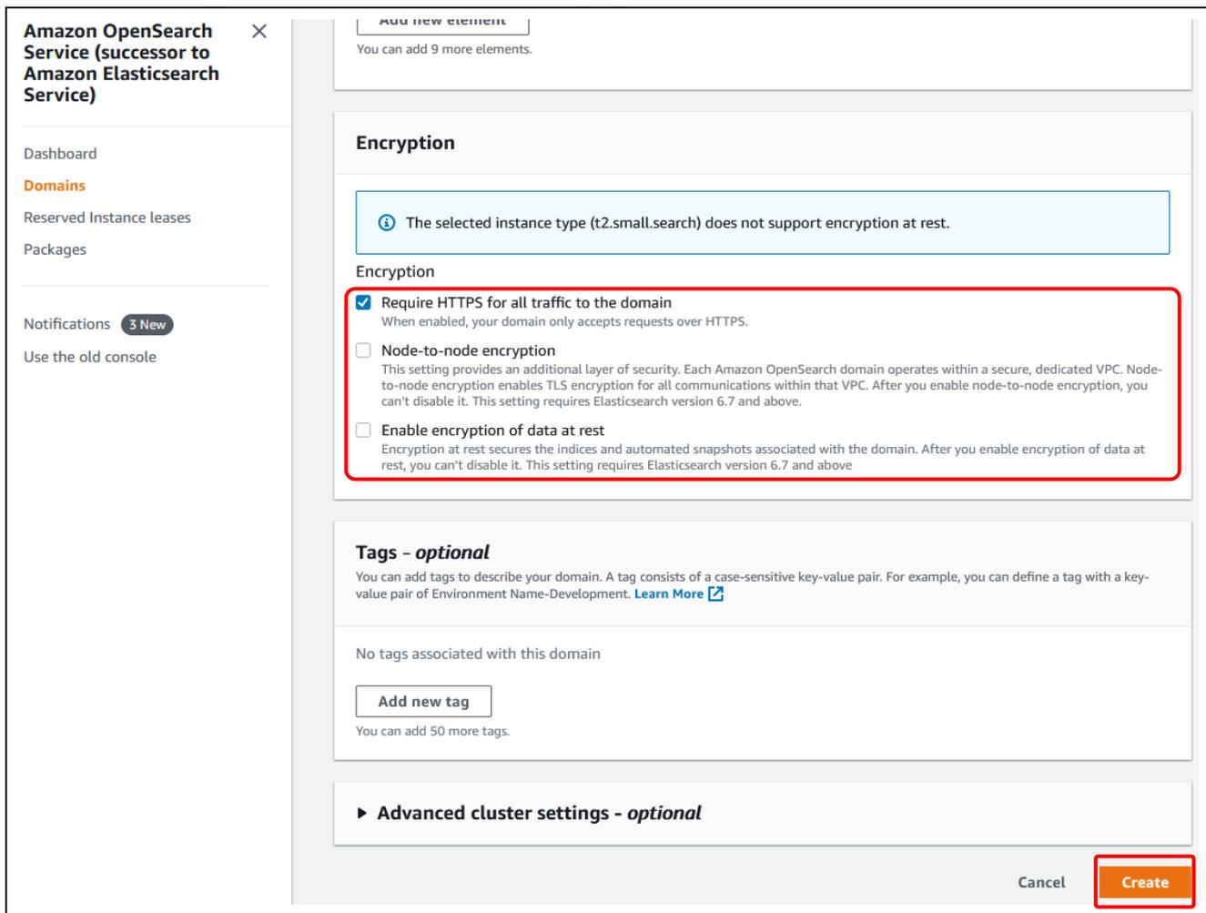
Figure 6.7 Configure encryption then create
