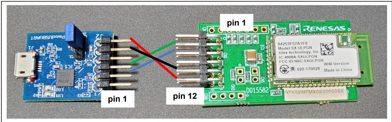
Figure 4.5 Connections between DIGILENT Pmod USBUART and SX-ULPGN
