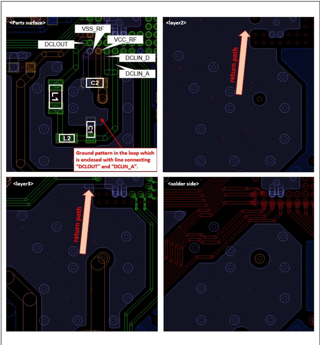
Figure 3-8 Example of the PCB pattern for DC-DC converter mode
