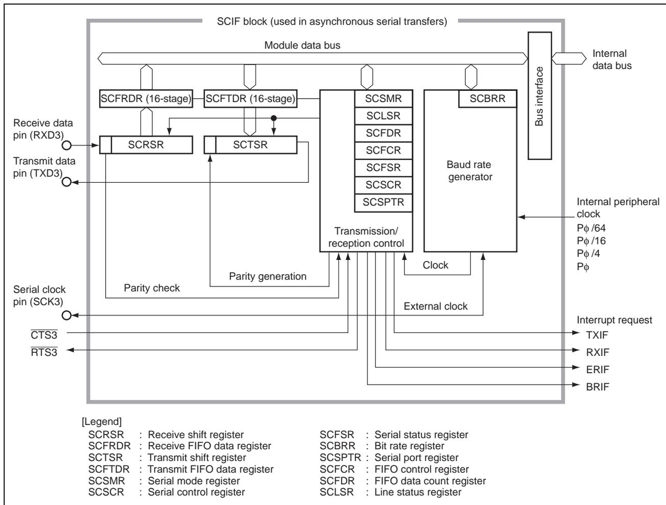
**Figure 2 Block Diagram of SCIF (Serial Communication Interface with FIFO)**
