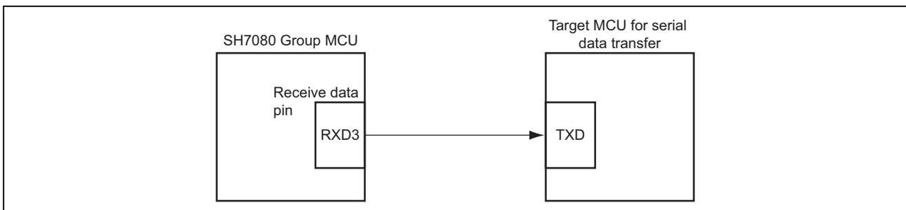
**Figure 1 Asynchronous Serial Data Reception with FIFO**
