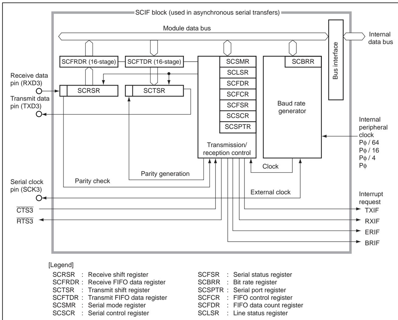
**Figure 2 Block Diagram of SCIF (Serial Communication Interface with FIFO)**
