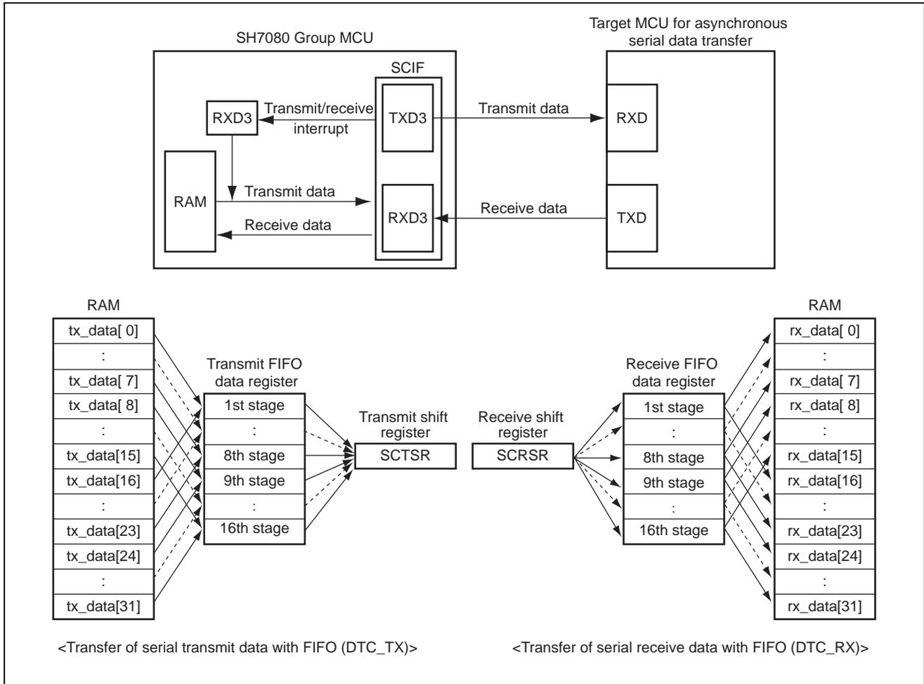
**Figure 1 Asynchronous Serial Data Transmission/Reception Using FIFO and the DTC**
