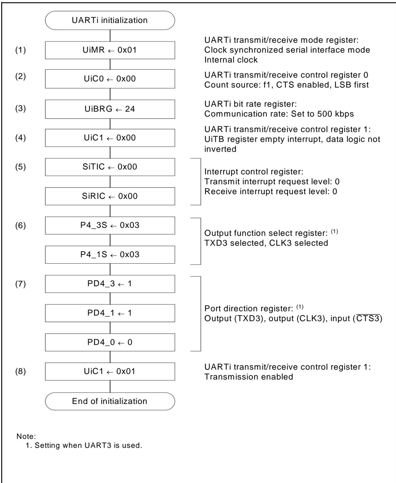
Figure 3.4 UARTi Initialization Process Flowchart (i = 0 to 6)
