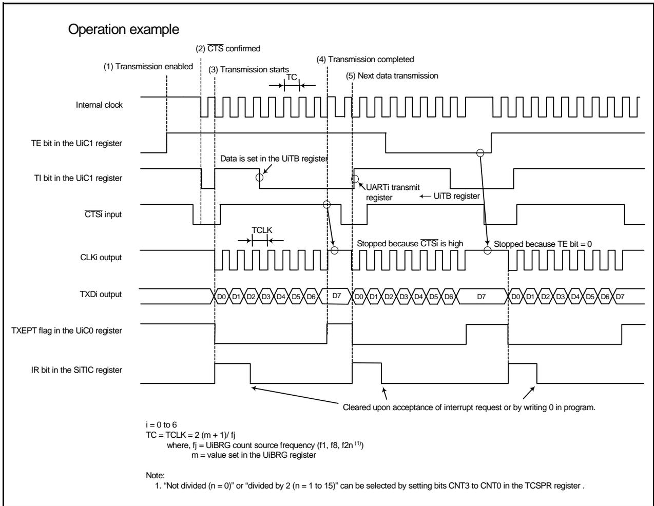
Figure 3.2 Transmit Operation Timing
