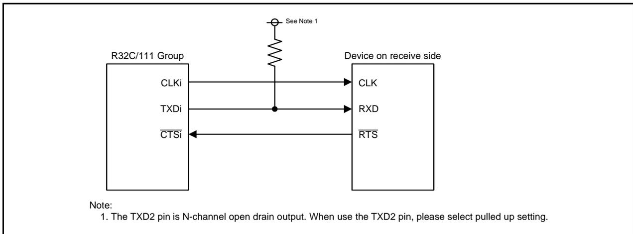
Figure 3.1 Connection Example for Transmission
