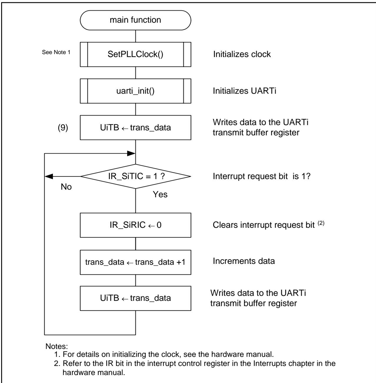
Figure 3.3 main Processing Flowchart (i = 0 to 6)
