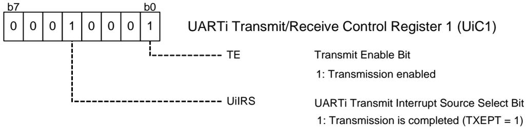
Read the interrupt request bit and set the interrupt control register.
