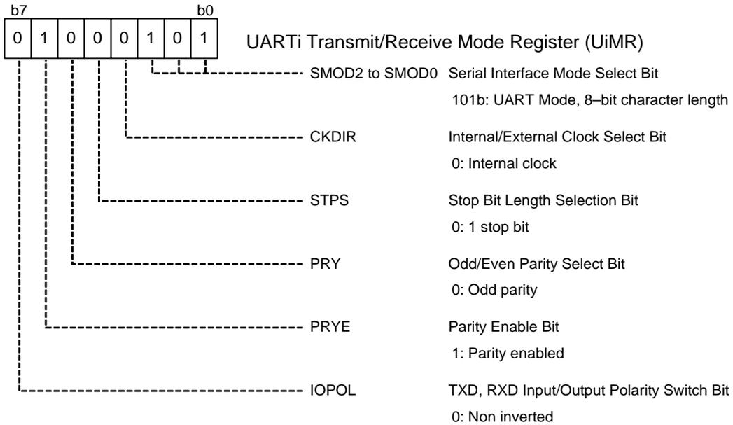
Set the UART<sub>i</sub> transmit/receive control register 0.
