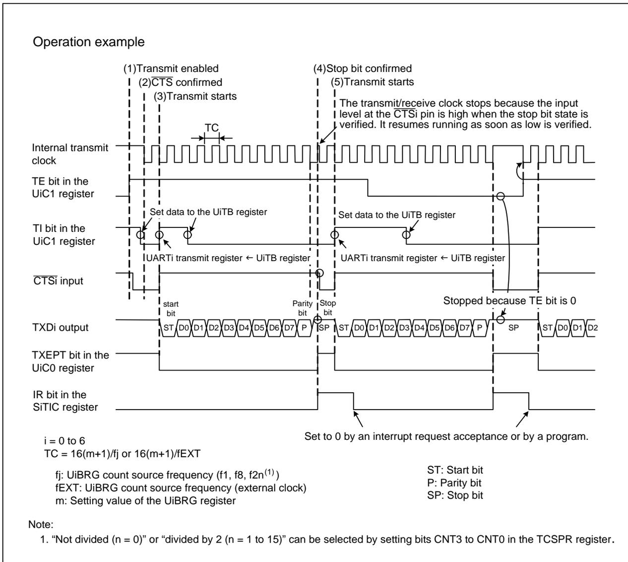
Figure 3.2 Transmit Operation Timing
