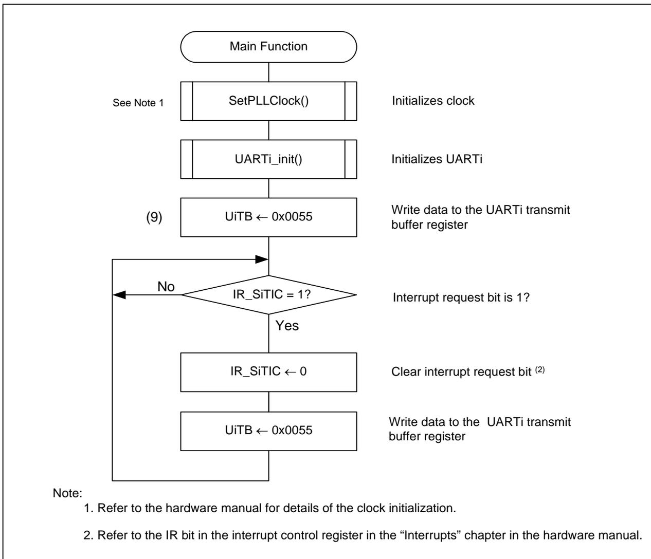
Figure 3.3 main Processing Transmission Flowchart (i = 0 to 6)
