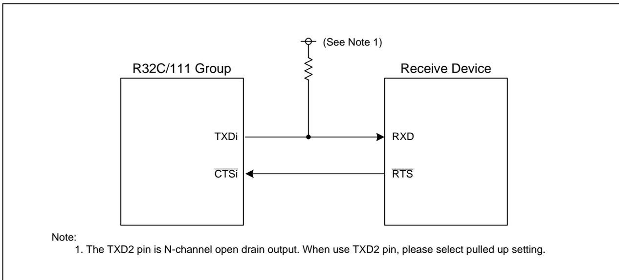
Figure 3.1 Connection Example for Transmission
