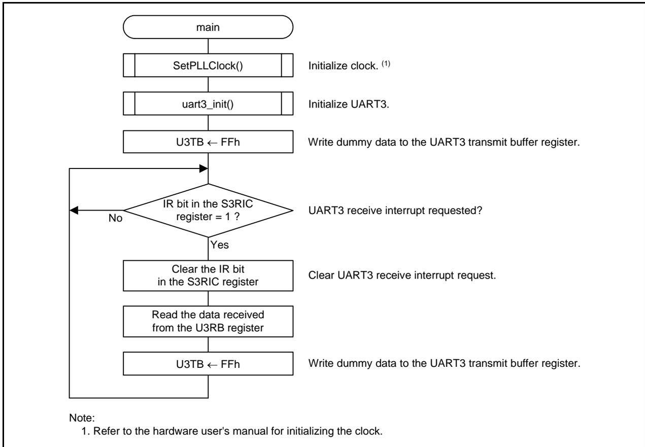
**Figure 3.3 Main Function Flowchart**
