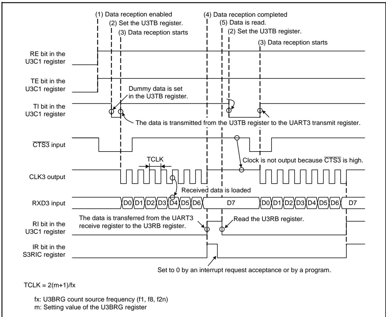
Figure 3.2 Receive Operation
