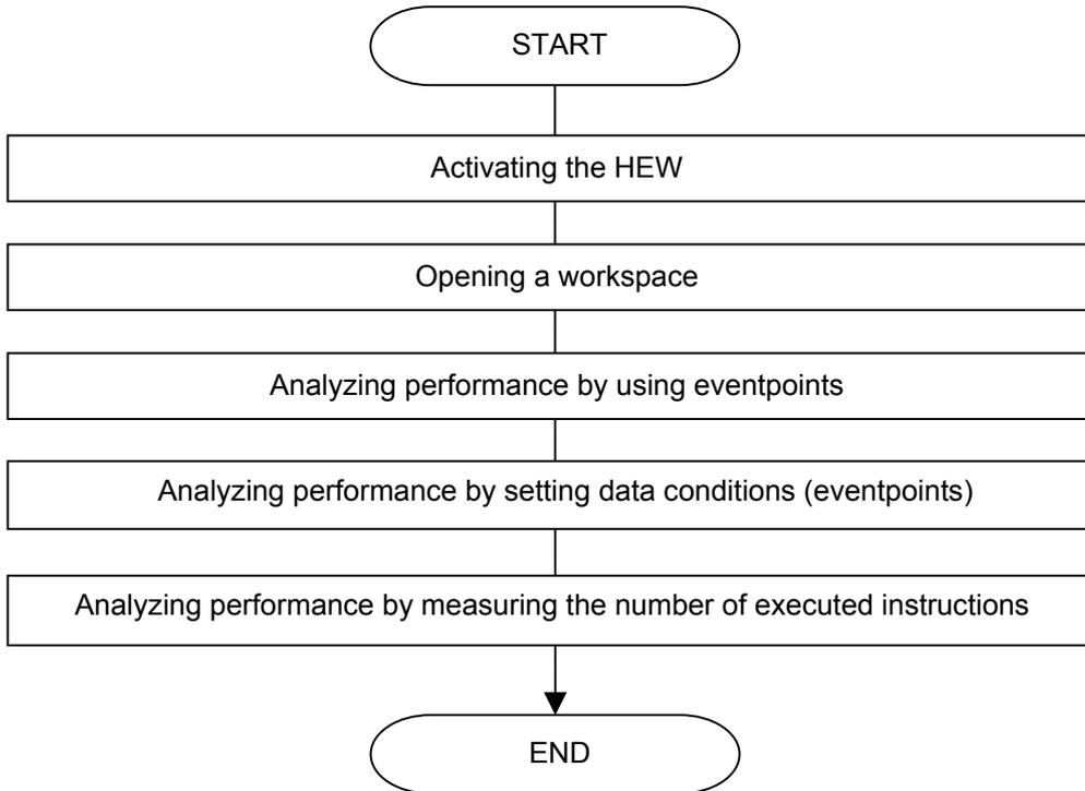
Figure 4.1 Procedures for Sample Program Execution
