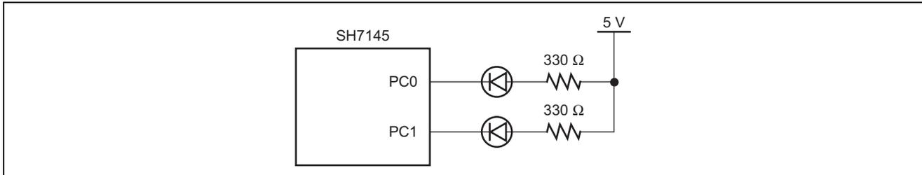
**Figure 1 Connections between SH7145F and LEDs**
