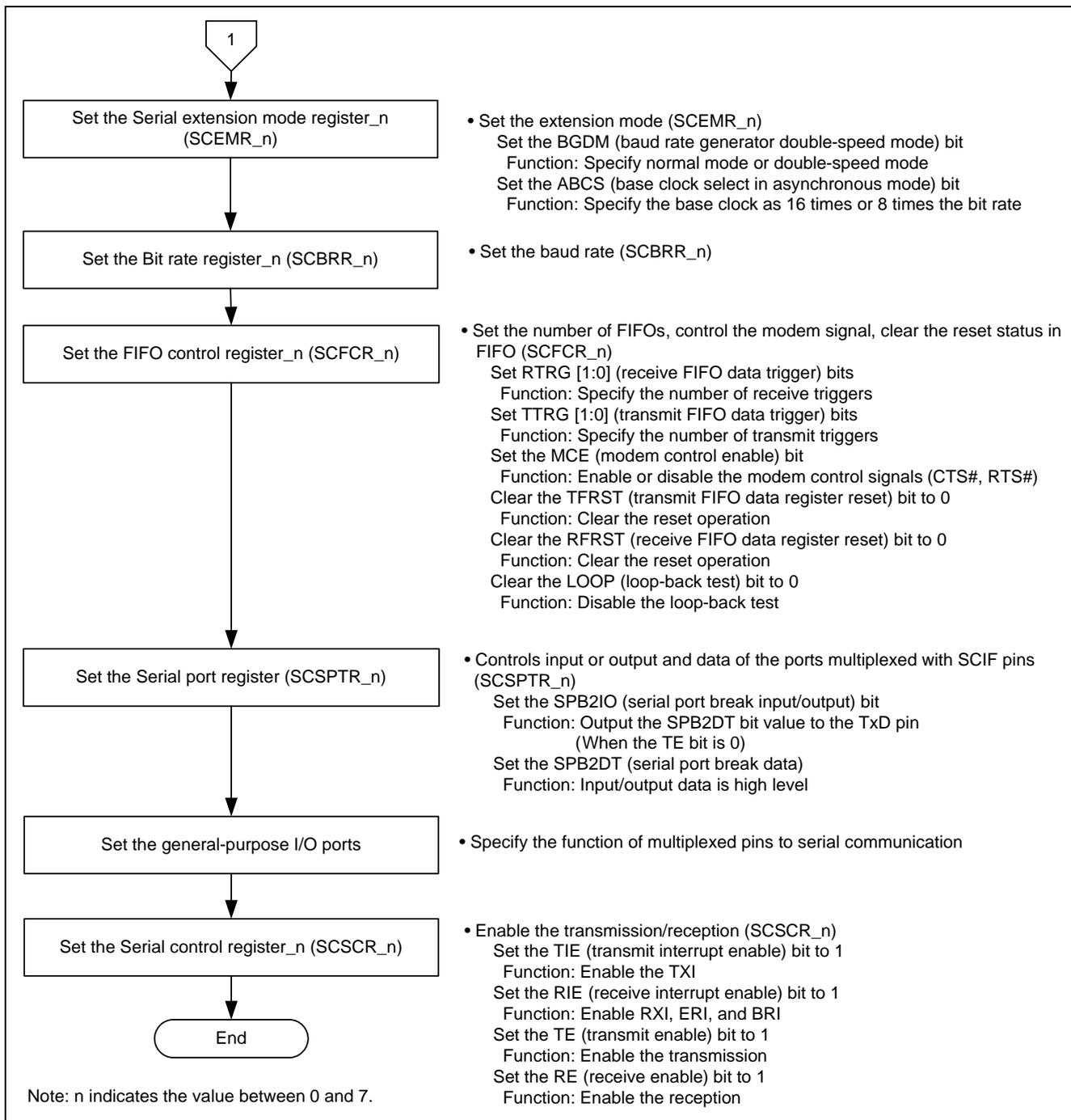
Figure 4 Flow Chart for Configuring the Transmission in Asynchronous Mode (2/2)
