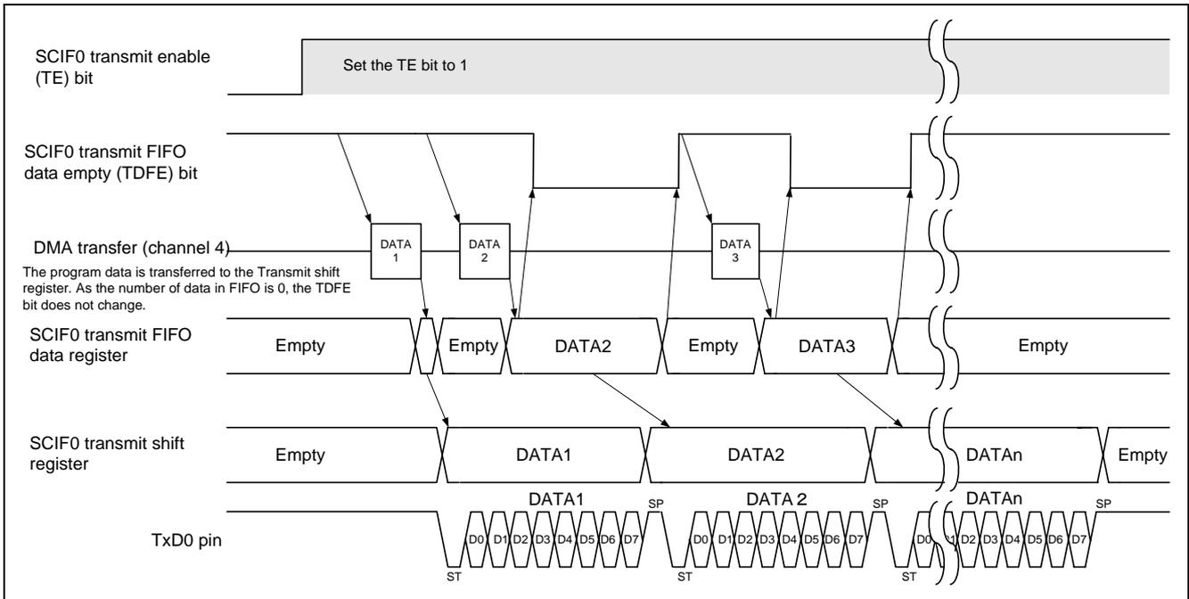
Figure 6 Transmission Timing in the Sample Program
