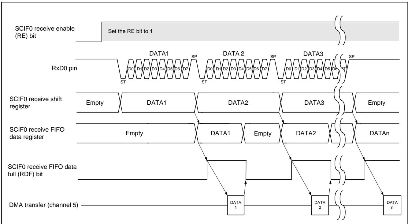
Figure 7 Reception Timing in the Sample Program
