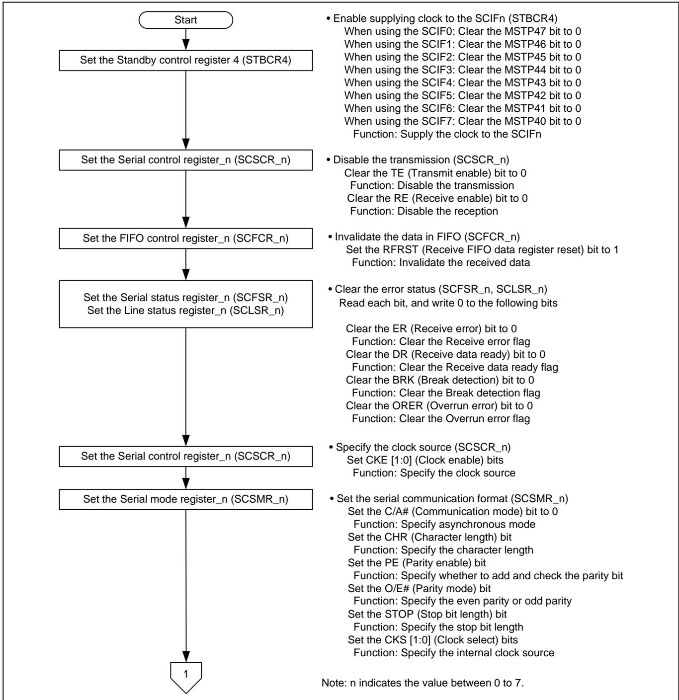
Figure 2 Flow Chart for Configuring the Reception in Asynchronous Mode (1/2)
