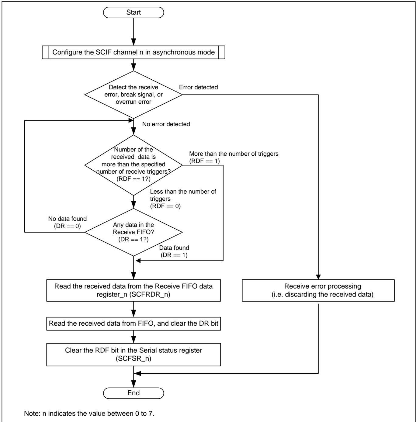
Figure 4 Flow Chart of the Reception in Asynchronous Mode
