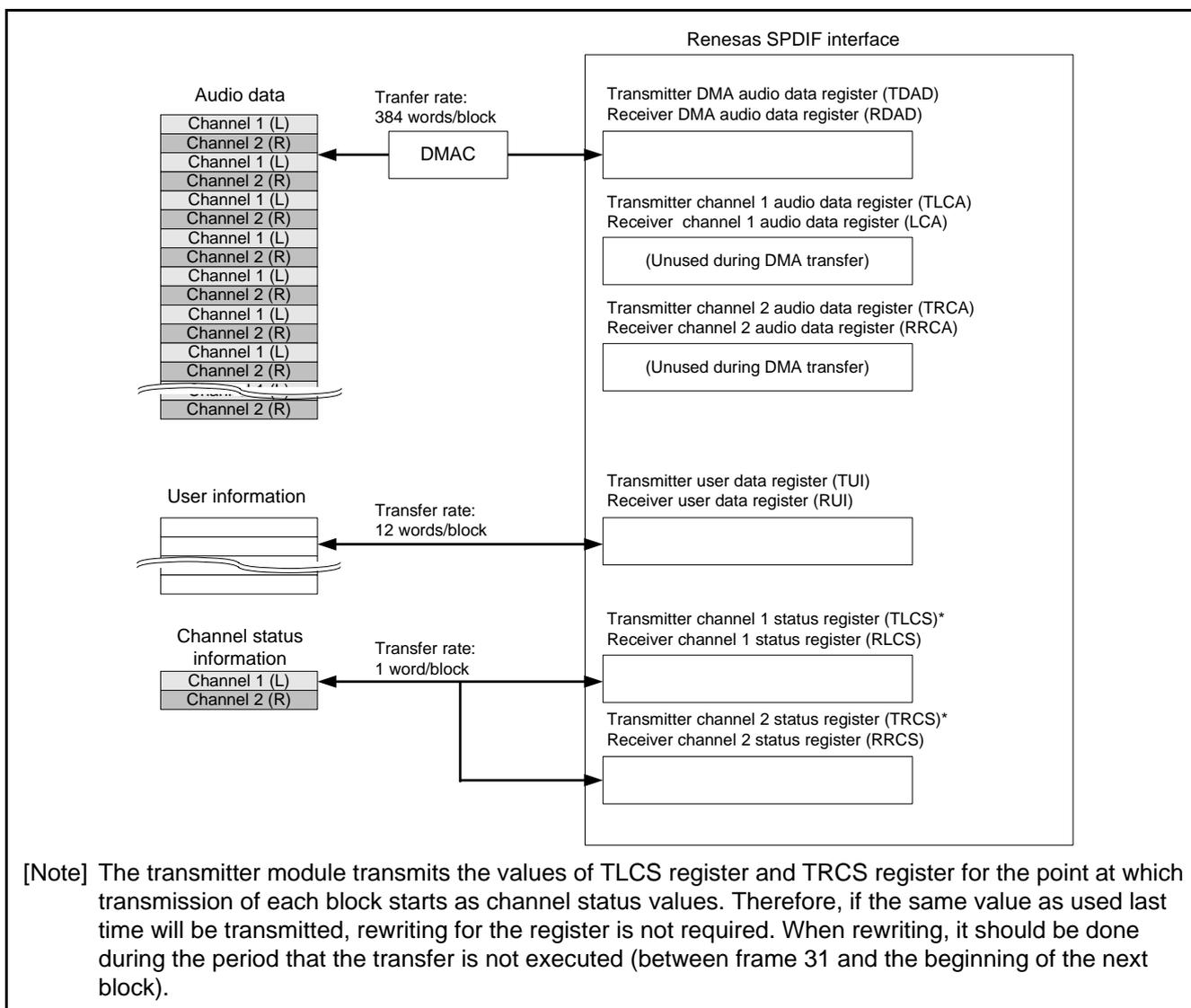
Figure 4.1 Register Group for Reading/Writing Transfer Data
