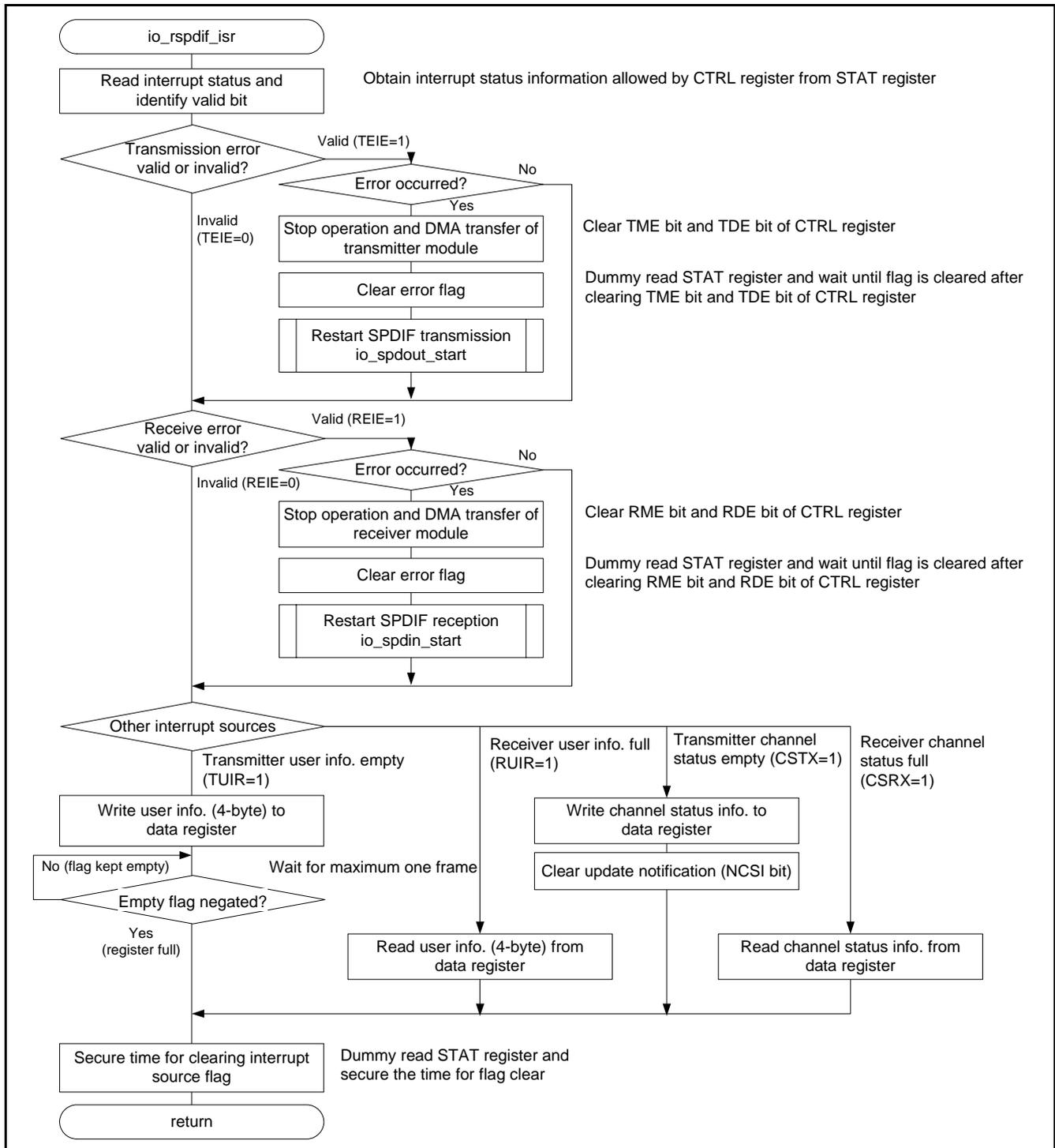
Figure 6.10 Interrupt Function of RSPDIF
