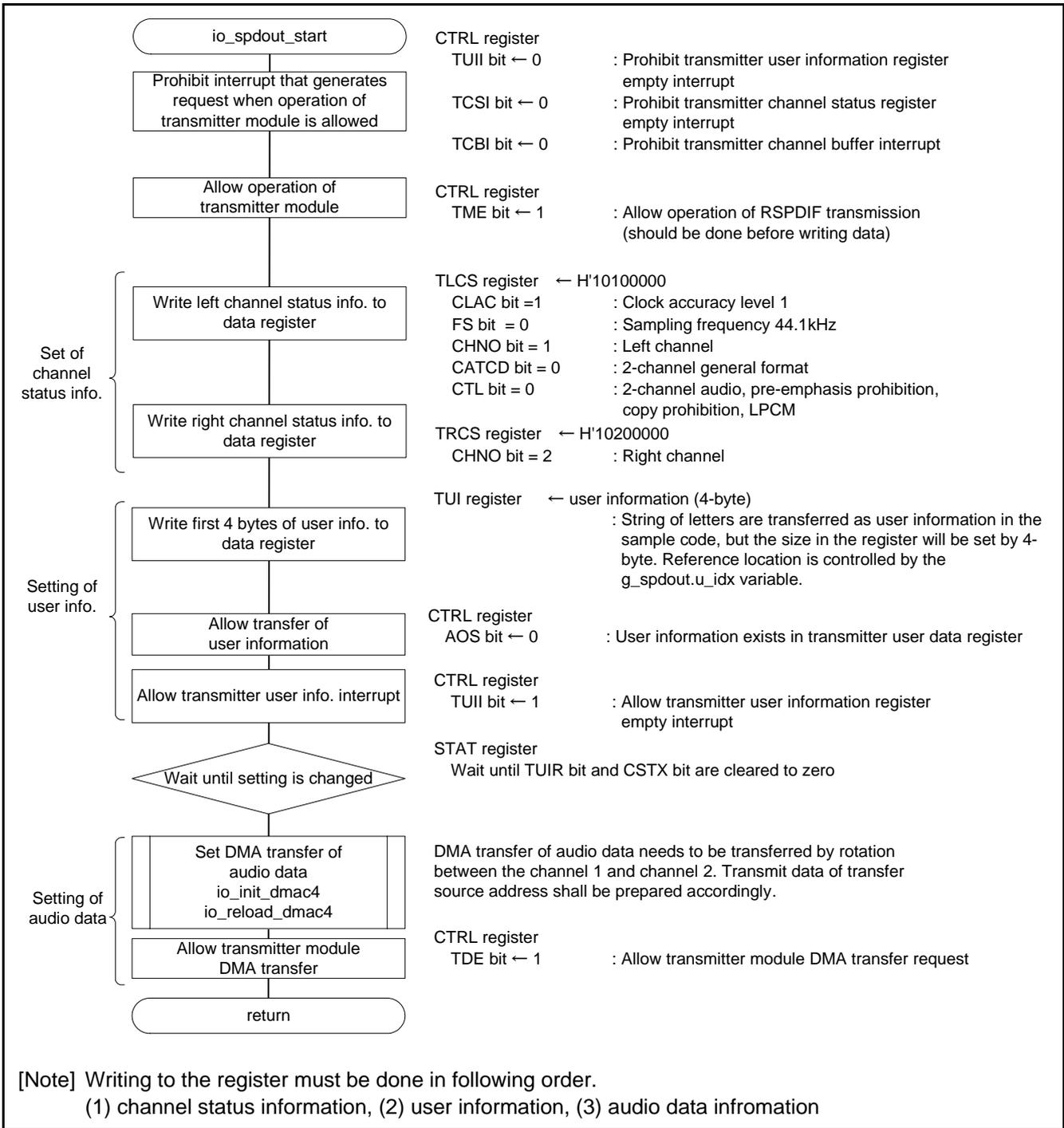
Figure 6.5 Starting of RSPDIF Transmission
